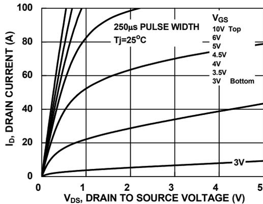
Figure 9. Saturation Characteristics
