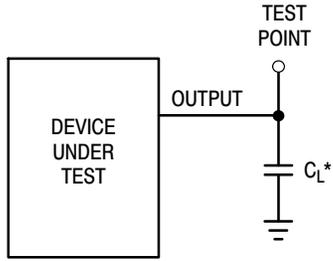
\*Includes all probe and jig capacitance
