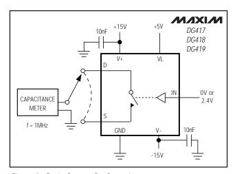
Figure 9. Drain-Source On-Capacitance
