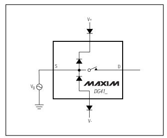
Figure 1. Overvoltage Protection Using External Blocking Diodes
