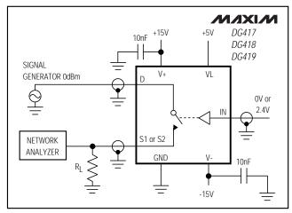
Figure 6. Off-Isolation Rejection Ratio
