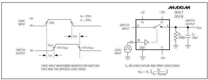
Figure 2. DG417/DG418 Switching Time
