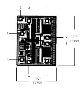
TRANSISTOR COUNT: 32 SUBSTRATE CONNECTED TO V+
