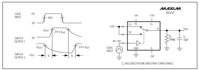
Figure 4. DG419 Break-Before-Make Interval
