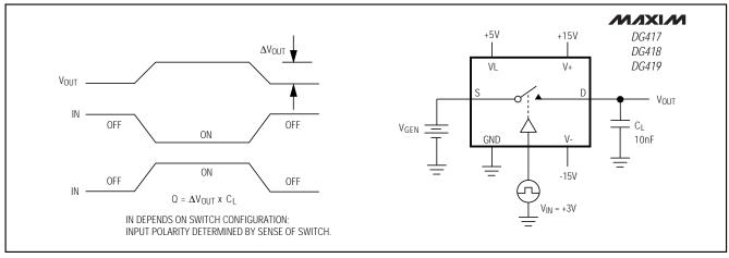
Figure 5. Charge Injection
