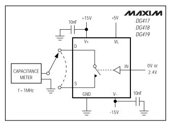
Figure 8. Drain-Source Off-Capacitance
