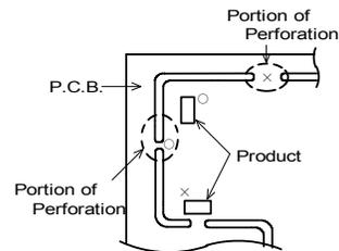
Products shall not be arranged on the line of a series of holes when there are big holes in P.C.B.
