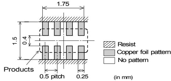
**16.7 Standard Soldering Condition (Reflow soldering)**
