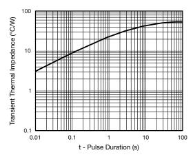
Fig. 7 - Typical Transient Thermal Impedance
