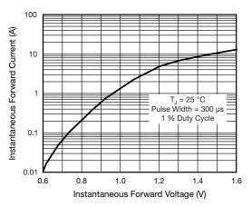
Fig. 4 - Typical Instantaneous Forward Characteristics
