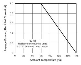
Fig. 1 - Forward Current Derating Curve
