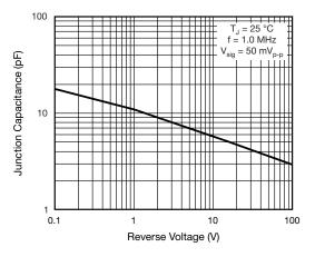
Fig. 6 - Typical Junction Capacitance
