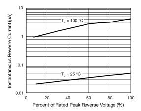
Fig. 5 - Typical Reverse Characteristics
