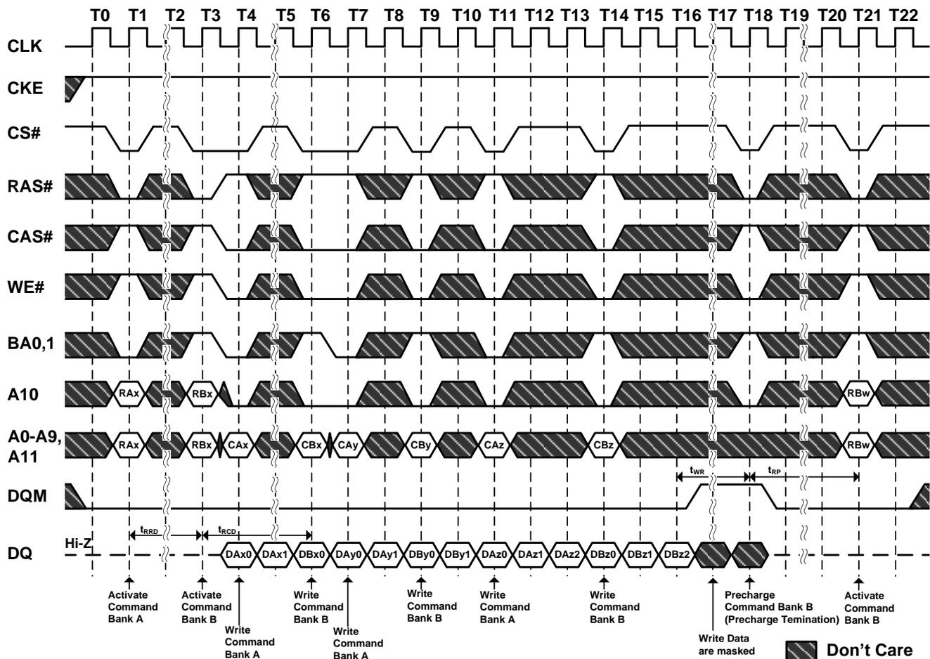
**Figure 42. Precharge Termination of a Burst**
