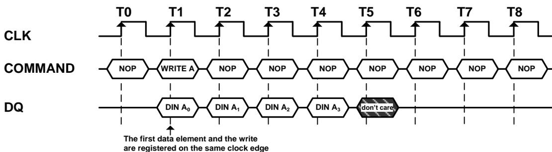
**Figure 10. Burst Write Operation (Burst Length = 4)**
