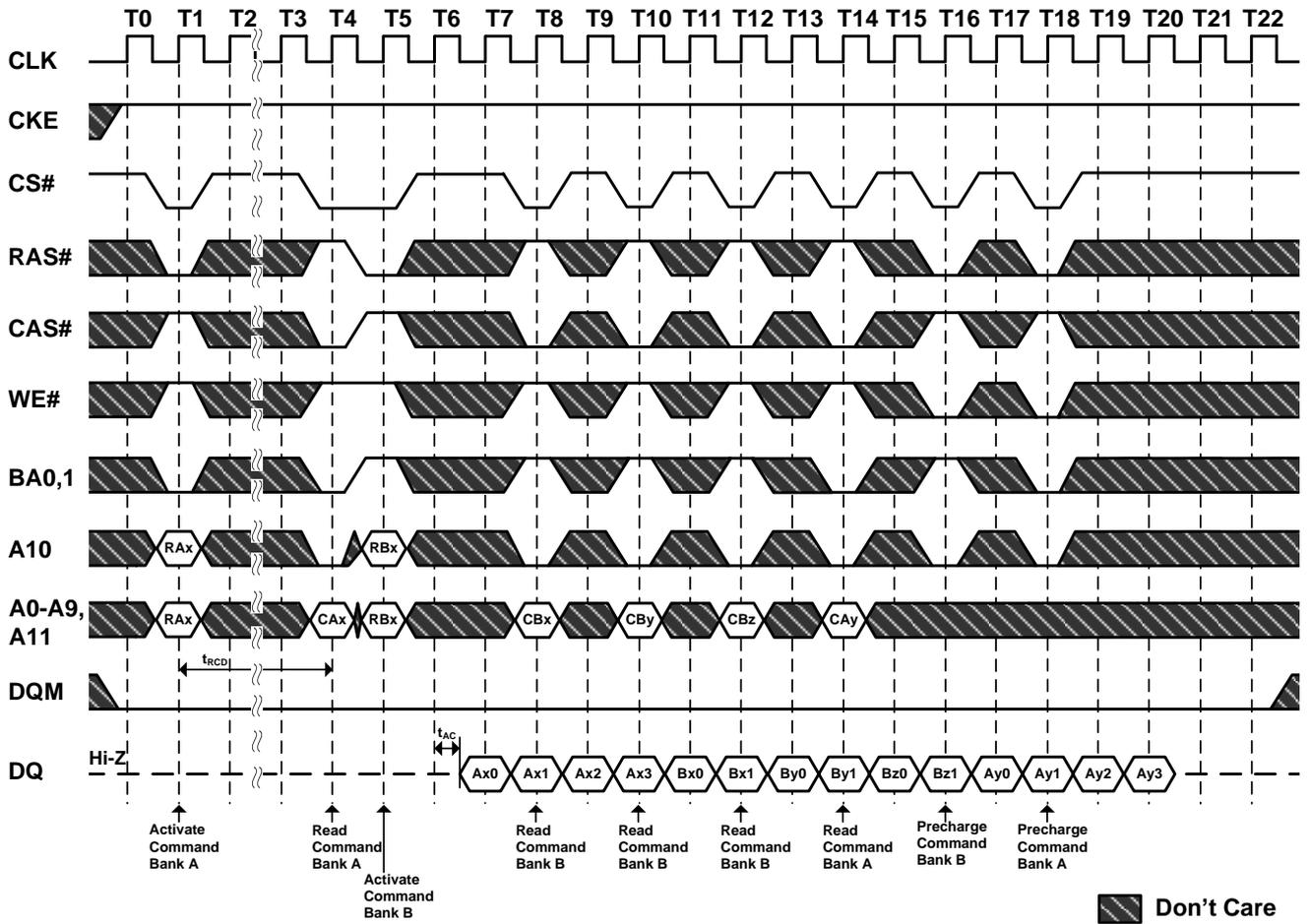
Figure 33. Interleaved Column Write Cycle (Burst Length=4)
