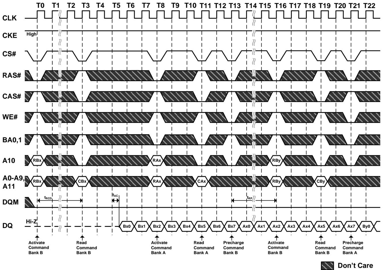
Figure 30. Random Row Write (Interleaving Banks)
