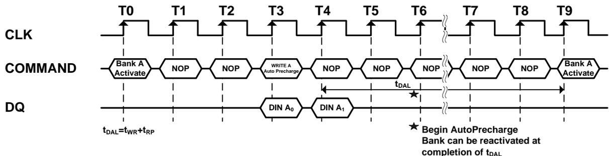
**Figure 14. Burst Write with Auto-Precharge (Burst Length = 2)**
