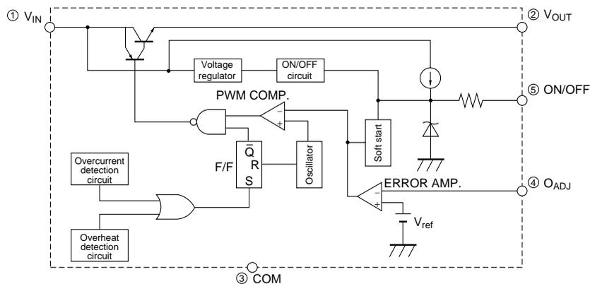
Fig.15 Step Down Type Circuit Diagram
