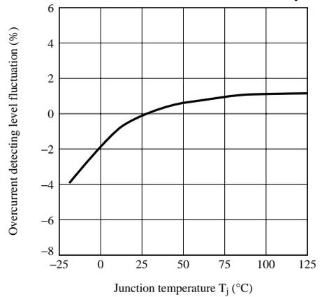
**Fig.12 Threshold Voltage vs. Junction Temperature**
