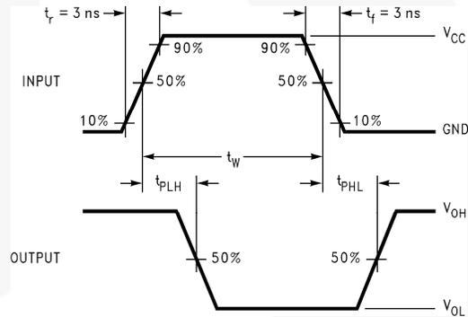
**Figure 5. AC Waveforms**
