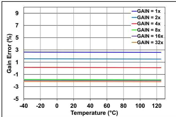
**FIGURE 2-33:** Gain Error vs. Temperature vs. Gain.
