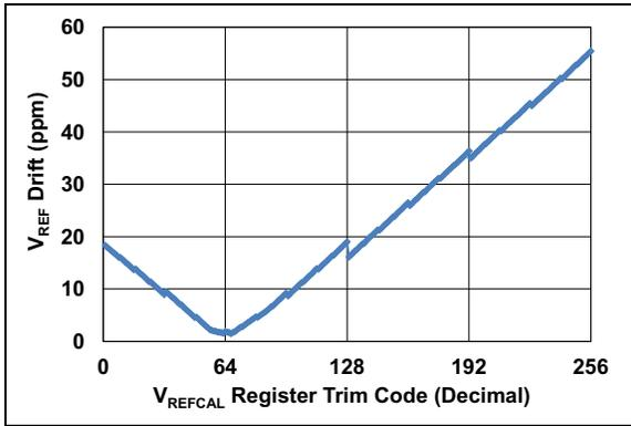
**FIGURE 5-7:** *V<sub>REF</sub> Tempco vs. V<sub>REFCAL</sub> Trim Code Chart.*
