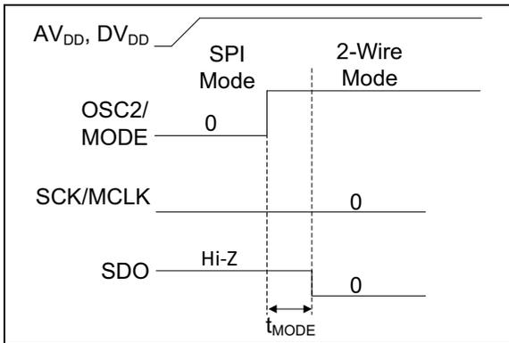
**FIGURE 1-5:** Entering 2-Wire Interface Mode Timing Diagram.
