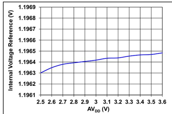
**FIGURE 2-35:** Internal Voltage Reference vs. Supply Voltage.
