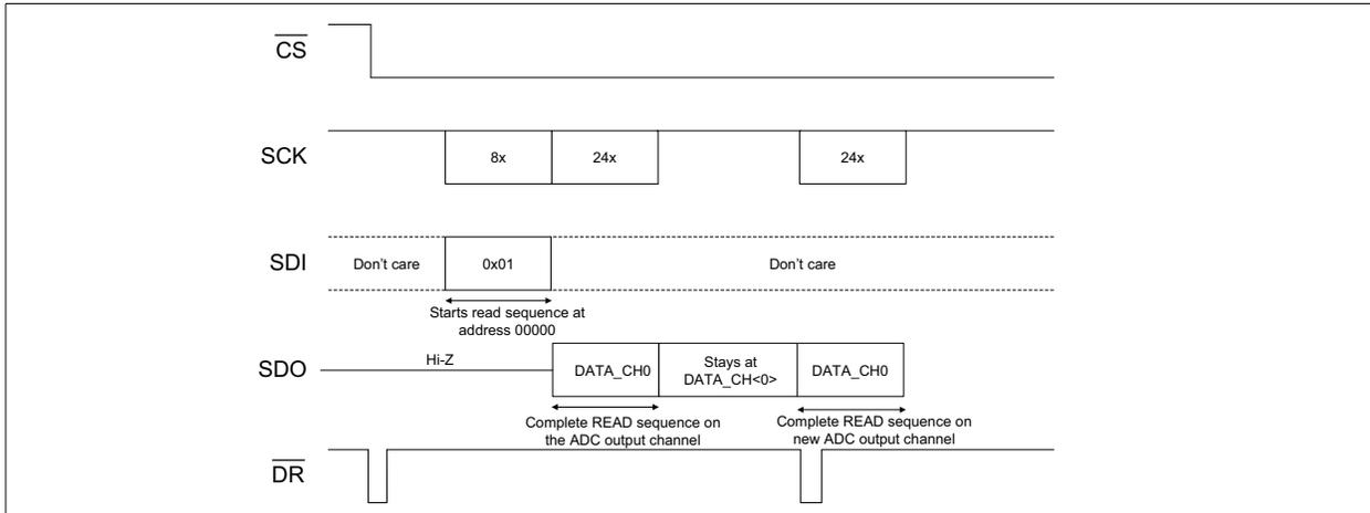
**FIGURE 6-7:** Typical Continuous Read Communication (WIDTH\_DATA<1:0> = 01, SPI Mode 0,0).
