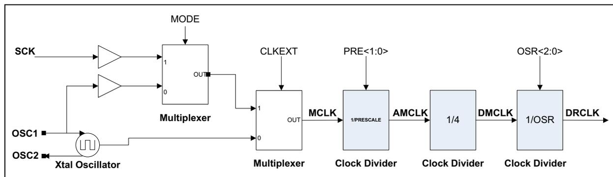
**FIGURE 4-1:** Clock Sub-Circuitry.
