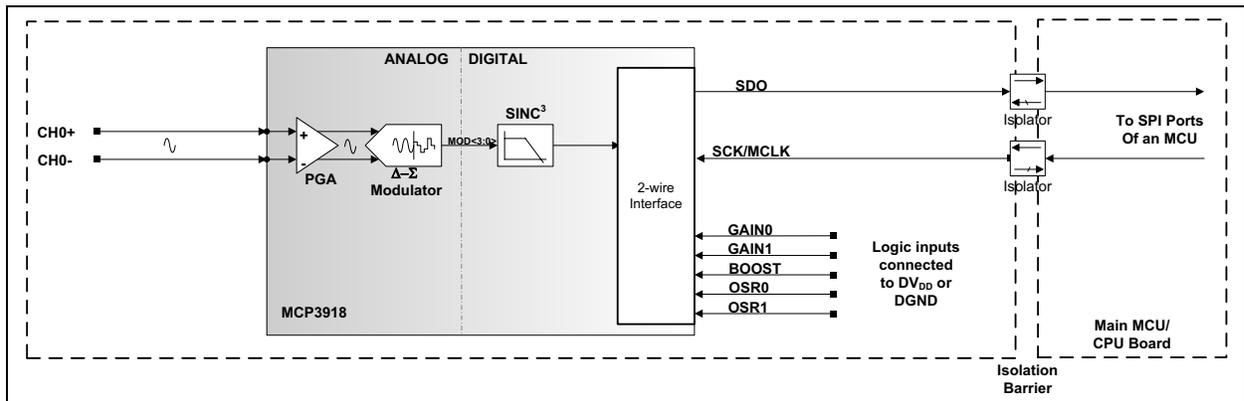
**FIGURE 7-1:** MCP3918 2-Wire Interface Typical Application Schematic.
