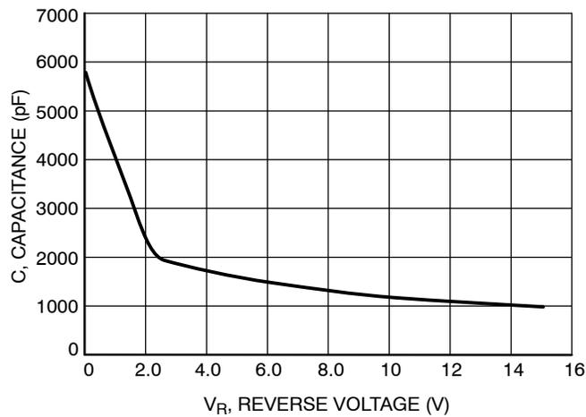
Figure 7. Typical Capacitance
