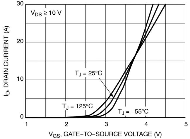
Figure 2. Transfer Characteristics
