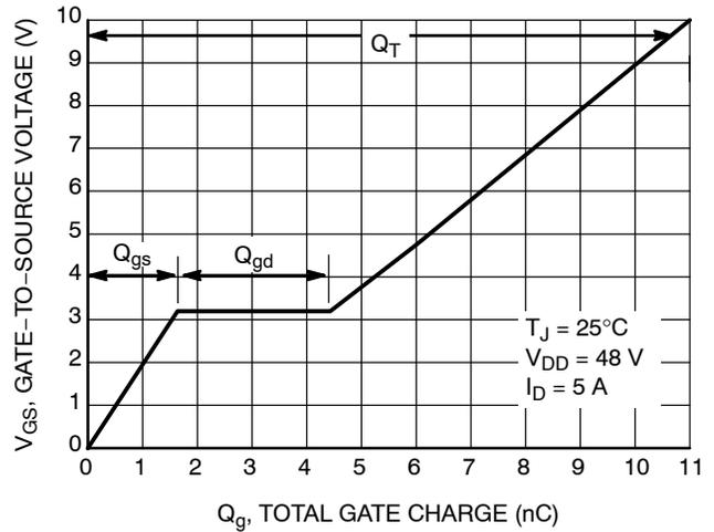
Figure 8. Gate-to-Source vs. Gate Charge
