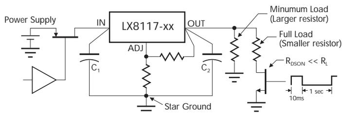
FIGURE 1 — DYNAMIC INPUT and OUTPUT TEST
