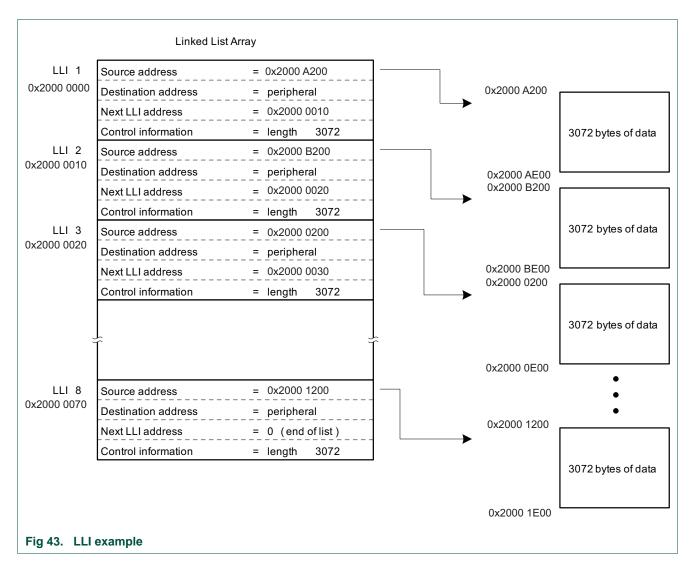
The first LLI, stored at 0x2000 0000, defines the first block of data to be transferred, which is the data stored from address 0x2000 A200 to 0x2000 AE00:
