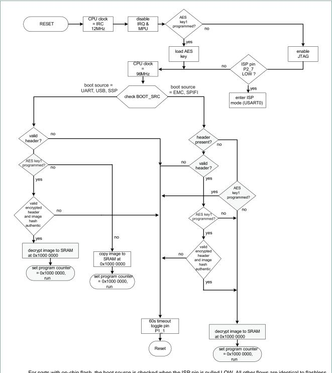
For parts with on-chip flash, the boot source is checked when the ISP pin is pulled LOW. All other flows are identical to flashless parts. See Figure 11.
