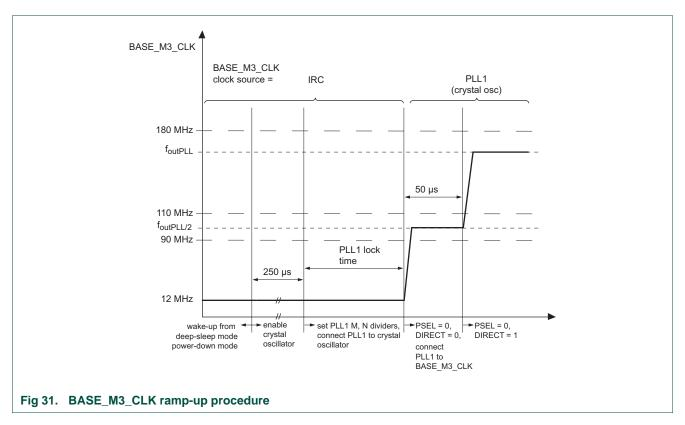
A similar two-step procedure applies when changing the BASE\_M3\_CLK from low to high frequencies using the PLL0AUDIO as the clock source.
