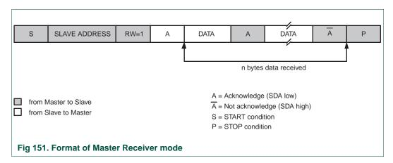
After a Repeated START condition, I<sup>2</sup>C may switch to the master transmitter mode.
