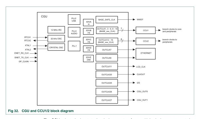
The CGU selects the inputs to the clock generators from multiple clock sources, controls the clock generation, and routes the outputs of the clock generators through the clock source bus to the output stages. Each output stage provides an independent clock source and corresponds to one of the base clocks for the LPC18xx. See <a href="Table 107">Table 107</a> for a description of each base clock and <a href="Table 109">Table 109</a> for the possible clock sources for each base clock.
