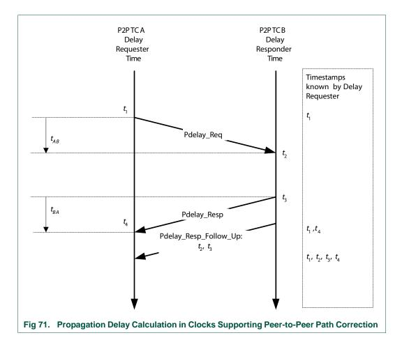
As shown in Figure 71, the propagation delay is calculated in the following way:
