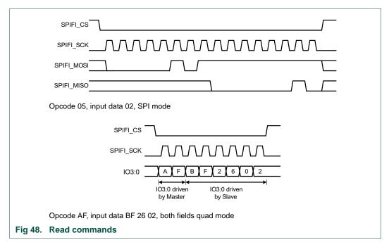
In quad mode, the IO3:0 lines are driven by the SPIFI in opcode, address, intermediate and output data fields, and driven by the flash memory in input data fields. In address fields the more significant bytes are sent first.
