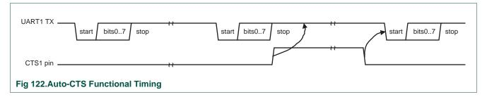
While starting transmission of the initial character the CTS1 signal is asserted. Transmission will stall as soon as the pending transmission has completed. The UART will continue transmitting a 1 bit as long as CTS1 is de-asserted (high). As soon as CTS1 gets de-asserted transmission resumes and a start bit is sent followed by the data bits of the next character.
