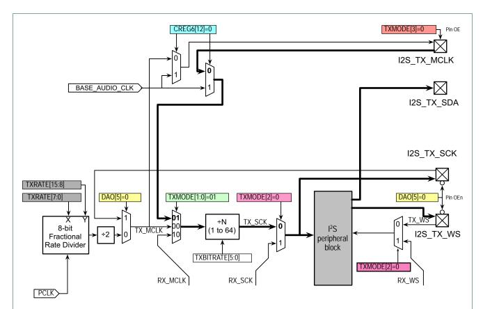
Bold lines indicate the clock path for this configuration. CREG6 bits 12 and 13 select BASE\_AUDIO\_CLK for the I2S0 interface. CREG bits 14 and 15 select BASE\_AUDIO\_CLK for the I2S1 interface.
