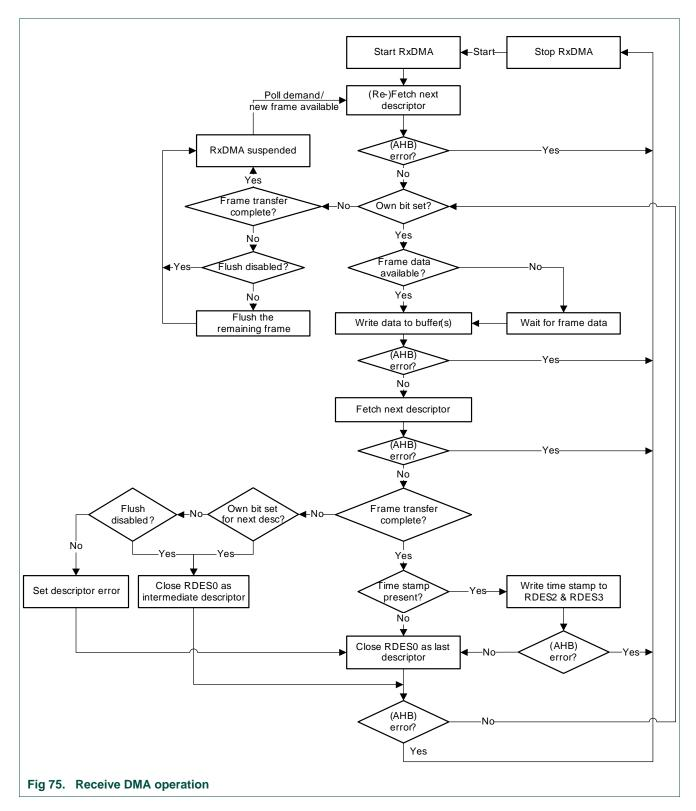
The DMA does not acknowledge accepting the status from the MTL until it has completed the time stamp write-back and is ready to perform status write-back to the descriptor.
