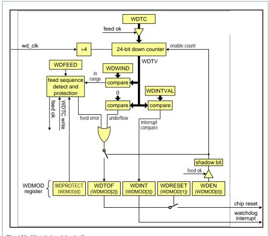
Fig 109. Watchdog block diagram
