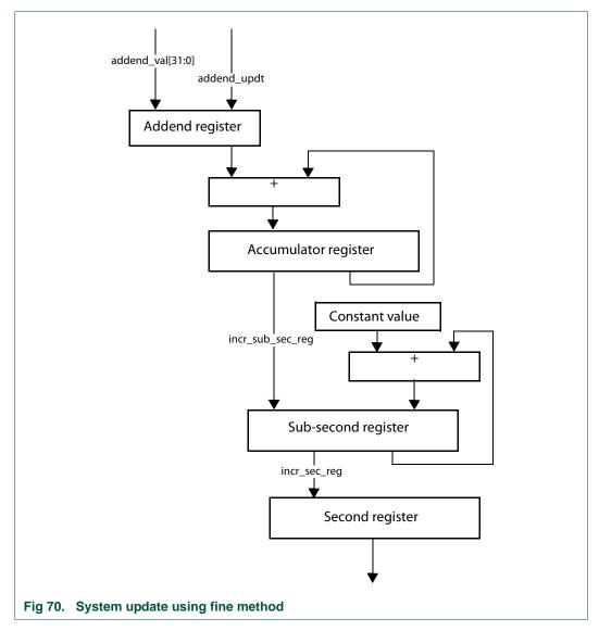
The System Time Update logic requires a 50-MHz clock frequency to achieve 20-ns accuracy. The frequency division is the ratio of the reference clock frequency to the required clock frequency. Hence, if the reference clock is, for example, 66 MHz, this ratio is calculated as  $66 \, \text{MHz} / 50 \, \text{MHz} = 1.32$ . Hence, the default addend value to be set in the register is  $2^{32} / 1.32$ ,  $0 \times 10^{12} \, \text{C} = 1.32$ .
