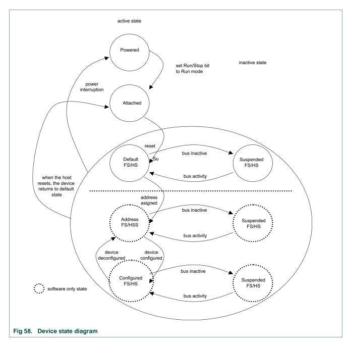
The states powered, attach, default FS/HS, suspend FS/HS are implemented in the device controller and are communicated to the DCD using the following status bits:
