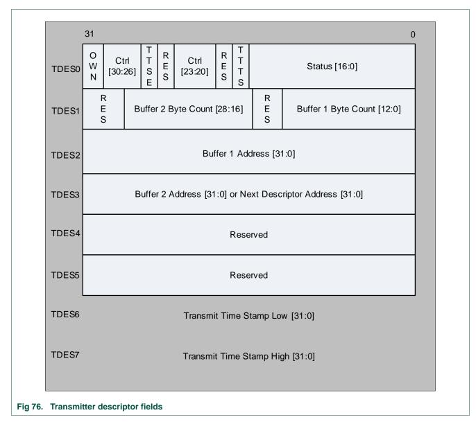
The DMA always reads or fetches four DWORDS of the descriptor from system memory to obtain the buffer and control information as shown in <u>Figure 77</u>. When Advanced timestamp feature support is enabled, TDES0 has additional control bits[6:3] for channel 1 and channel 2. For channel 0, the bits 6:3 are ignored. The bits 6:3 are described in <u>Table 576</u>.
