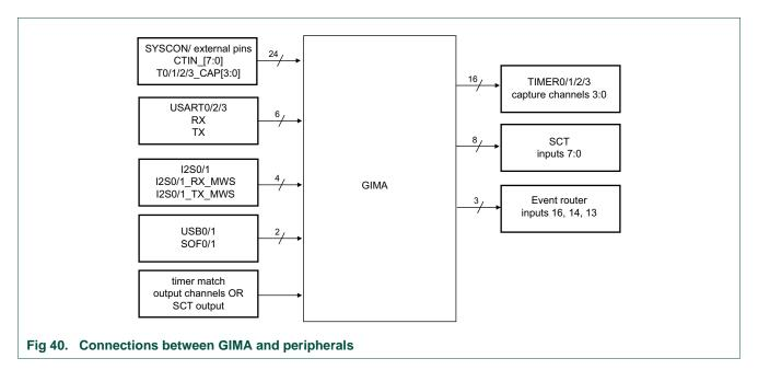
Table 191 shows the GIMA output number, the peripheral function the GIMA output is connected to, and the events that can be selected for this GIMA output. For signals that originate from an external pin, select a pin from the pinout (more than one pins may be possible) and program the corresponding pin function in the pin configuration register. Inputs from external pins include any of the timer capture pins (T0/1/2/3\_CAPx and SCT input pins CTIN\_x).
