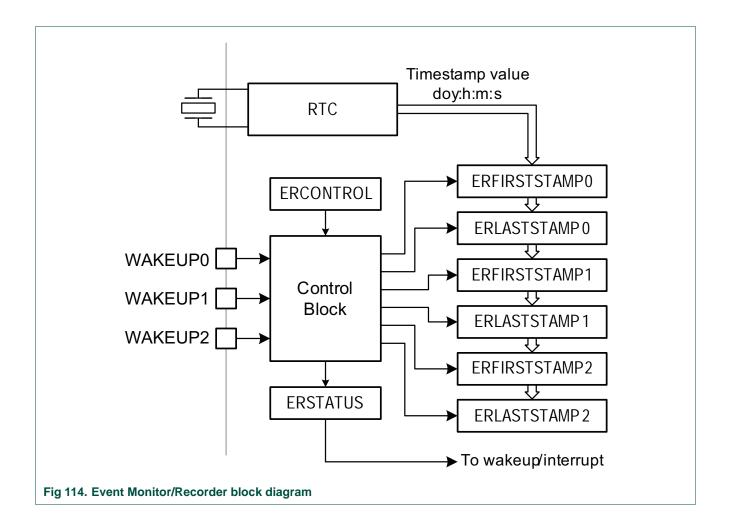
The CPU may at any time check the ERSTATUS register for events. If, for instance the EV0 bit is set, the corresponding ERFIRSTSTAMP0 and ERLASTSTAMP0 registers contain valid timestamps. The ERCOUNTER0 will also contain a valid count of the total number of events on channel 0 (up to a maximum of seven).
