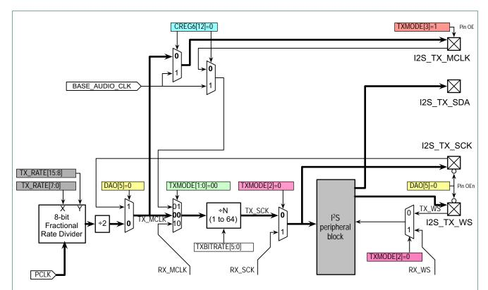
Bold lines indicate the clock path for this configuration. CREG6 bits 12 and 13 select BASE\_AUDIO\_CLK for the I2S0 interface. CREG bits 14 and 15 select BASE\_AUDIO\_CLK for the I2S1 interface.
