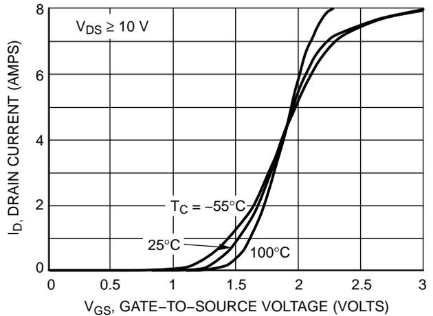
**Figure 2. Transfer Characteristics**
