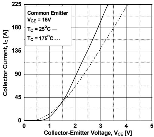
Figure 4. Transfer Characteristics
