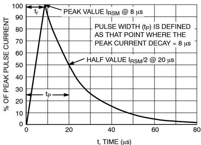
Figure 3. 8 x 20  $\mu s$  Pulse Waveform
