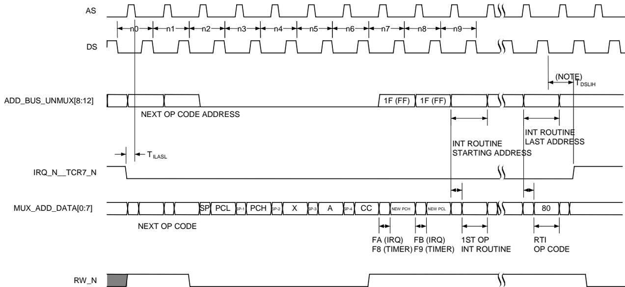
**Note:**  $t_{DSLH}$ - the interrupting device must release the IRQ\_N line within this time to prevent subsequent recognition of the same interrupt.
