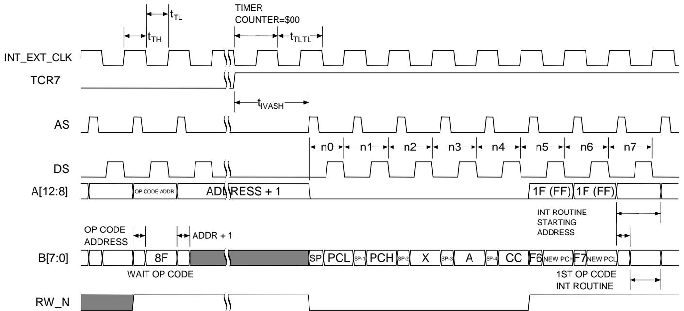
**Figure 17. Timer Interrupt After WAIT Instruction Timing**
