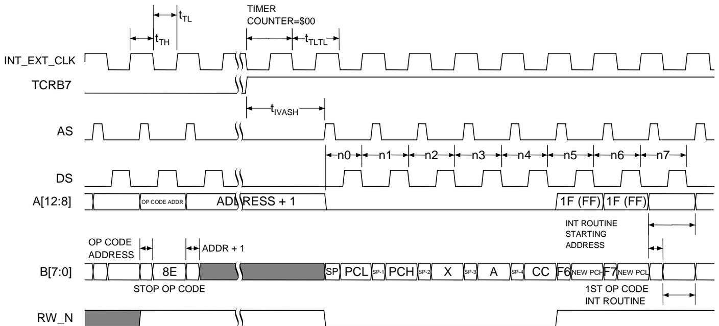
**Figure 18. Interrupt Recovery From STOP Instruction Timing**
