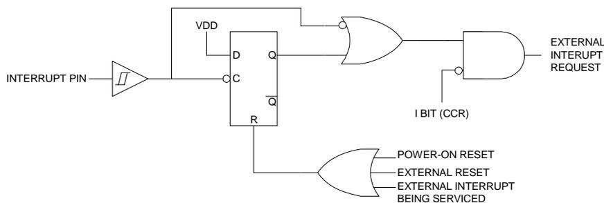
**Figure 9. Interrupt Functional Diagram**
