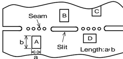
Products (A, B, C, D) shall be located carefully so that products are not subject to the mechanical stress due to warping the board. Because they may be subjected the mechanical stress in order of A>C>B≒D.
