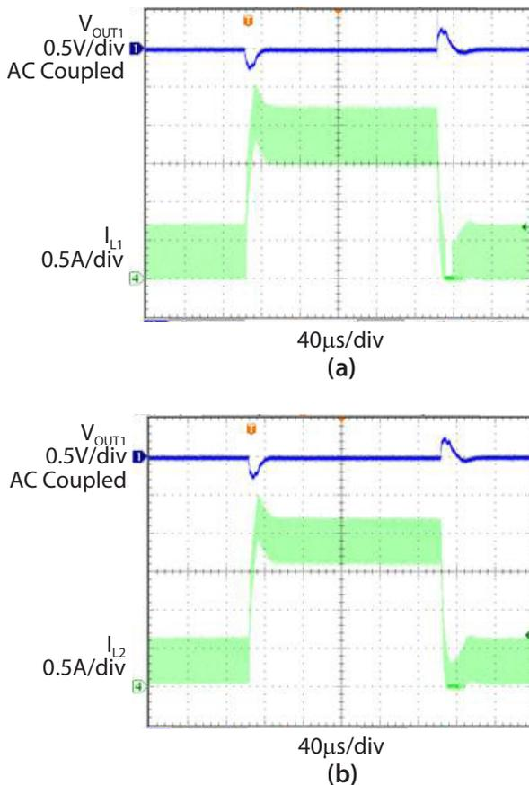
**Figure 12. Load Transient Response of the Converter in Figure 1.**
