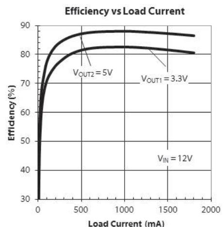
Figure 1. 1.3MHz 12V to 5V and 3.3V Step-down Converter
