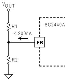
**Figure 4.**  $R_1$  and  $R_2$  Set the Output Voltage
