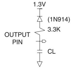
Note:  $C_L = 100$  pF including jig capacitance.
