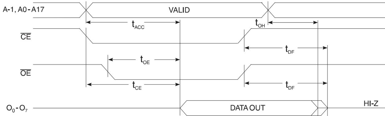
Note:  $\overline{\text{BYTE}}/V_{PP} = V_{IL}$
