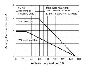
Fig. 1 - Forward Current Derating Curve
