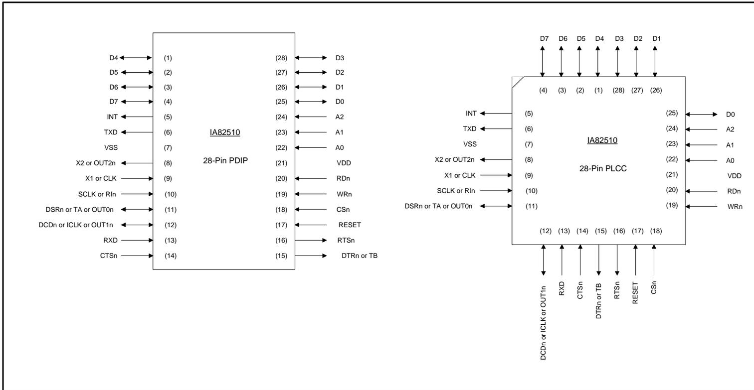
**Figure 1. Package Pinout**
