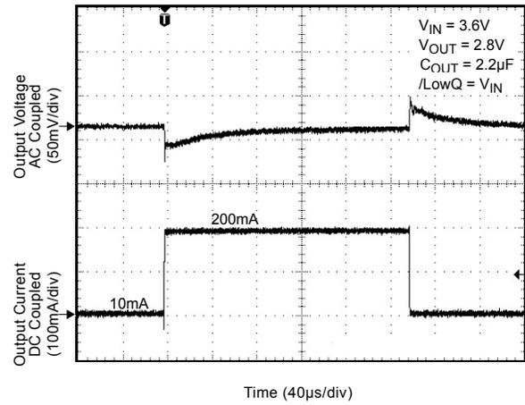
**DC/DC<sub>[LOWQ Mode]</sub> Load Transient**
