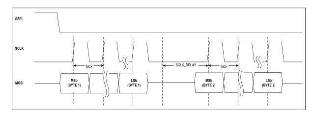
The length of the delay is a function of the SPI clock frequency as shown in the following table. The SPI master must be operated in sample mode with a maximum frequency of 24MHz.
