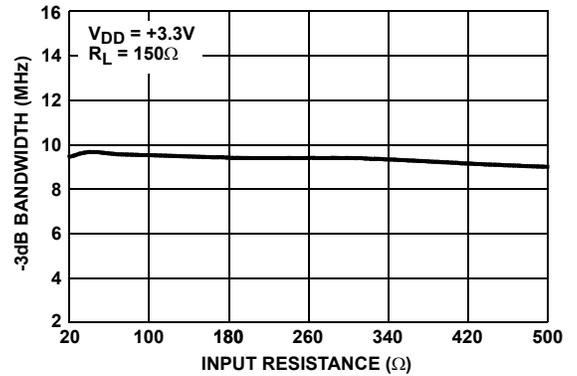
FIGURE 18. -3dB BANDWIDTH vs INPUT RESISTANCE
