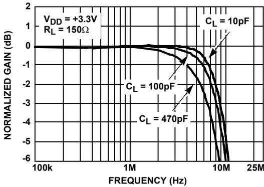
FIGURE 3. GAIN vs FREQUENCY FOR VARIOUS  $C_{LOAD}$
