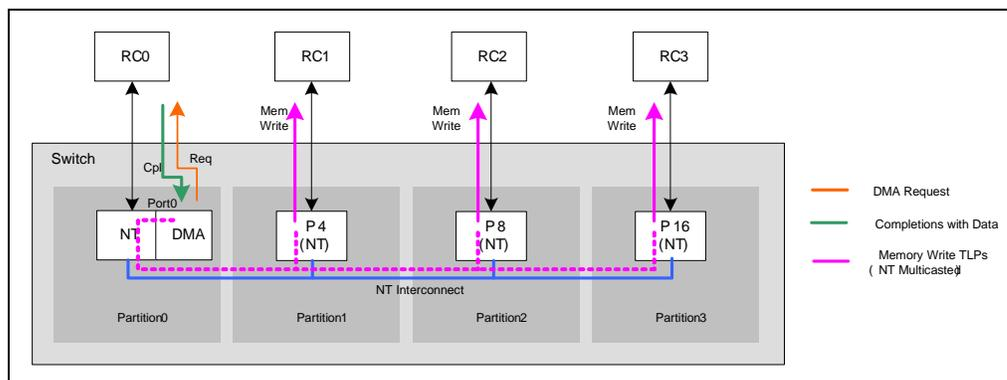
Figure 26.20 PES32NT8xG2 with Port 0 Configured in NT Function with DMA Mode and Ports 4, 8, and 16 in NT Function Mode
