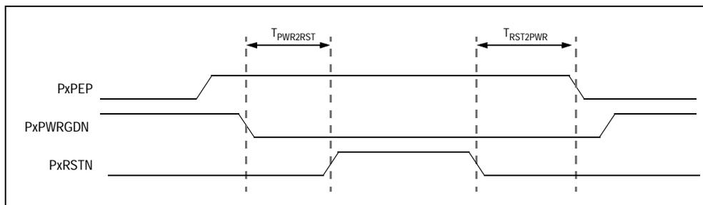
Figure 11.5 Power Good Controlled Reset Output Mode Operation
