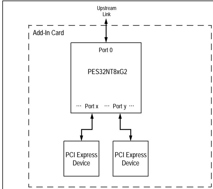
Figure 11.2 Hot-Plug with Switch on Add-In Card Application
