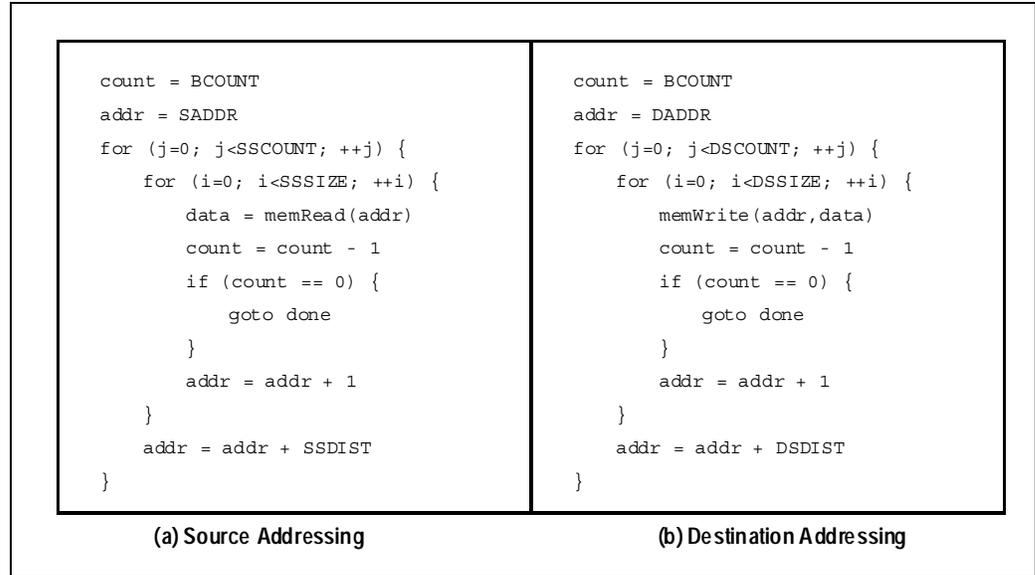
Figure 15.4 DMA Channel Addressing<sup>1</sup>
