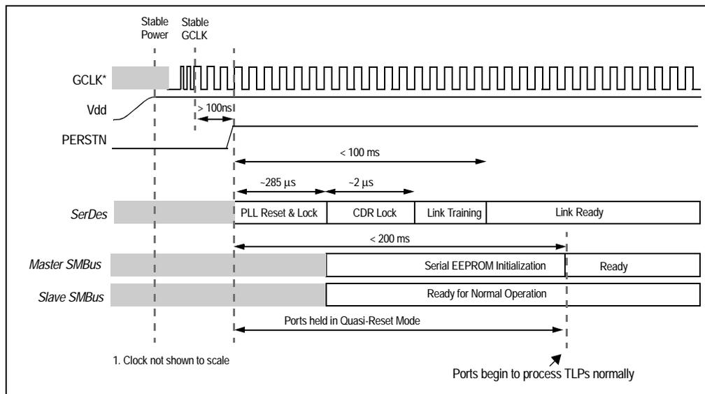
Figure 3.1 Switch Fundamental Reset with Serial EEPROM Initialization
