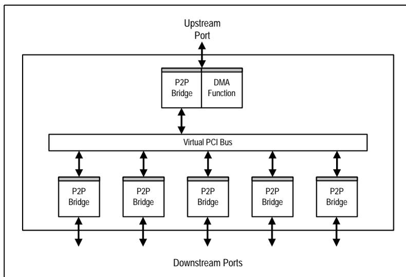
Figure 1.12 Switch Partition with DMA function
