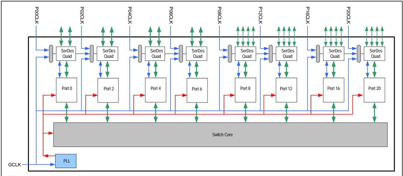
Figure 2.1 Logical Representation of PES32NT8AG2 Clocking Architecture
