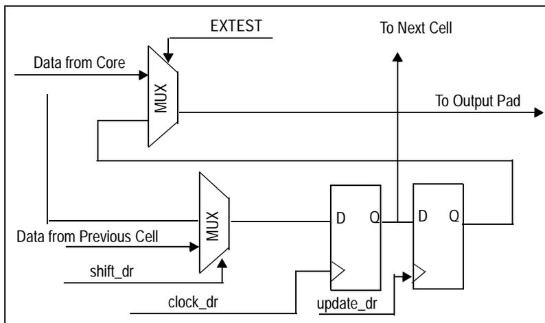
Figure 25.4 Diagram of Output Cell
