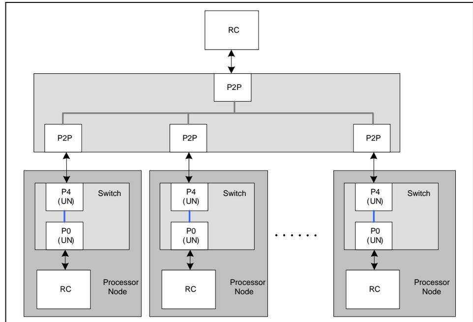
Figure 26.10 System Configuration Immediately after Switch Fundamental Reset
