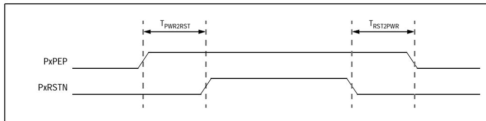
Figure 11.4 Power Enable Controlled Reset Output Mode Operation
