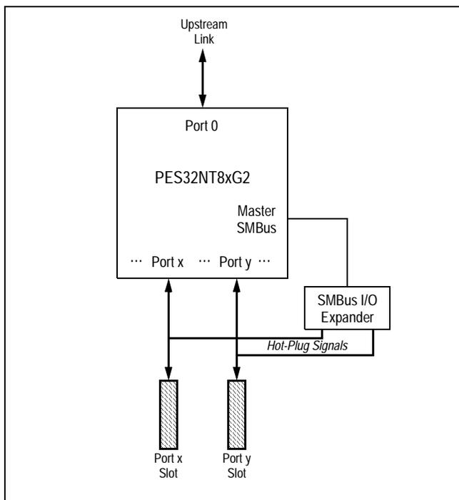
Figure 11.1 Hot-Plug on Switch Downstream Slots Application
