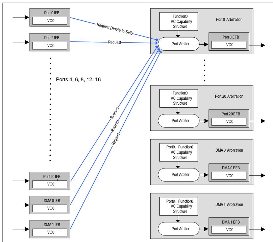
Figure 4.2 Architectural Model of Arbitration
