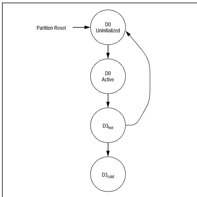
Figure 9.1 PES32NT8xG2 Power Management State Transition Diagram
