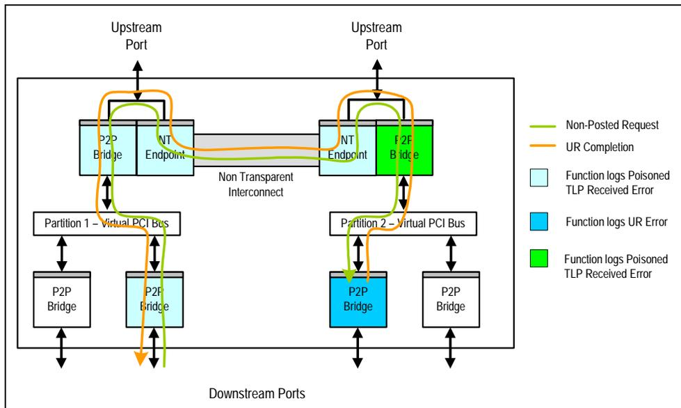
Figure 14.17 Example of Combined Transaction Layer Error Handling
