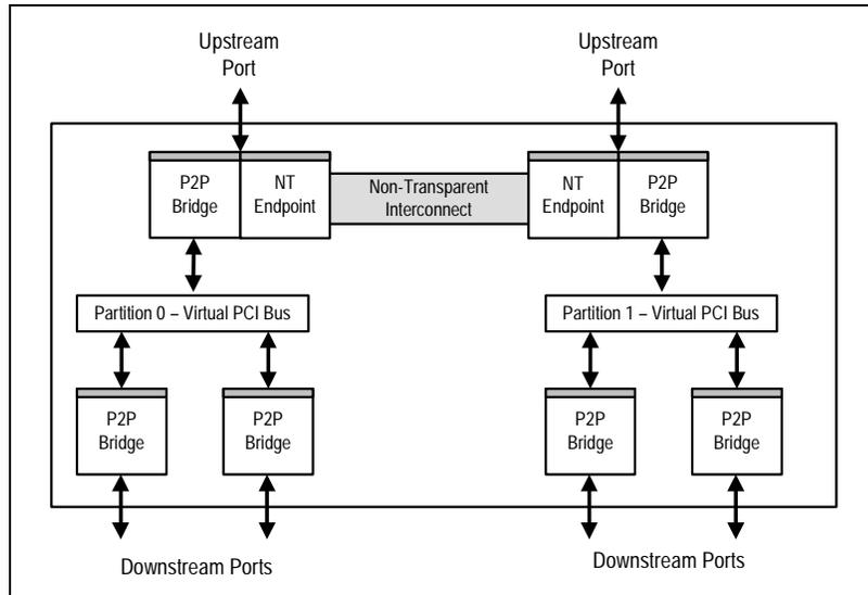
Figure 1.8 Non-Transparent Switch with Non-Transparency Between Partitions
