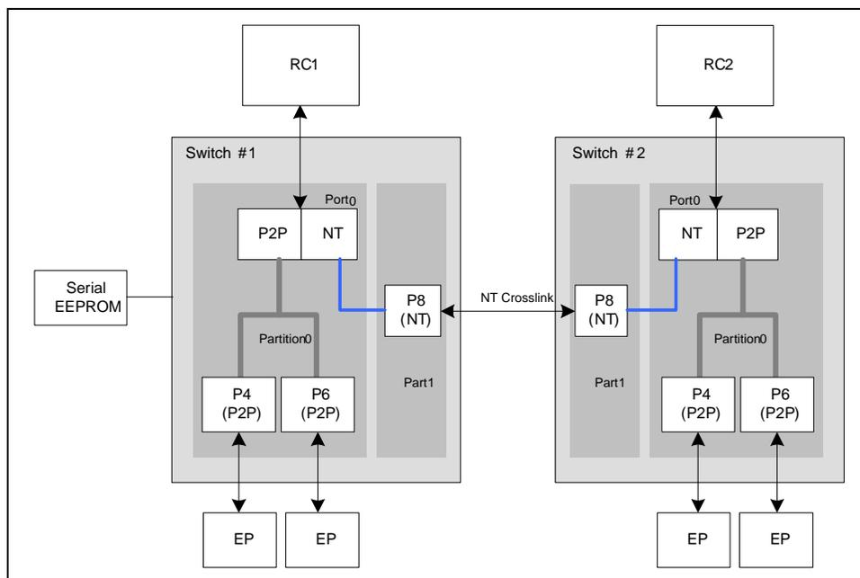
Figure 26.9 System Configuration after Serial EEPROM Initialization
