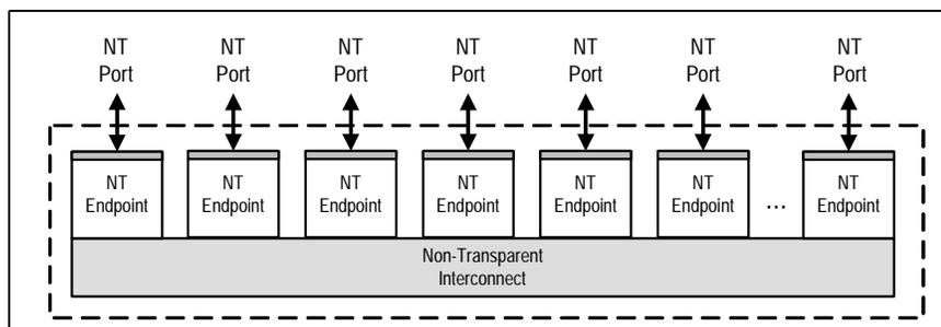
Figure 1.10 Non-Transparent Switch with Non-Transparent Ports
