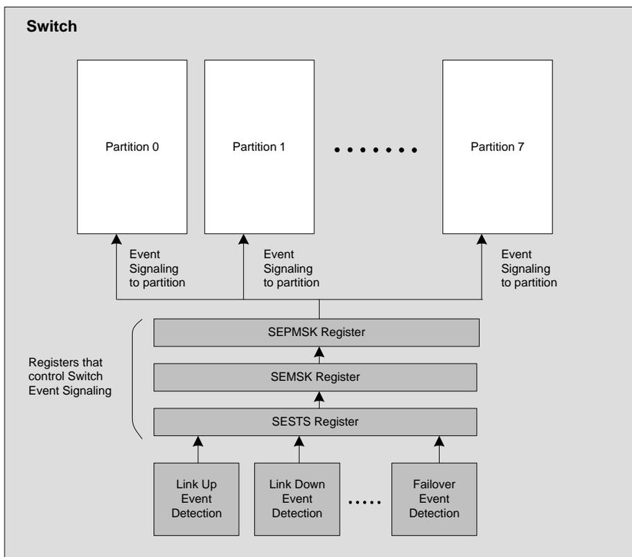
Figure 16.1 Switch Event Detection and Signaling Mechanism
