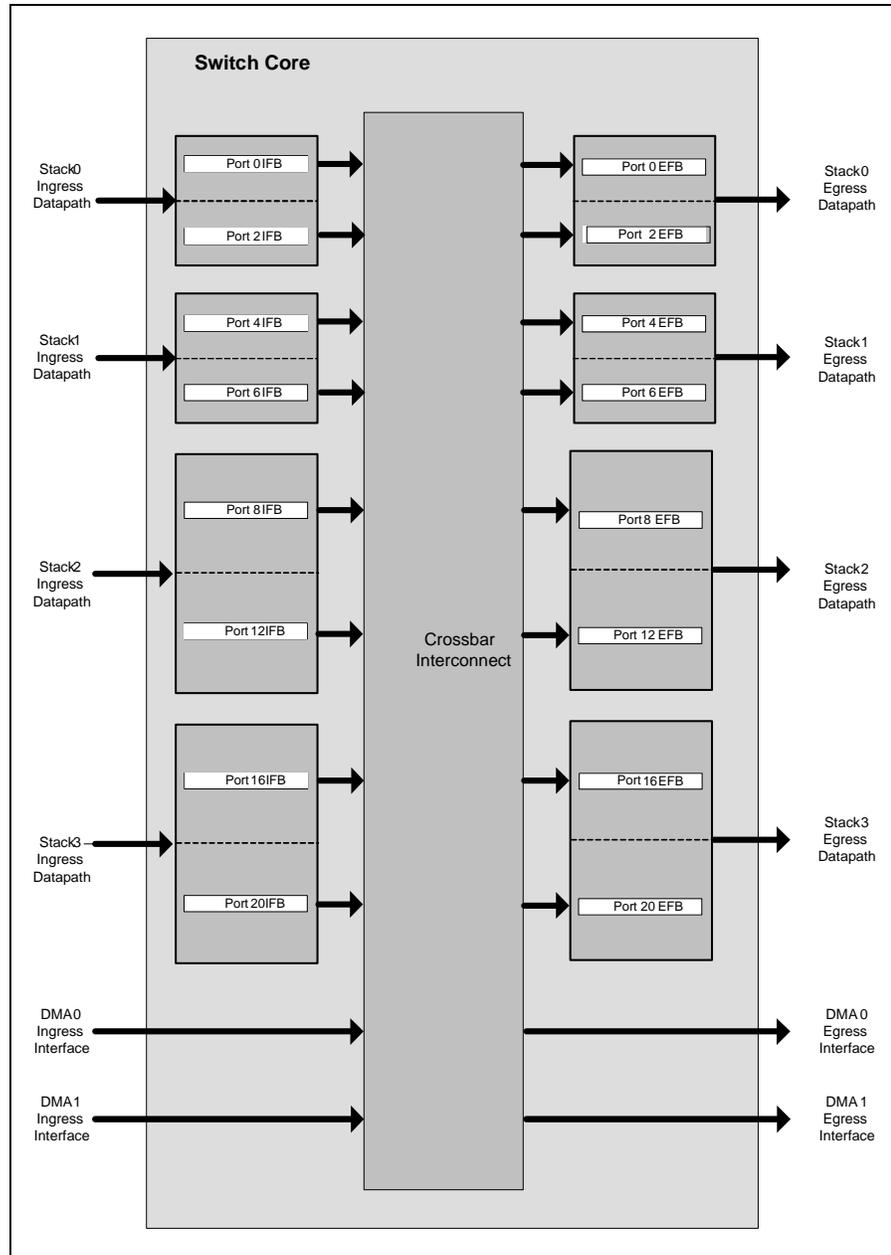
Figure 4.1 High Level Diagram of Switch Core
