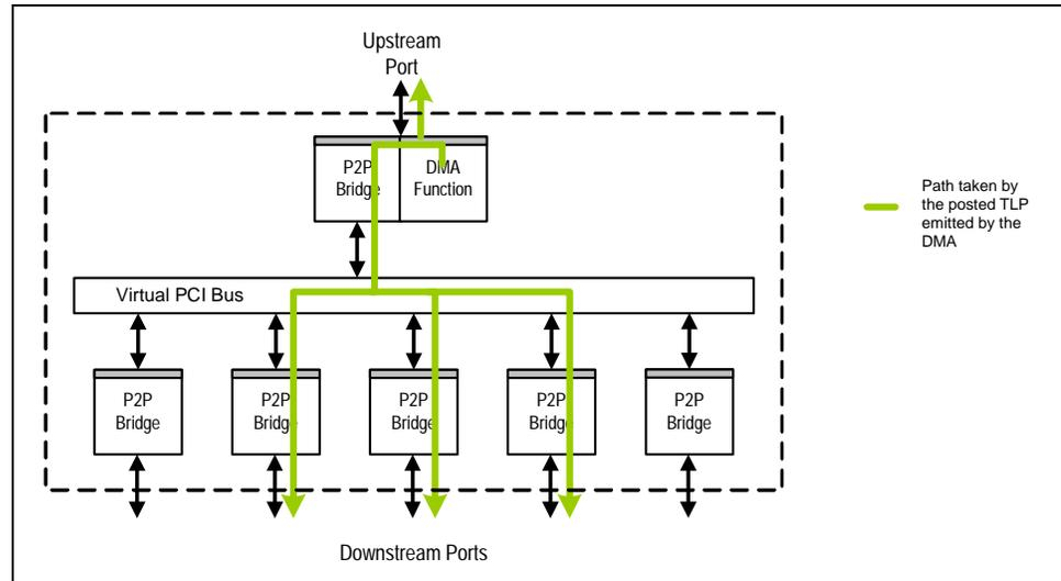
Figure 15.12 Path Taken by a TLP Emitted by the DMA When it is Multicast<sup>1</sup>
