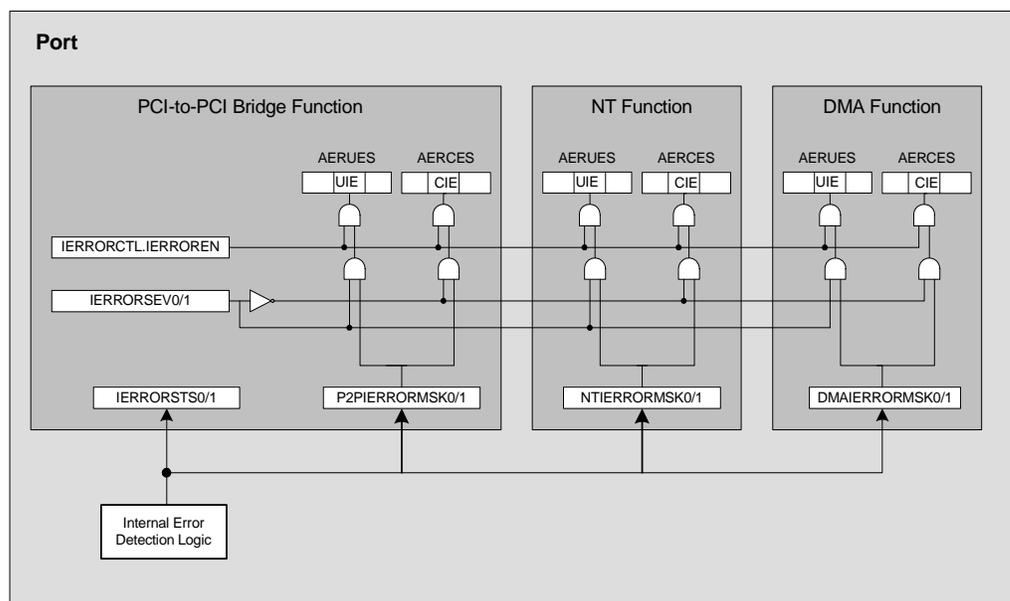
Figure 4.7 Internal Error Logic in Each PES32NT8xG2 Port
