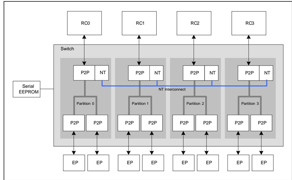
Figure 26.7 Multiprocessor System Interconnection Using the PES32NT8xG2
