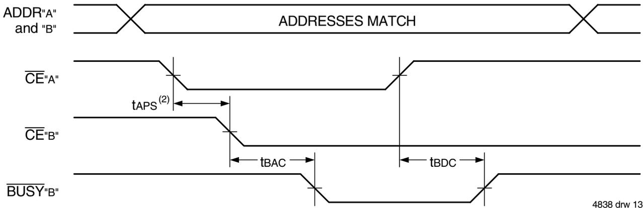
**Waveform of  $\overline{BUSY}$  Arbitration Cycle Controlled by Address Match Timing ( $M/\overline{S} = V_{IH}$ )<sup>(1)</sup>**
