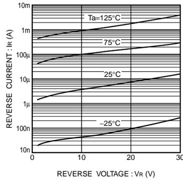
Fig. 2 Reverse characteristics
