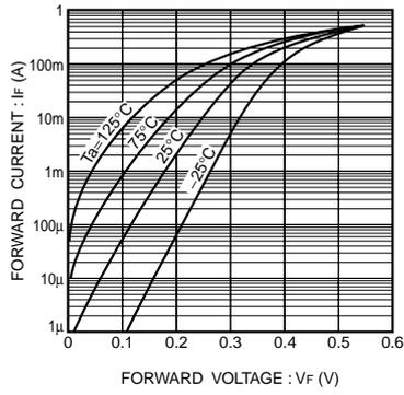
Fig. 1 Forward characteristics
