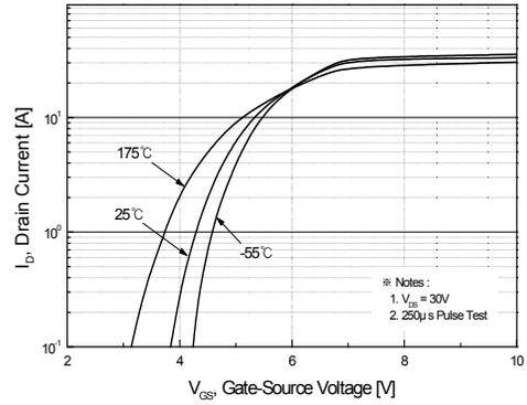
Figure 2. Transfer Characteristics
