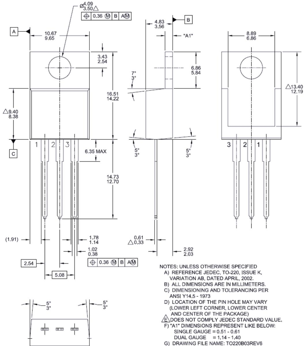
**Figure 16. TO-220, Molded, 3-Lead, Jedec Variation AB**
