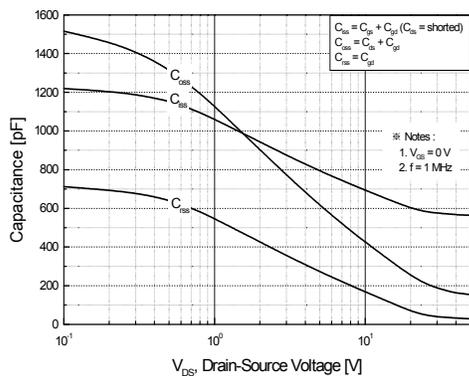
Figure 5. Capacitance Characteristics
