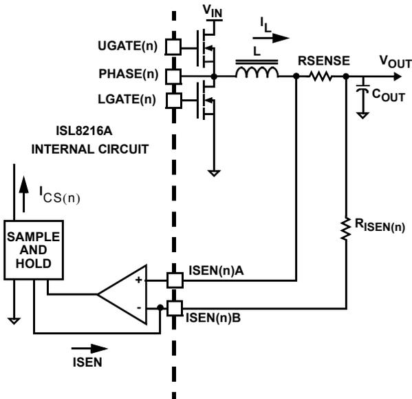
FIGURE 21. SENSE RESISTOR IN SERIES WITH INDUCTOR
