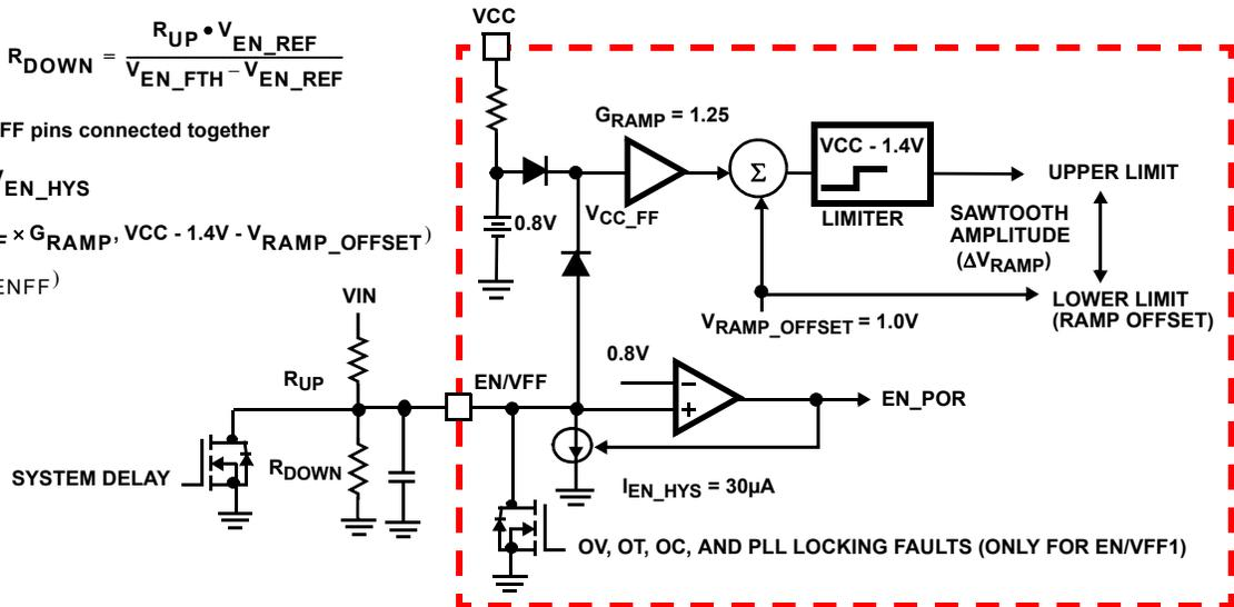
FIGURE 12. SIMPLIFIED ENABLE AND VOLTAGE FEED-FORWARD CIRCUIT
