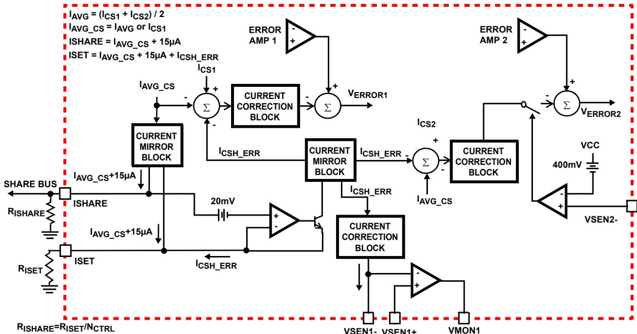
FIGURE 23. SIMPLIFIED CURRENT SHARE AND INTERNAL BALANCE IMPLEMENTATION
