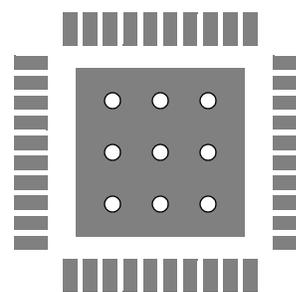
FIGURE 35. PCB VIA PATTERN
