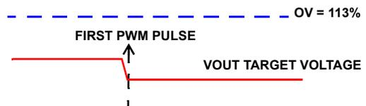
FIGURE 16. SOFT-START WITH VOUT BELOW 0V BUT ABOVE FINAL TARGET VOLTAGE
