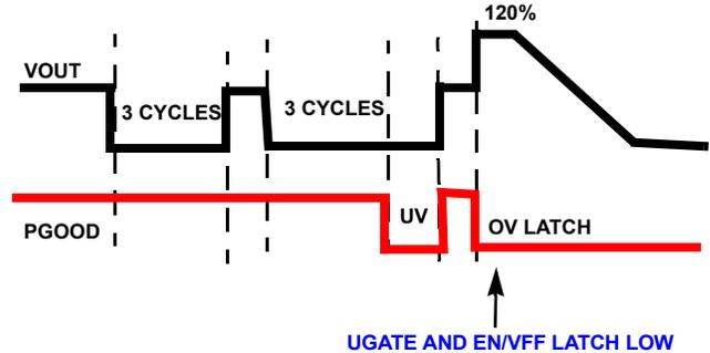
FIGURE 19. PGOOD TIMING UNDER UV AND OV
