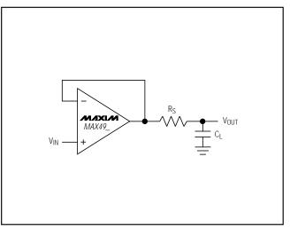
Figure 8. Capacitive-Load Driving Circuit
