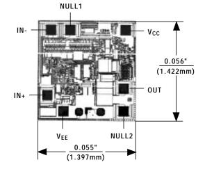
TRANSISTOR COUNT: 134 (single MAX495) 268 (dual MAX492) 536 (quad MAX494) SUBSTRATE CONNECTED TO VFF
