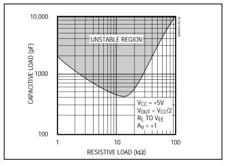
Figure 5. Capacitive-Load Stable Region Sourcing Current
