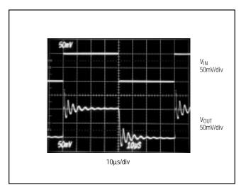
Figure 9a. Driving a 10,000pF Capacitive Load
