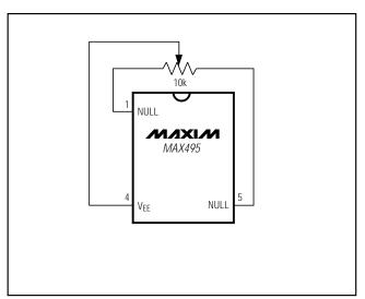
Figure 2. Offset Null Circuit
