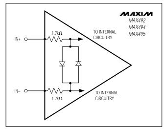
Figure 4. Input Stage Protection Circuitry
