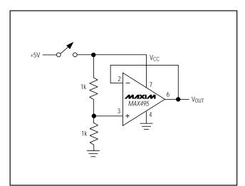
Figure 10. Power-Up Test Configuration
