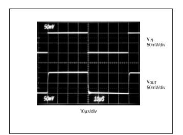
Figure 7a. MAX492 Voltage Follower with 500pF Load—  $R_L = 5k\Omega$
