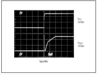
Figure 11b. Power-Up Settling Time ( $V_{CC} = +5V$ )
