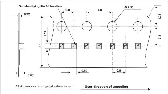
Figure 12. Tape and reel specifications
