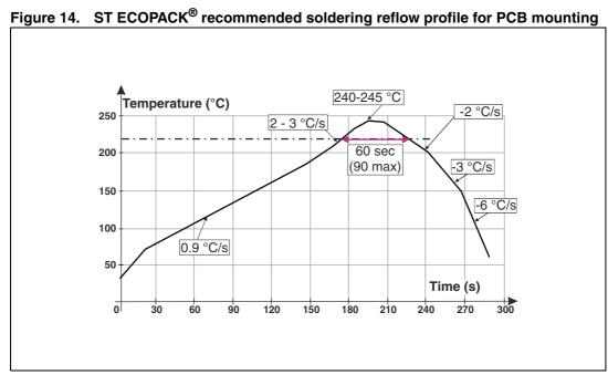
Note: Minimize air convection currents in the reflow oven to avoid component movement.
