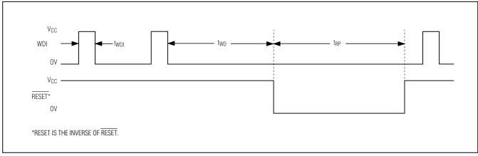
Figure 3. Detailed Watchdog Input Timing Relationship
