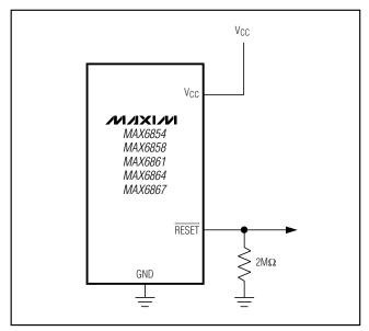
Figure 5. Ensuring RESET Valid to VCC = Ground
