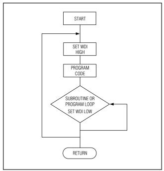
Figure 6. Watchdog Flow Diagram
