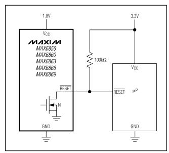
Figure 4. Interfacing with Other Voltage Levels
