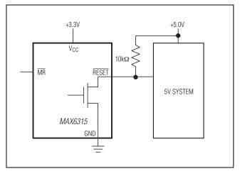
Figure 1. MAX6315 Open-Drain RESET Output Allows Use with Multiple Supplies
