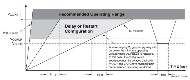
Figure 9: V<sub>CCINT</sub> Power-Up Requirements
