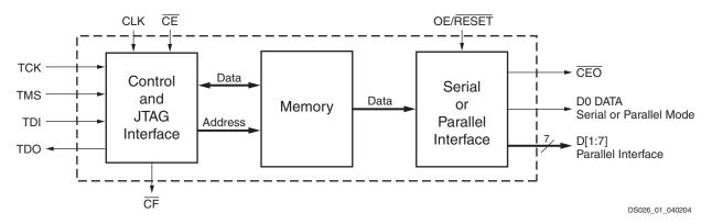
Figure 1: XC18V00 Series Block Diagram
