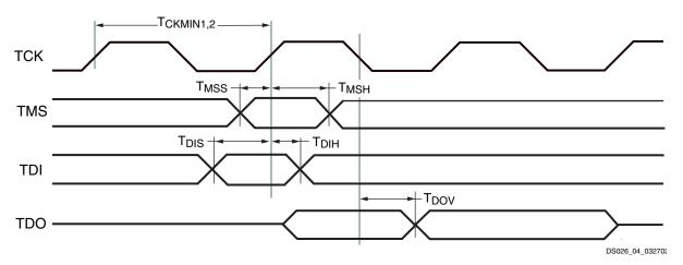
Figure 4: Test Access Port Timing
