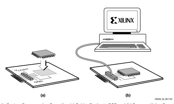
Figure 2: In-System Programming Operation (a) Solder Device to PCB and (b) Program Using Download Cable
