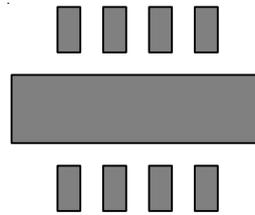
(c) Copper Area =  $30 \text{ mm}^2$ ,  $\theta_{JA} = 54^\circ\text{C/W}$
