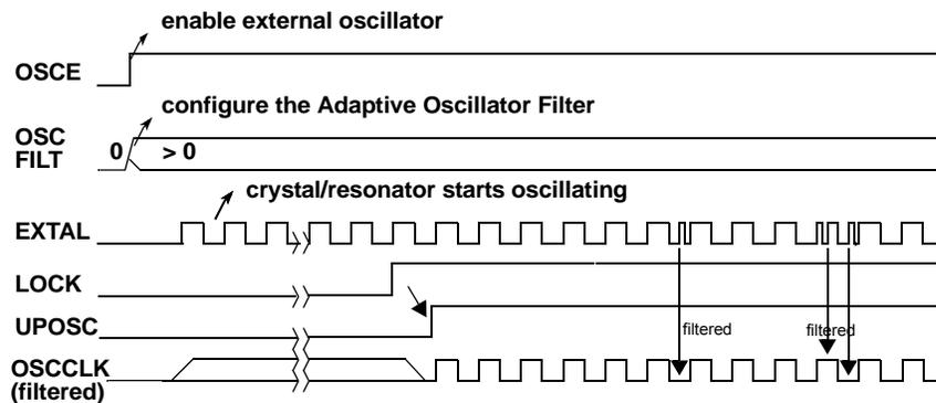
Figure 91. Noise Filtered by the Adaptive Oscillator Filter
