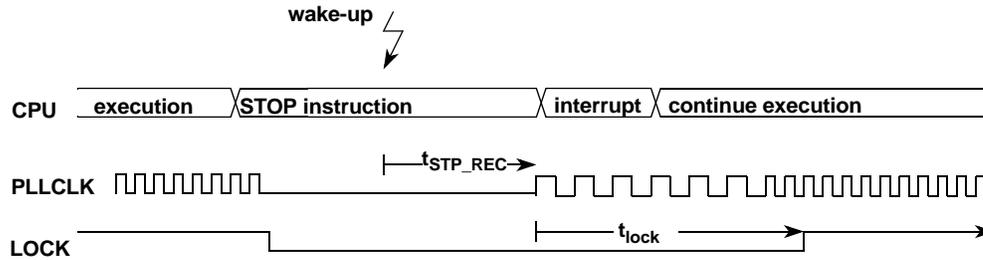
Figure 88. Stop Mode Using PLLCLK as Bus Clock
