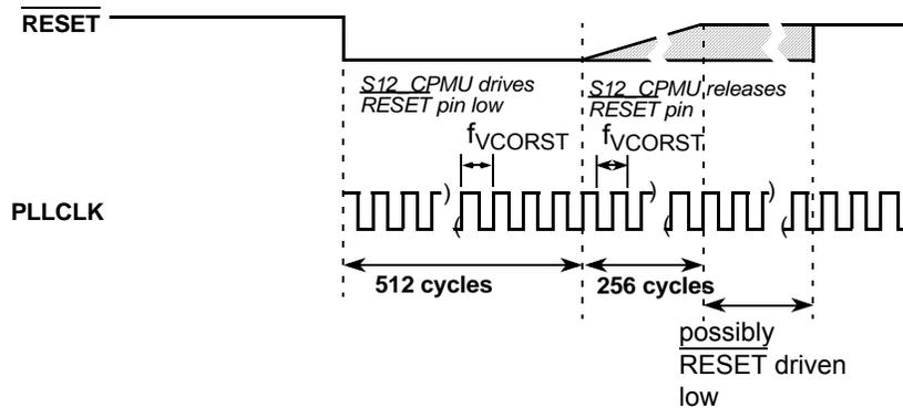
**Figure 93. RESET Timing**
