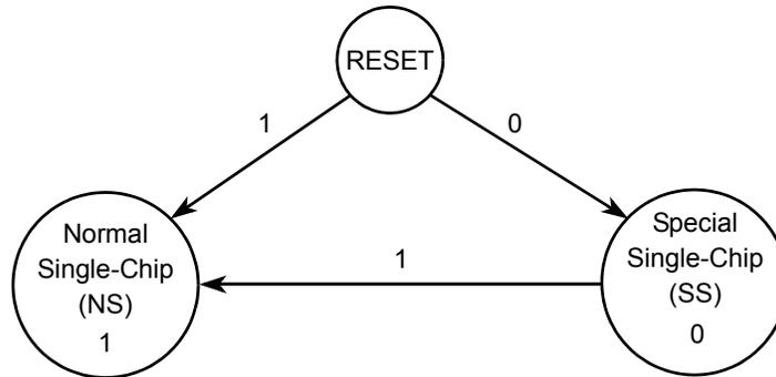
**Figure 45. Mode Transition Diagram When MCU is Unsecured**
