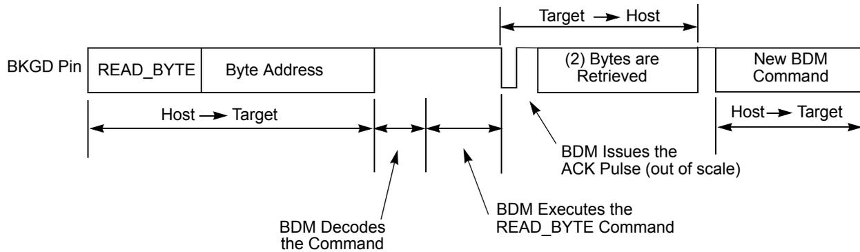
**Figure 59. Handshake Protocol at the Command Level**
