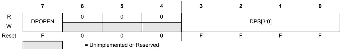
The (unreserved) bits of the DFPROT register are writable with the restriction that protection can be added but not removed. Writes must increase the DPS value and the DPOPEN bit can only be written from 1 (protection disabled) to 0 (protection enabled). If the DPOPEN bit is set, the state of the DPS bits is irrelevant.
