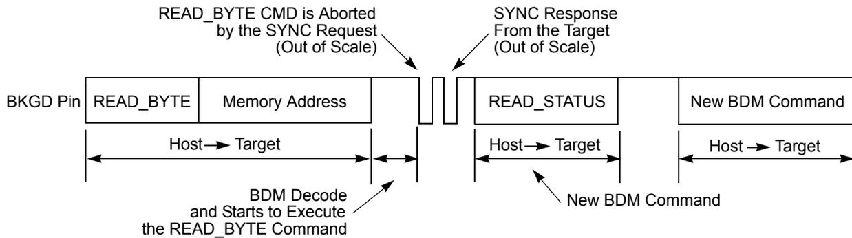
**Figure 60. ACK Abort Procedure at the Command Level**
