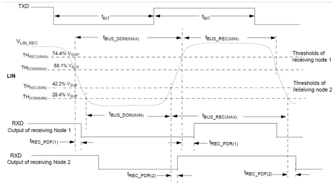
Figure 6. LIN Timing Measurements for Normal Baud Rate
