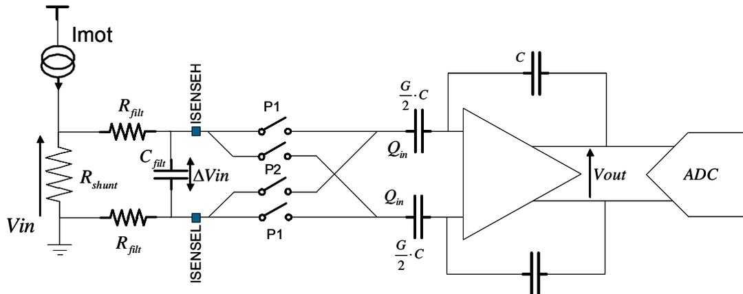
Figure 37. Current Sense Module with External Filter Option
