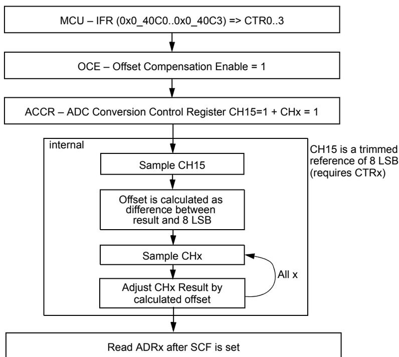
**Figure 36. Automatic Offset Compensation**
