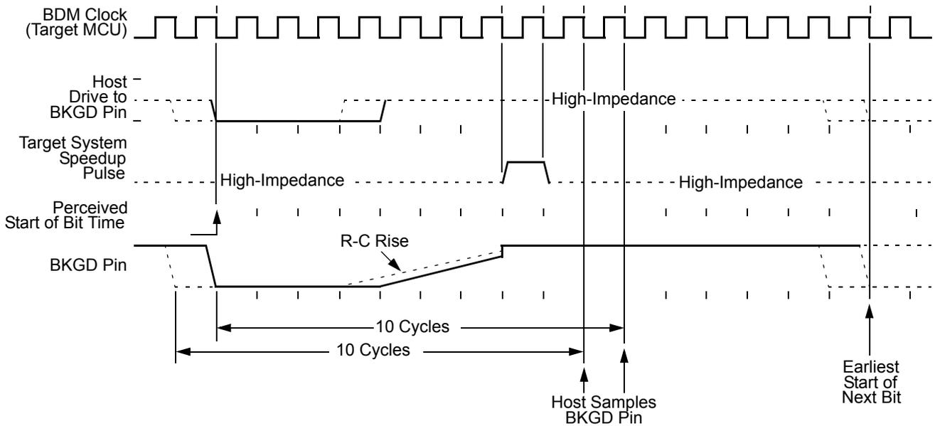
**Figure 56. BDM Target-to-Host Serial Bit Timing (Logic 1)**
