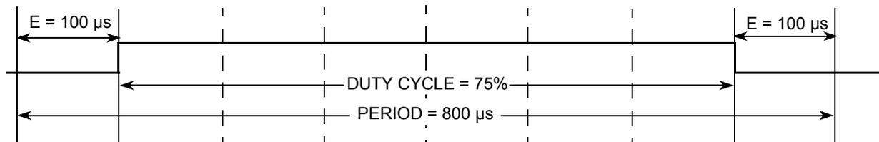
**Figure 28. PWM Center Aligned Output Example Waveform**
