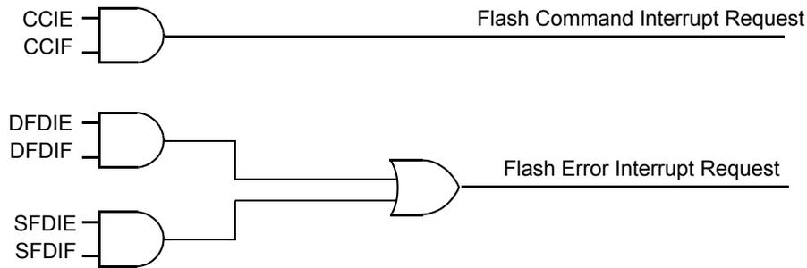
**Figure 108. Flash Module Interrupts Implementation**
