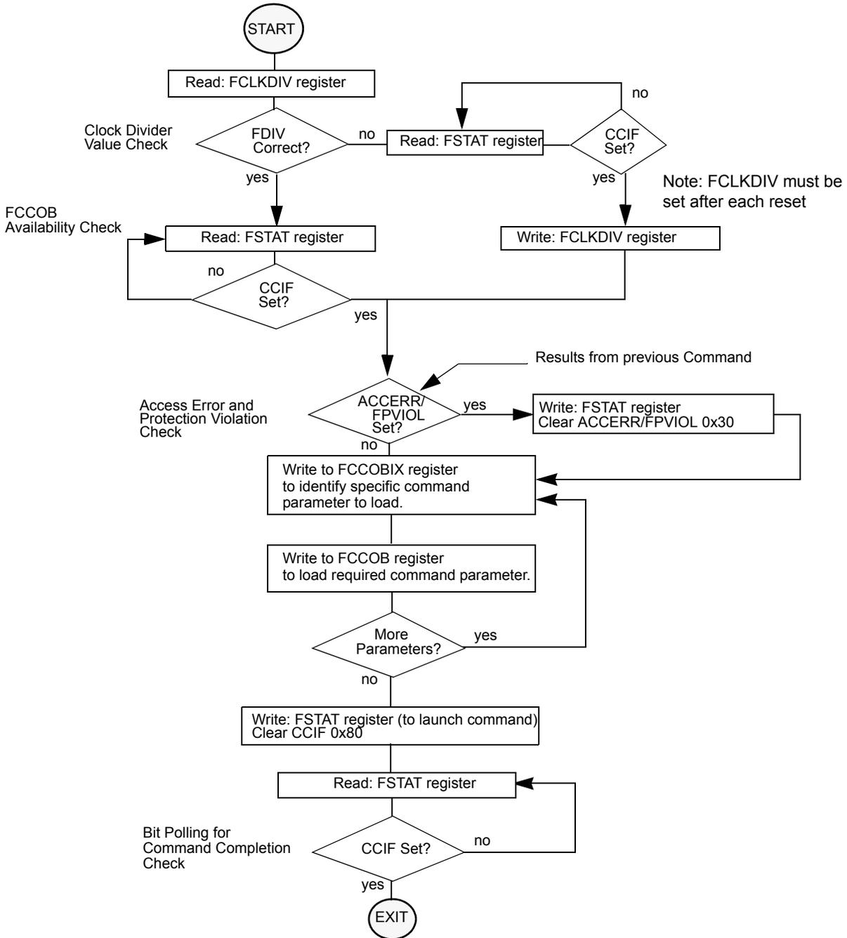
Figure 107. Generic Flash Command Write Sequence Flowchart
