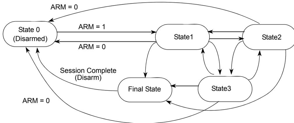
Figure 64. State Sequencer Diagram
