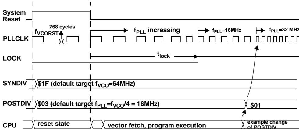
**Figure 87. Startup of Clock System After Reset**
