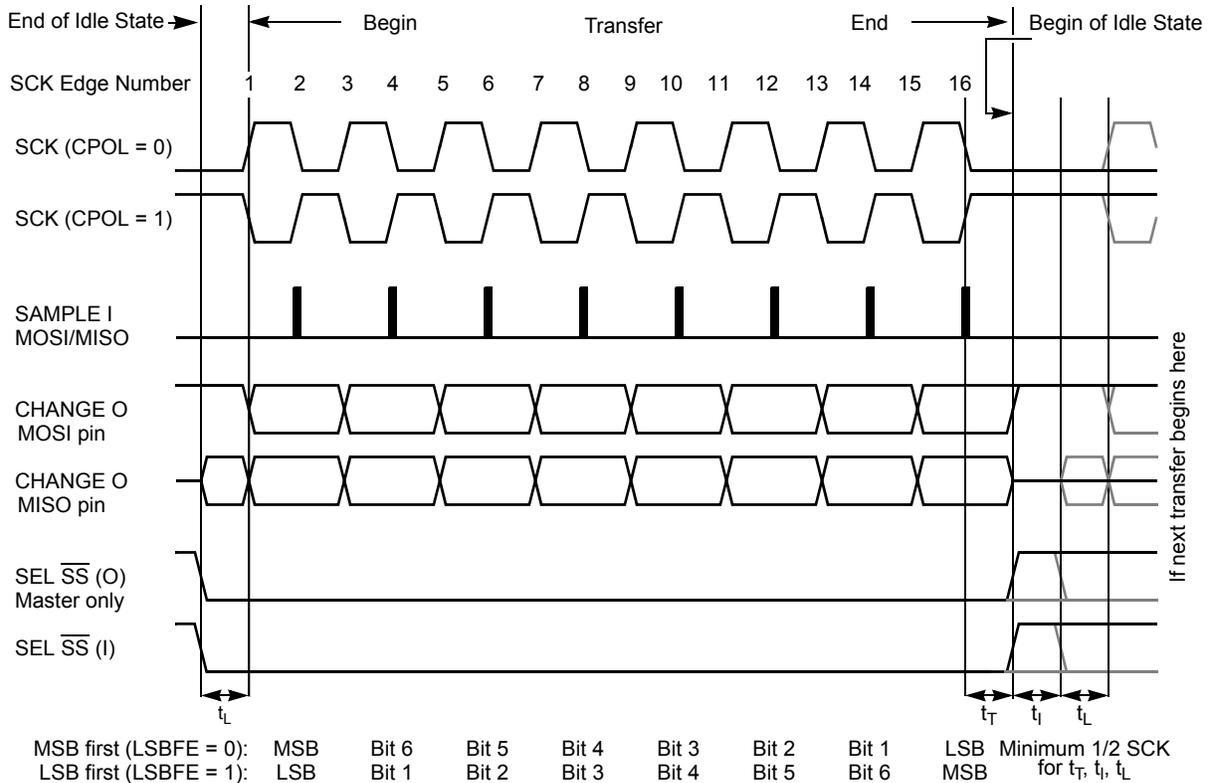
$t_L$  = Minimum leading time before the first SCK edge, not required for back-to-back transfers
