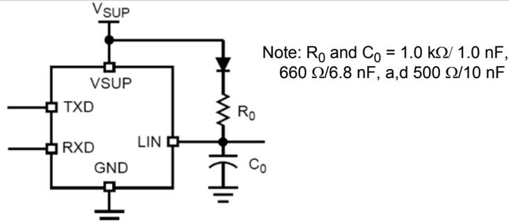
Figure 5. Test Circuit for Timing Measurements
