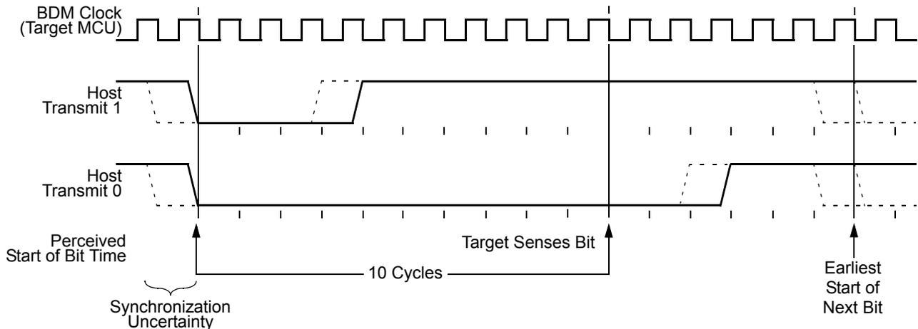
Figure 55. BDM Host-to-Target Serial Bit Timing
