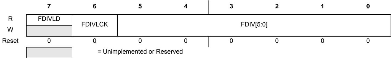
All bits in the FCLKDIV register are readable, bit 7 is not writable, bit 6 is write-once-hi and controls the writability of the FDIV field.
