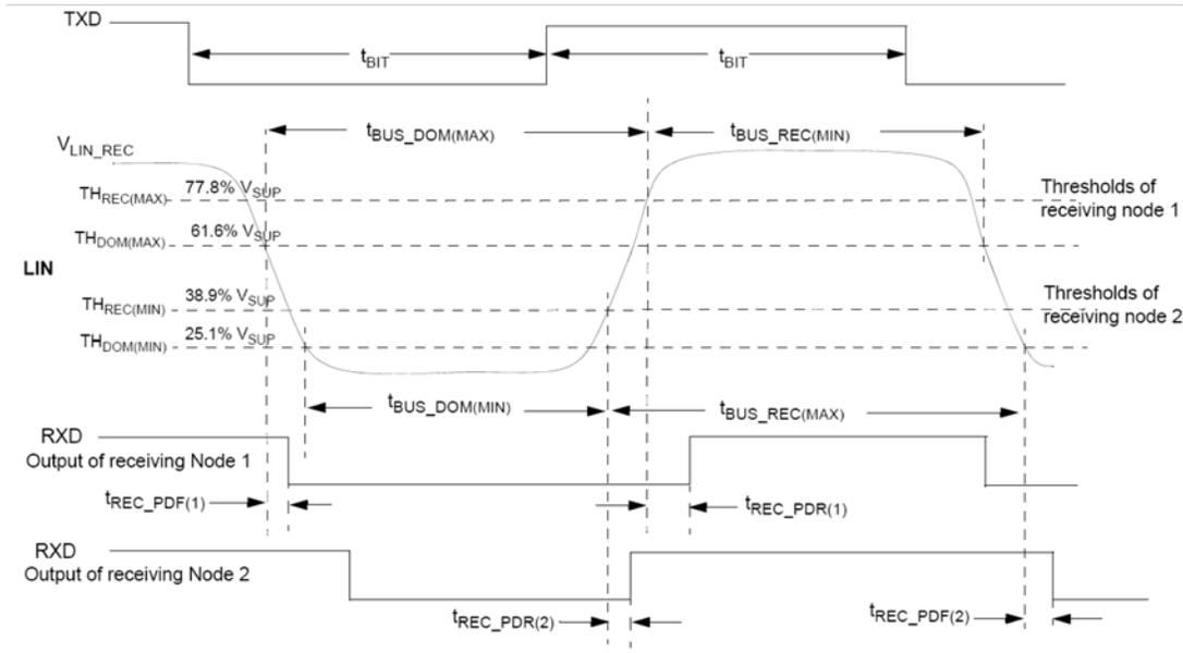
Figure 7. LIN Timing Measurements for Slow Baud Rate
