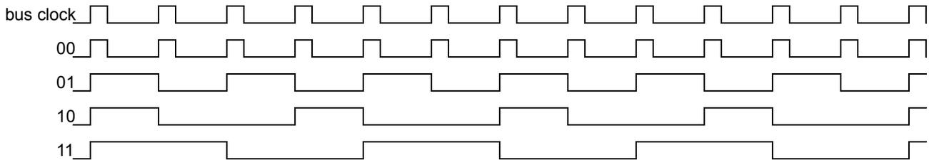
**Figure 111. Interface Clock Waveforms for various D2DCLKDIV Encoding**
