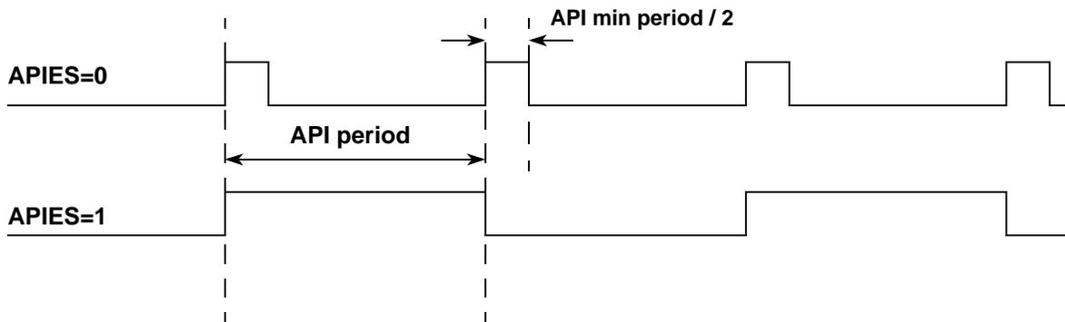
**Figure 84. Waveform selected on API\_EXTCLK pin (APIEA=1, APIFE=1)**
