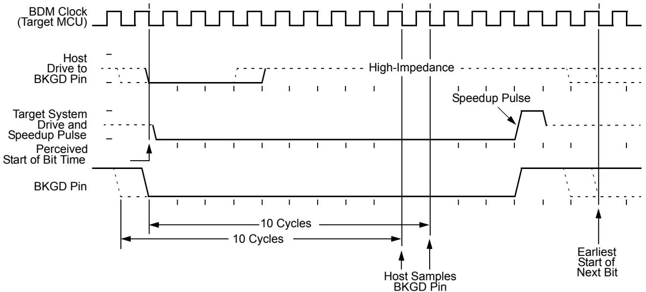
**Figure 57. BDM Target-to-Host Serial Bit Timing (Logic 0)**
