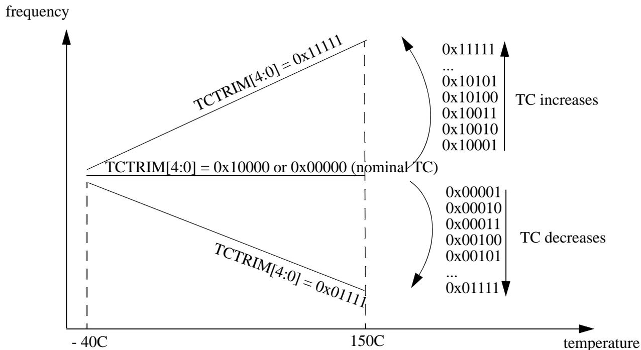
**Figure 86. Influence of TCTRIM[4:0] on the Temperature Coefficient**
