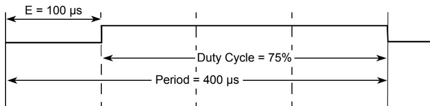
**Figure 26. PWM Left Aligned Output Example Waveform**
