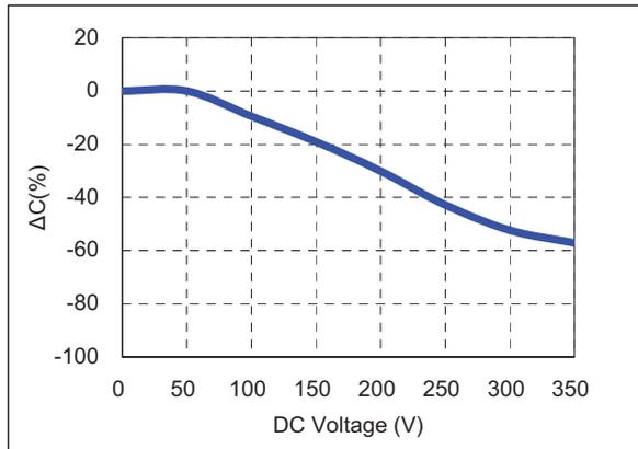
4) Bias TCC characteristics (Agilent 4284A, 1kHz, 1Vrms, 175Vdc)
