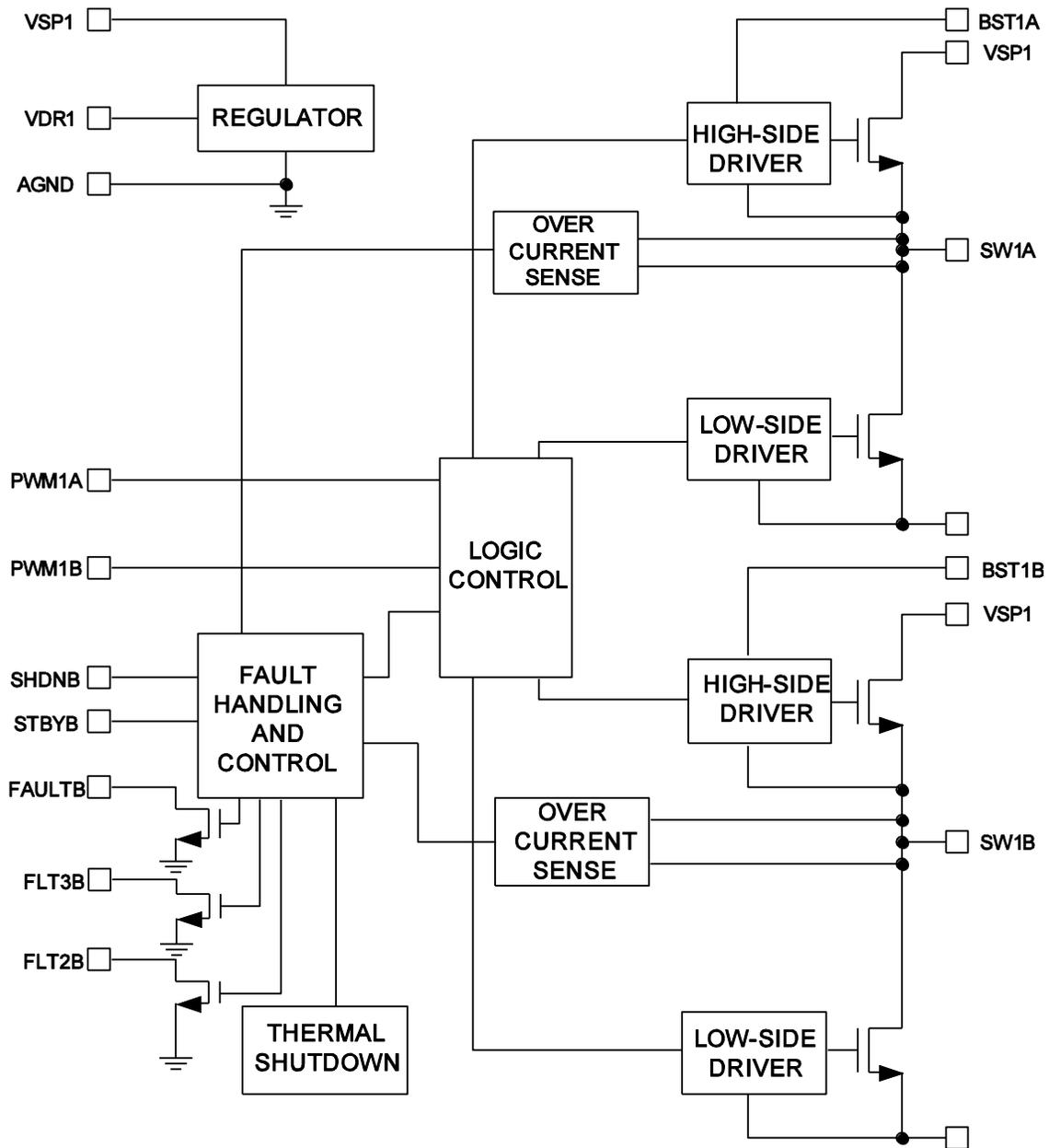
Figure 2—Function Block Diagram (1 full bridge channel only)
