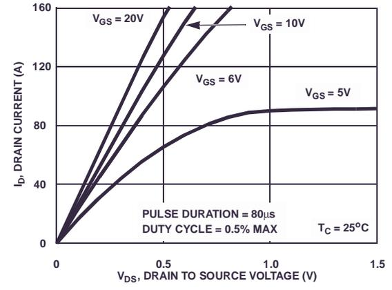
**Figure 8. Saturation Characteristics**
