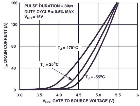
**Figure 7. Transfer Characteristics**
