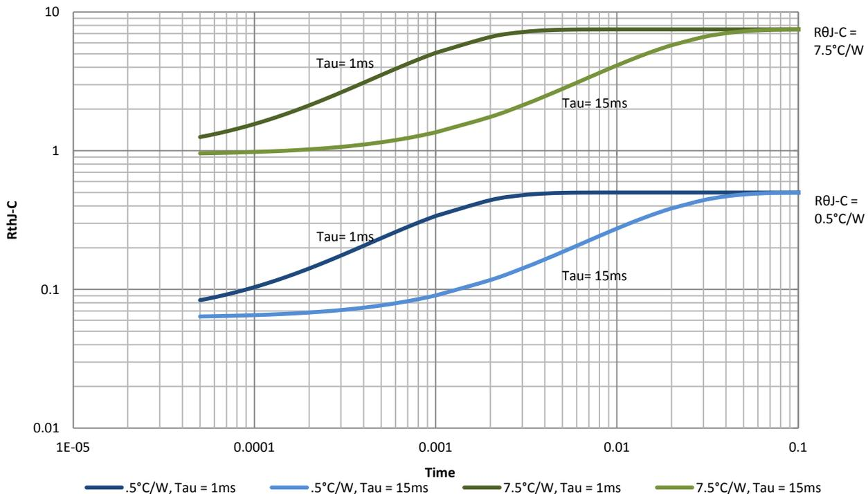
Figure 3 - The range of PI2211  $R_{\theta_{j-c}}$  thermal impedance adjustment at 1W.
