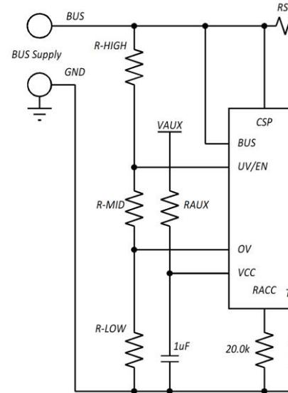
Figure 6 - External VAUX connection for lower BUS voltages.
