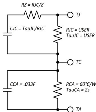
Figure 2 - Simplified representation of the PI2211 thermal model.
