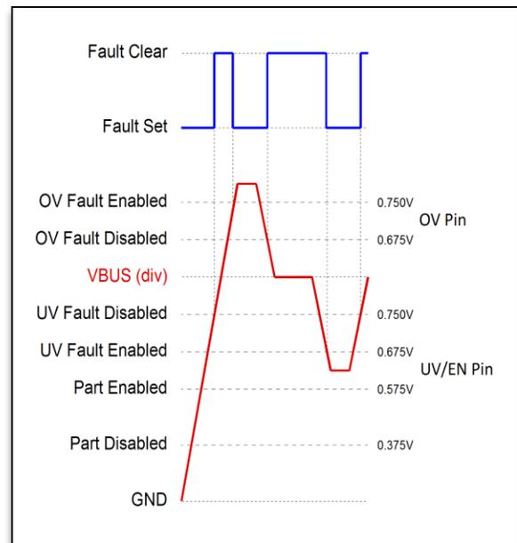
Figure 7 - Enable, UV and OV thresholds.
