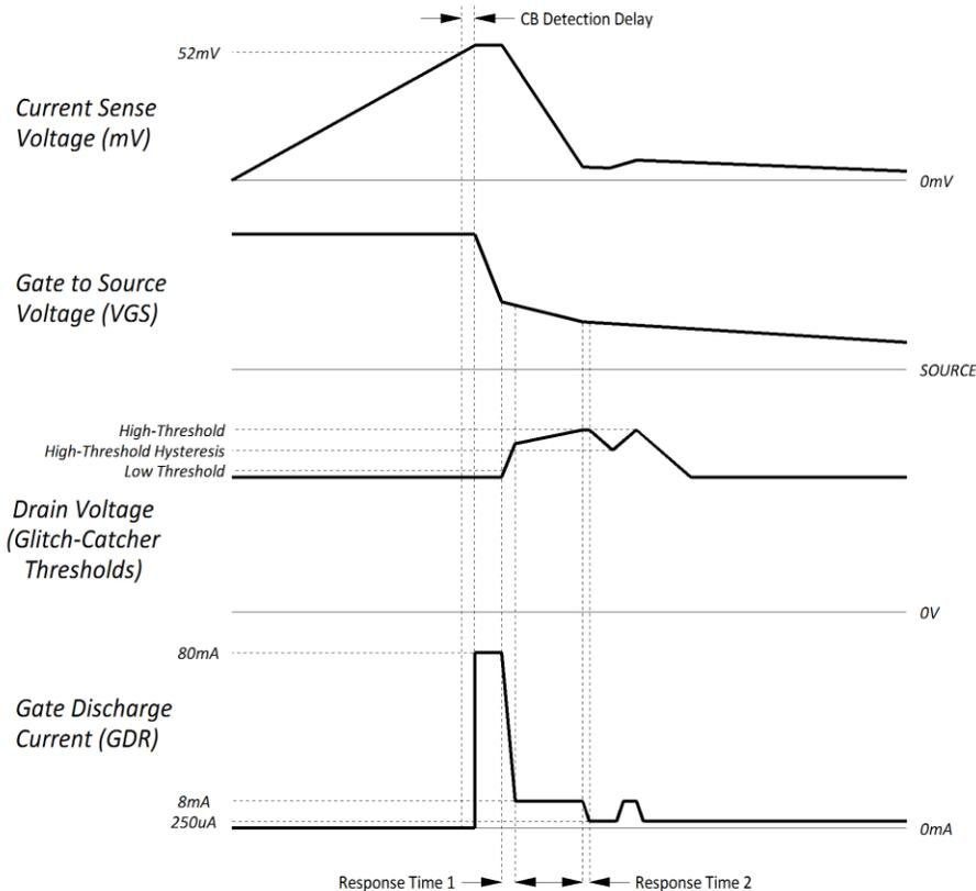
**Figure 9 - Circuit Breaker (CB) and Glitch-Catcher™ waveforms.**
