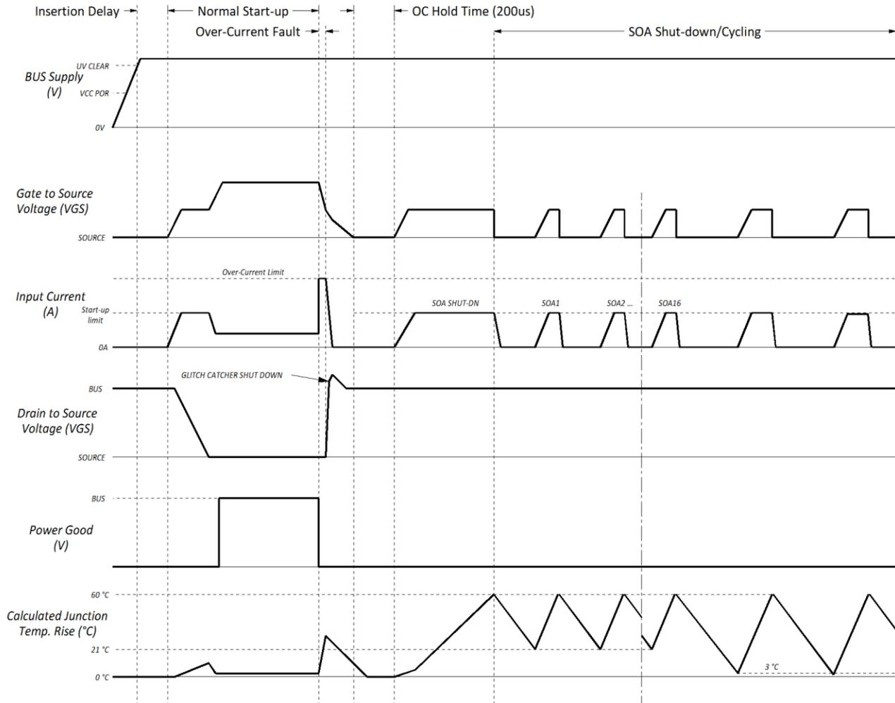
Figure 11 - Start-up, Over-Current, and SOA shut-down waveforms.
