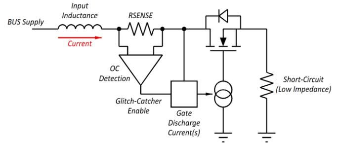
**Figure 8 - Glitch-Catcher™ Over-current fault detection circuit.**
