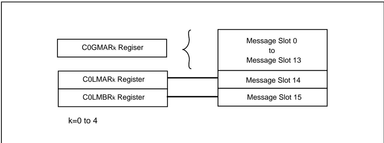
**Figure 23.27 Mask Registers and Message Slots**
