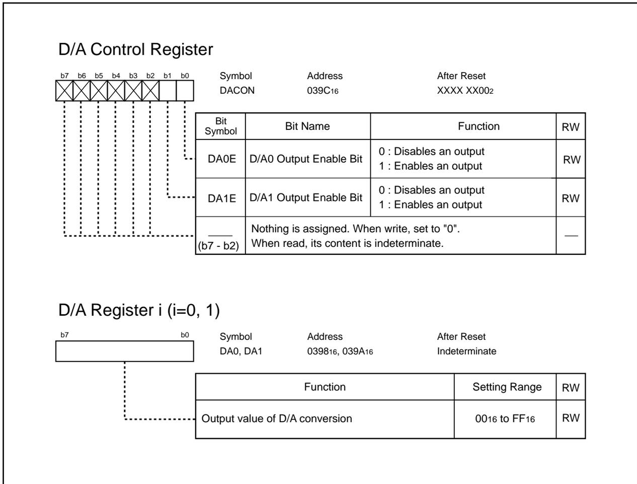
**Figure 19.2 DACON Register, DA0 and DA1 Registers**
