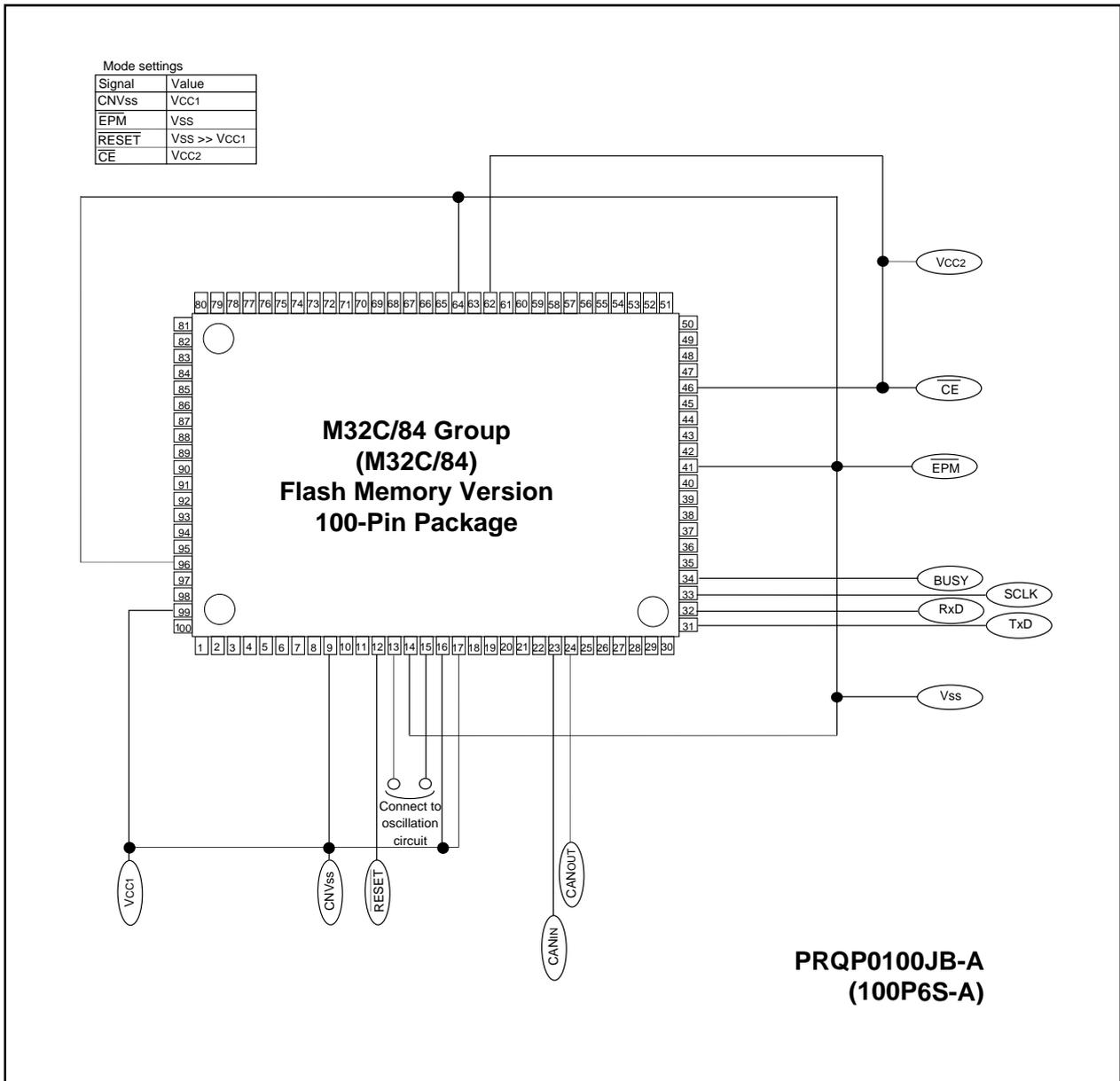
Figure 25.14 Pin Connections in Standard Serial I/O Mode (1)
