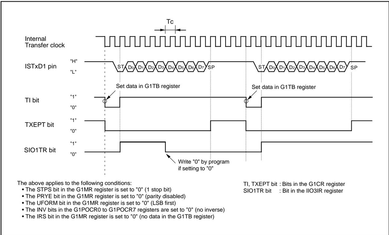
**Figure 22.31 Transmit Operation**
