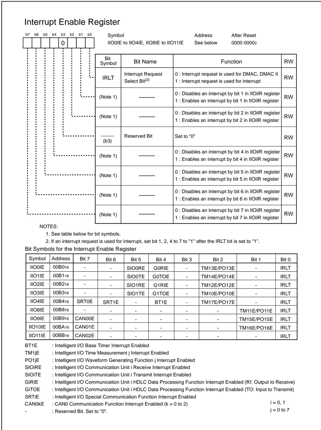
Figure 11.15 IIO0IE to IIO4IE, IIO8IE to IIO11IE Registers
