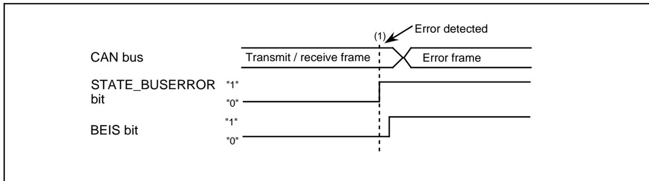
Figure 23.40 Operation Timing when CAN Bus Error Occurs
