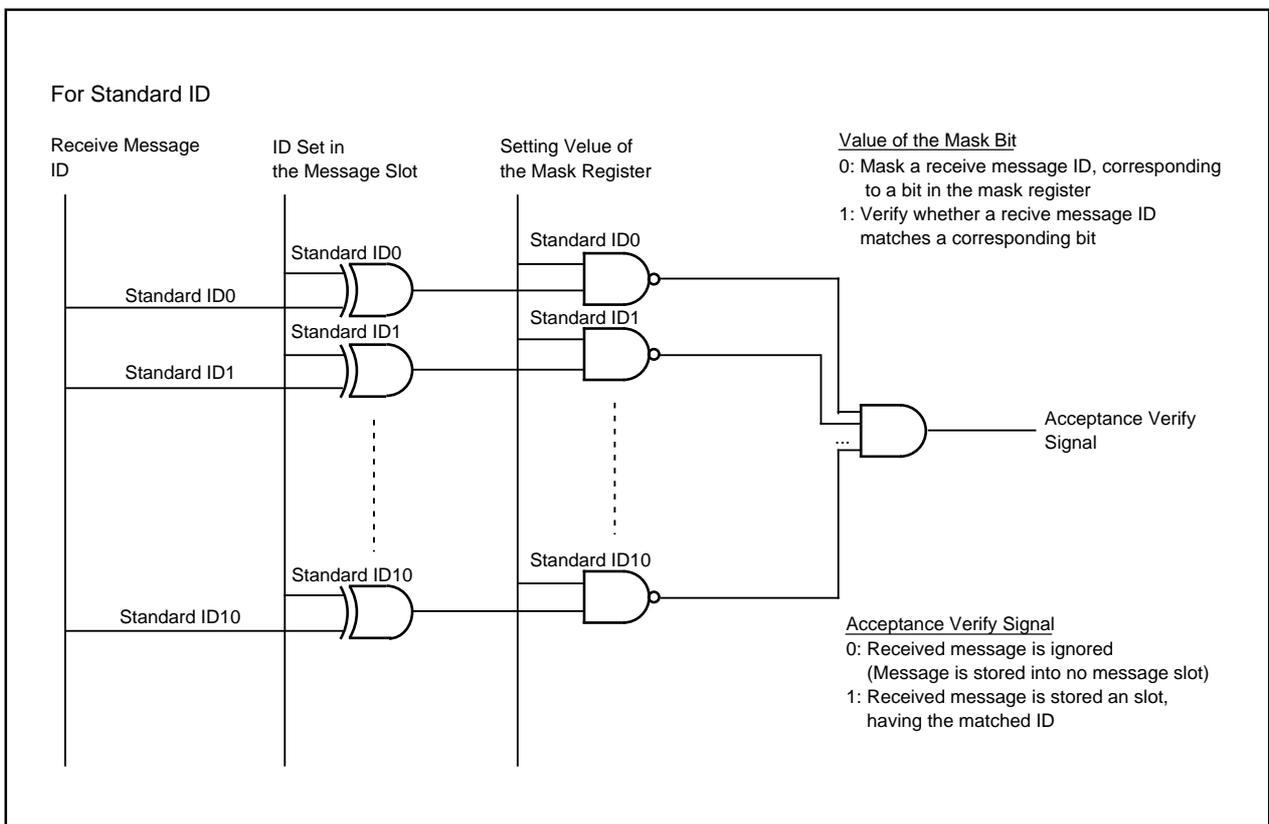
**Figure 23.28 Acceptance Filtering**
