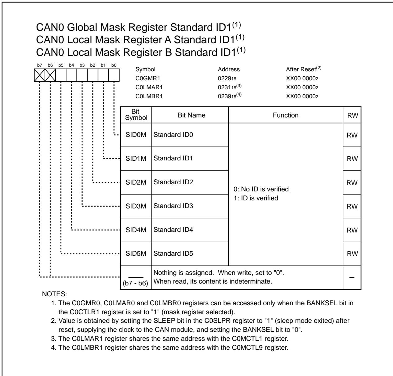
**Figure 23.23 C0GMR1, C0LMAR1 and C0LMBR1 Registers**
