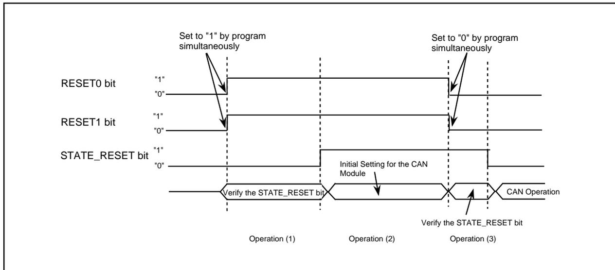
Figure 23.37 Example of CAN Module Reset Operation
