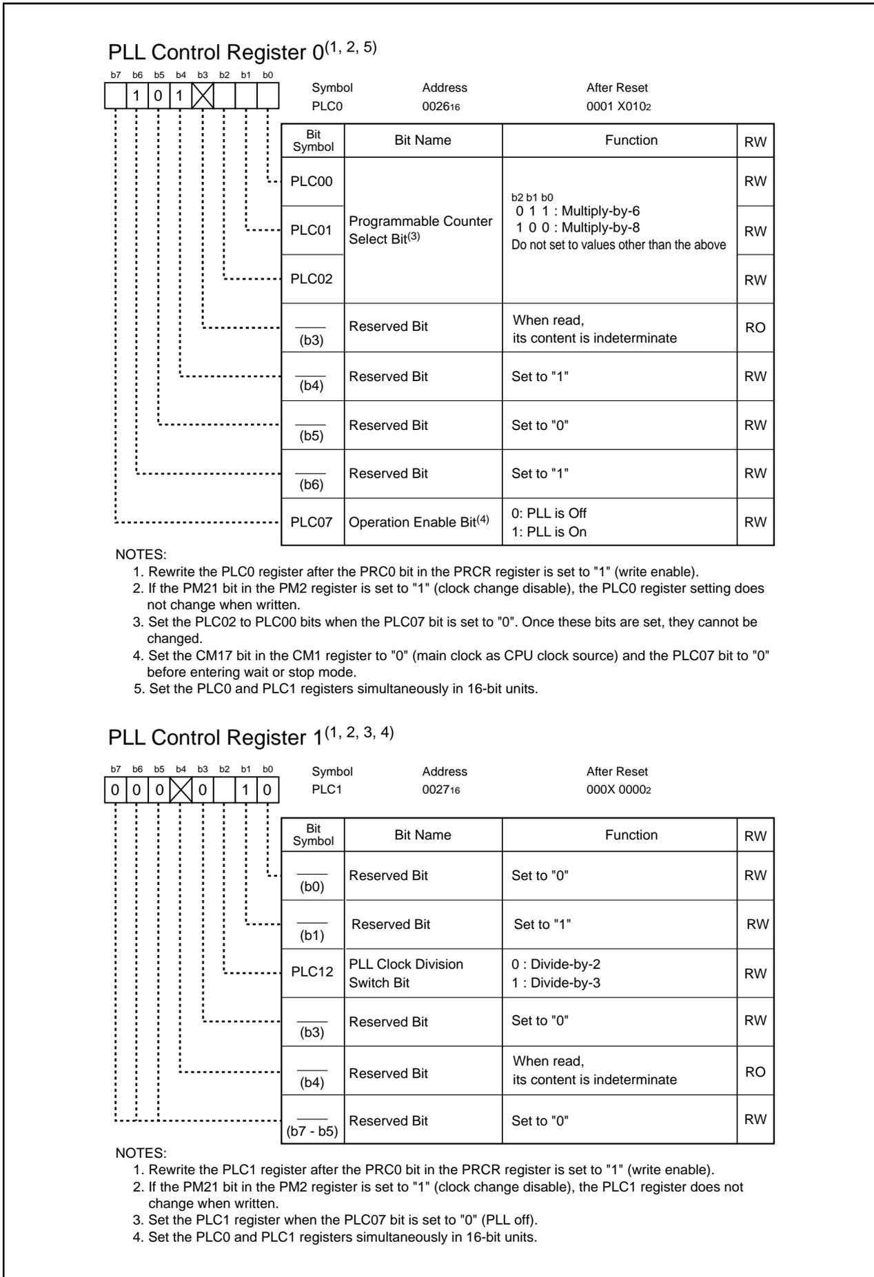
Figure 9.7 PLC0 and PLC1 Registers
