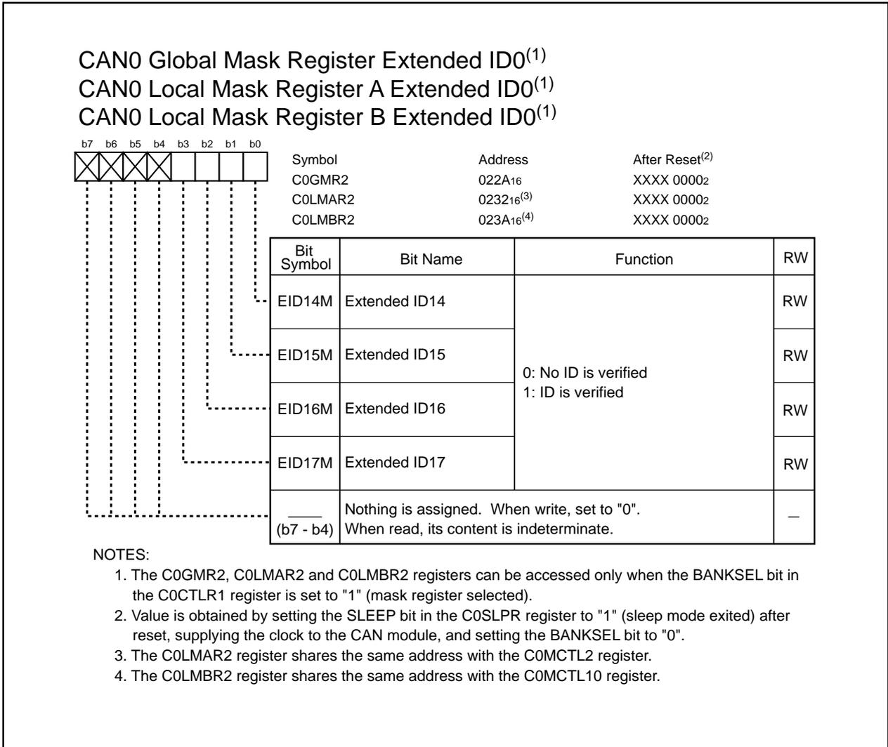
Figure 23.24 C0GMR2, C0LMAR2 and C0LMBR2 Registers
