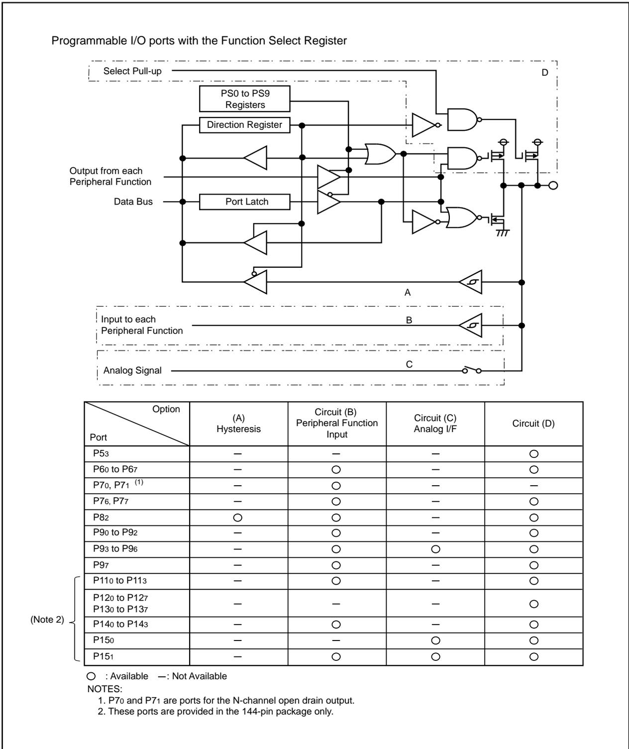
Figure 24.3 Programmable I/O Ports (3)
