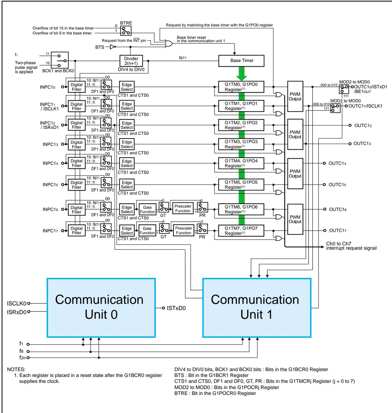
Figure 22.1 Intelligent I/O Block Diagram
