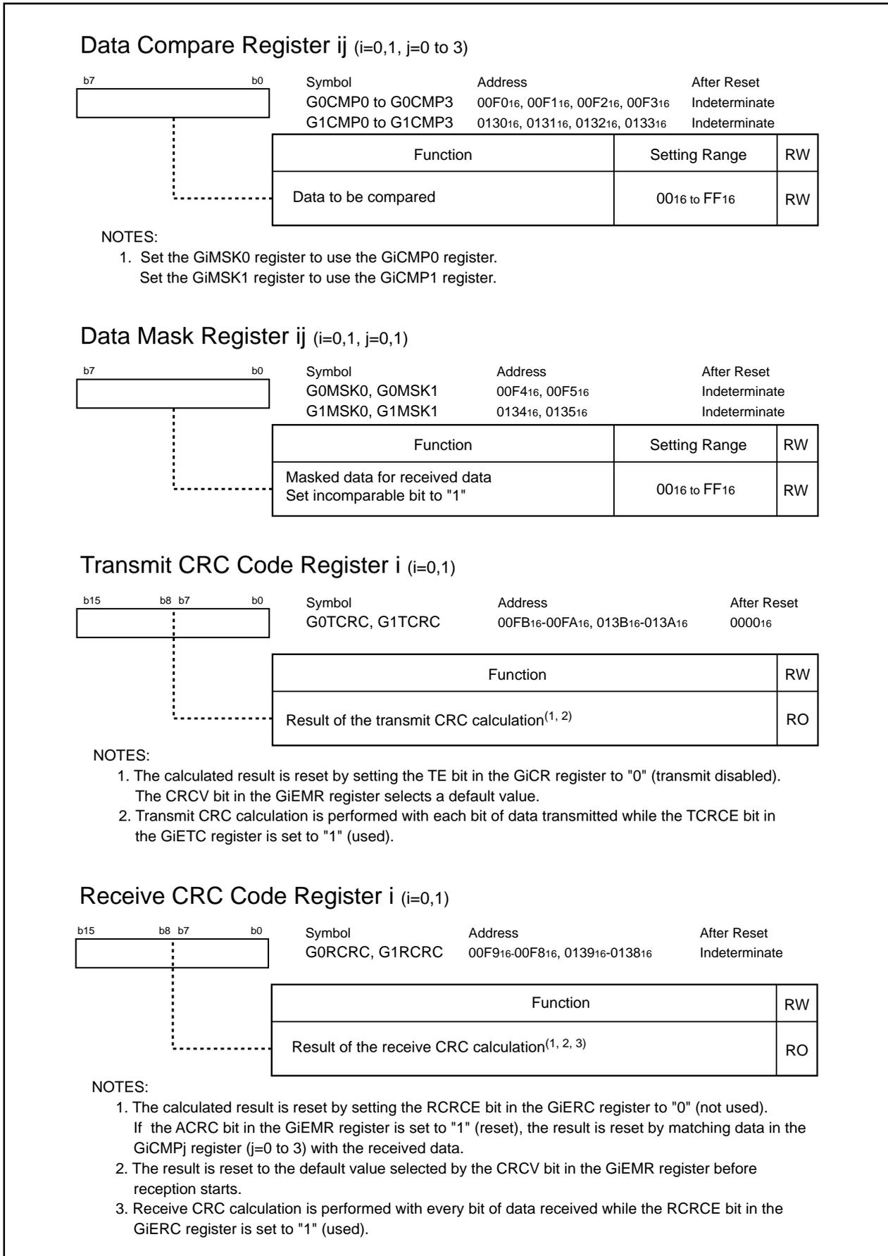
**Figure 22.28 G0CMP0 to G0CMP3 Registers and G1CMP0 to G1CMP3 Registers
