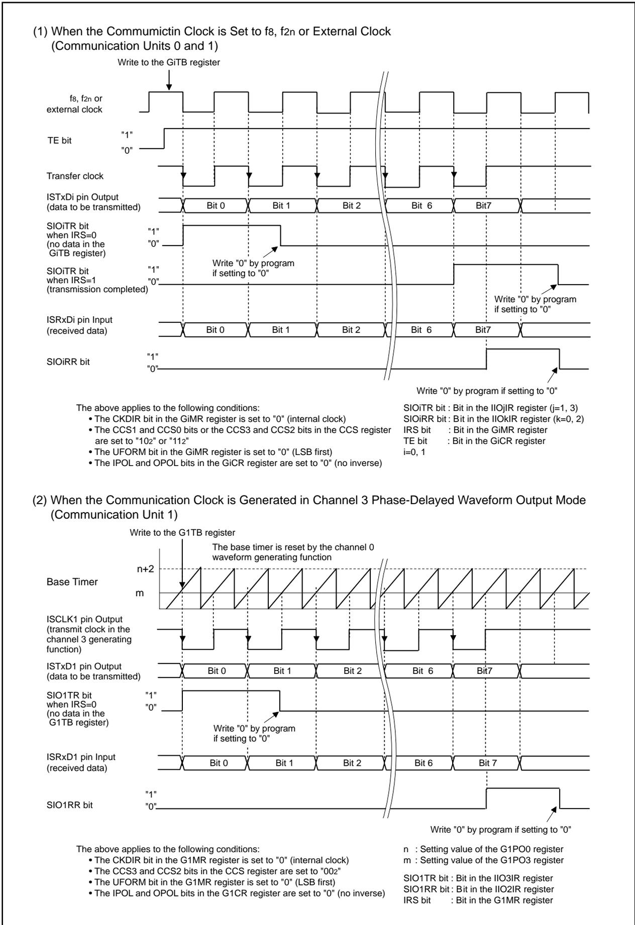
Figure 22.30 Transmit and Receive Operation
