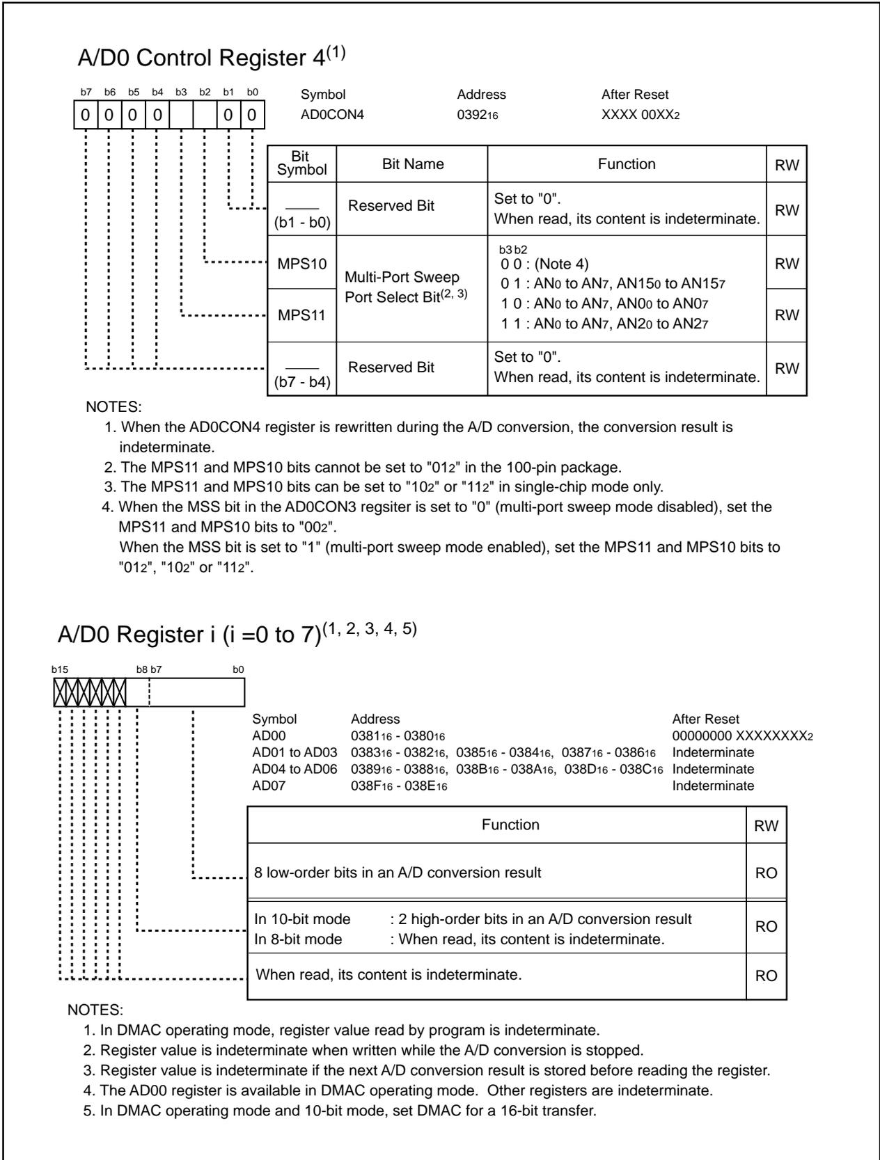
**Figure 18.6 AD0CON4 Register and AD00 to AD07 Registers**
