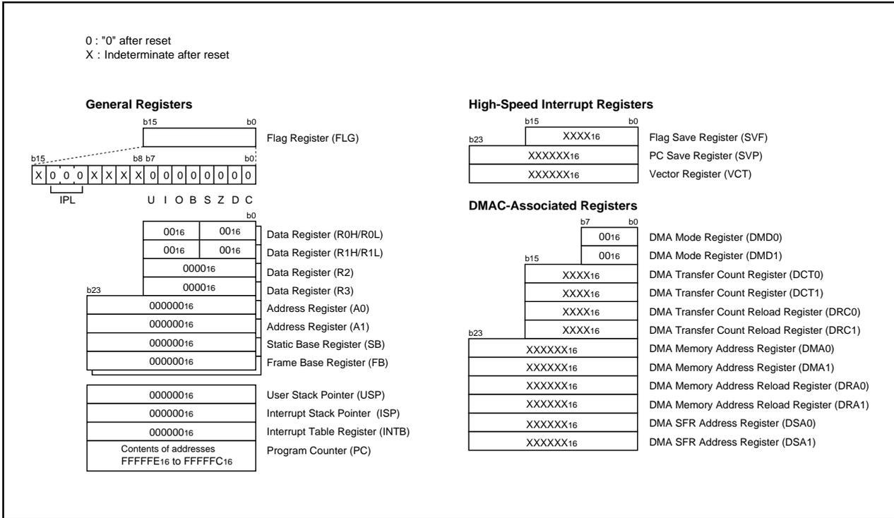
Figure 5.4 CPU Register States after Reset
