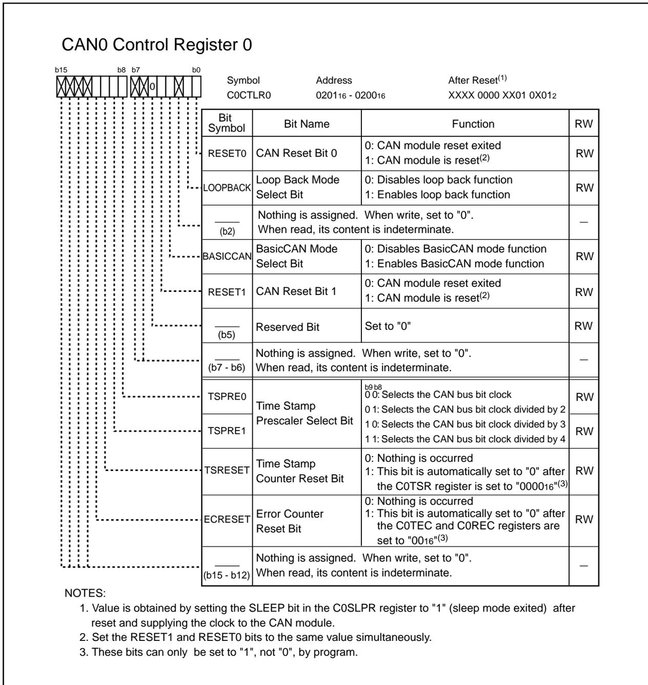
**Figure 23.3 C0CTRL0 and C1CTRL0 Registers**
