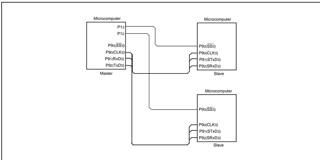
Figure 17.23 Serial Bus Communication Control with SS Pin
