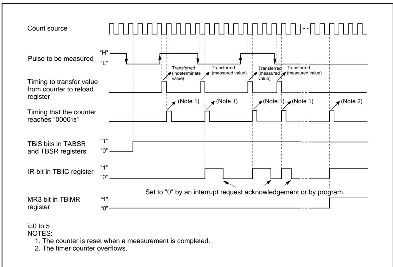
Figure 15.24 Operation Example in Pulse Width Measurement Mode
