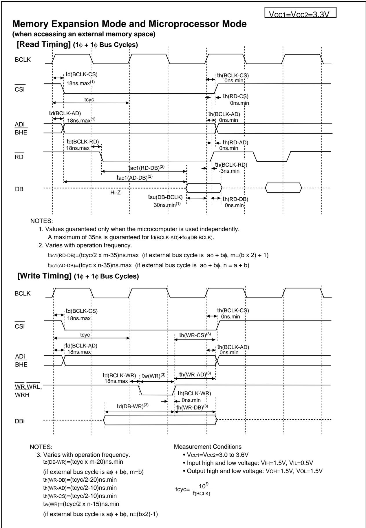
**Figure 26.7 V<sub>CC1</sub>=V<sub>CC2</sub>=3.3V Timing Diagram (1)**
