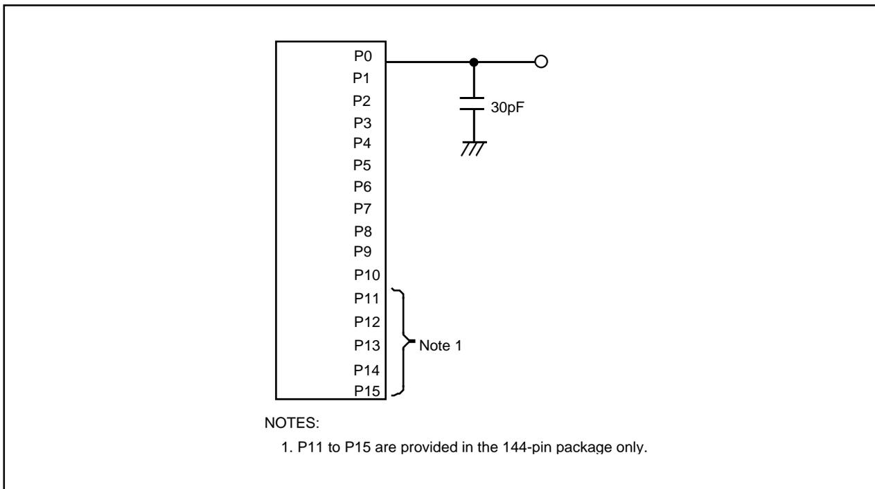
**Figure 26.12 P0 to P15 Measurement Circuit**
