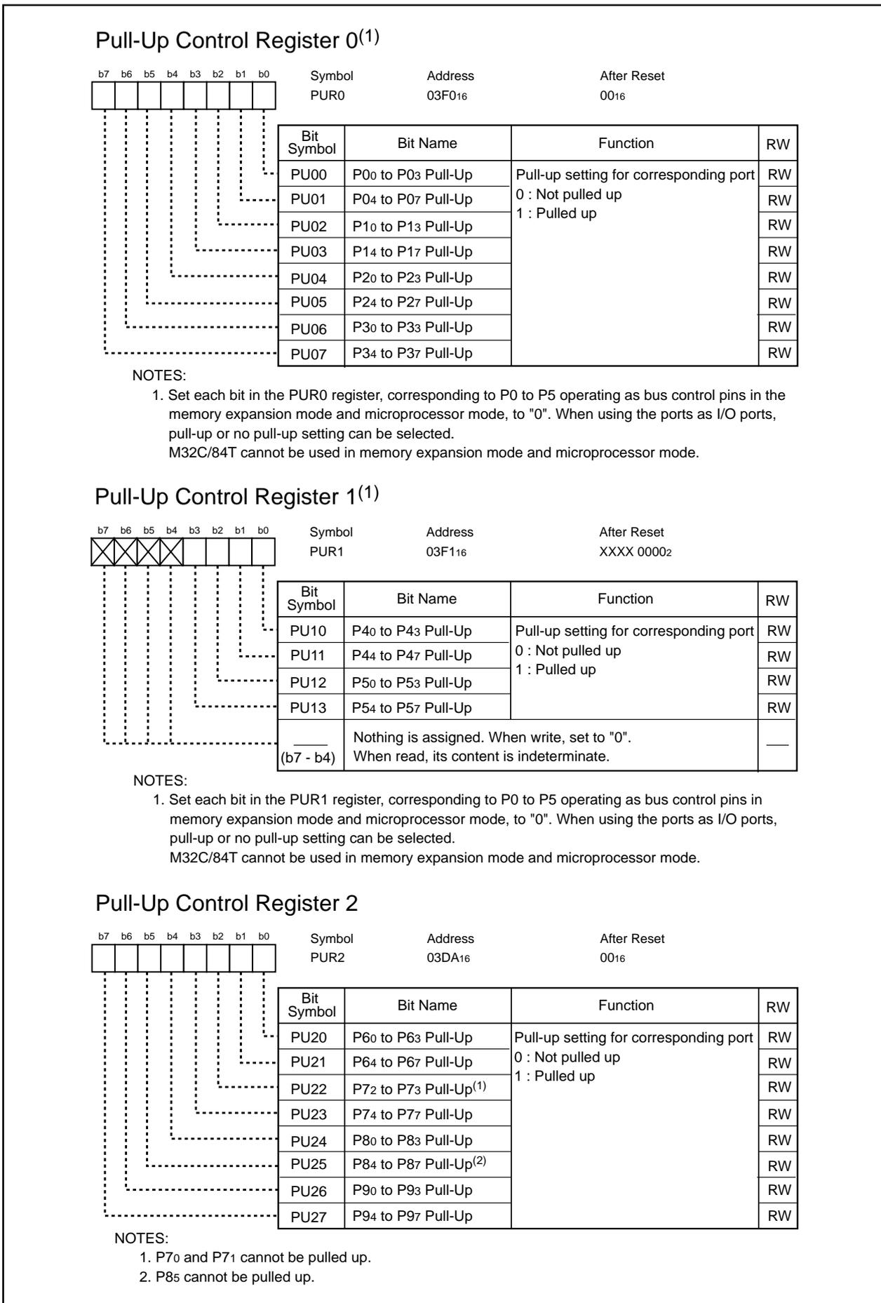
**Figure 24.15 PUR0 Register, PUR1 Register and PUR2 Register**
