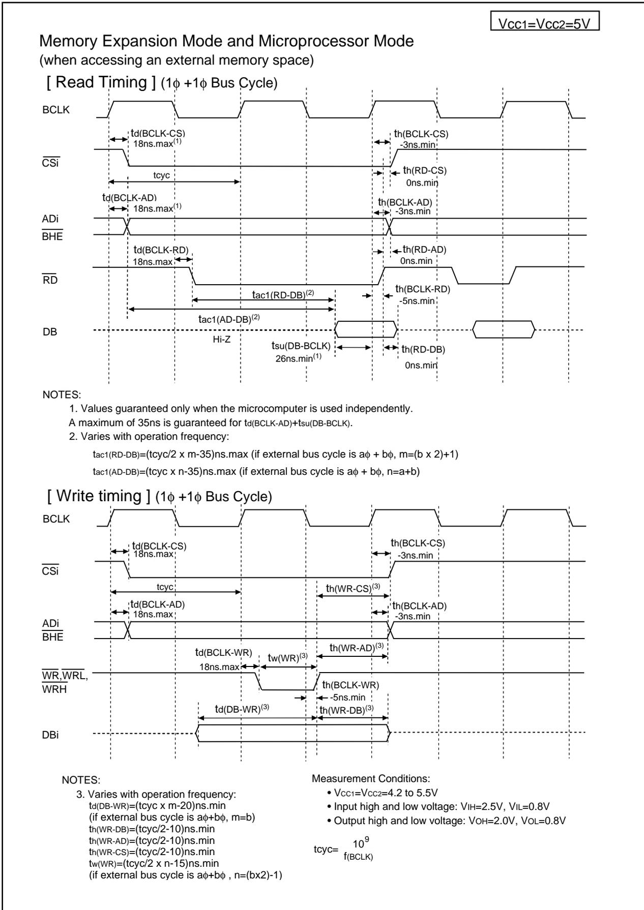
Figure 26.3 V<sub>CC1</sub>=V<sub>CC2</sub>=5V Timing Diagram (1)
