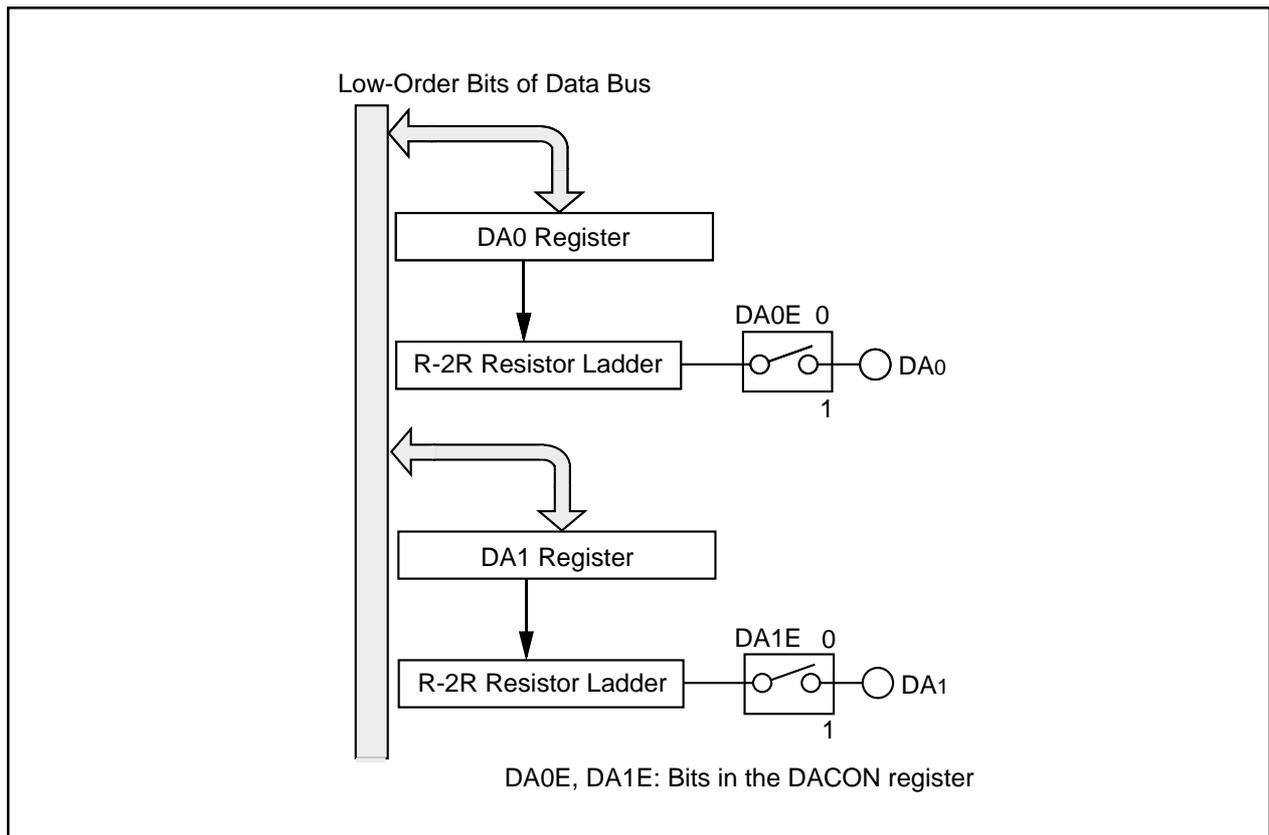
**Figure 19.1 D/A Converter**
