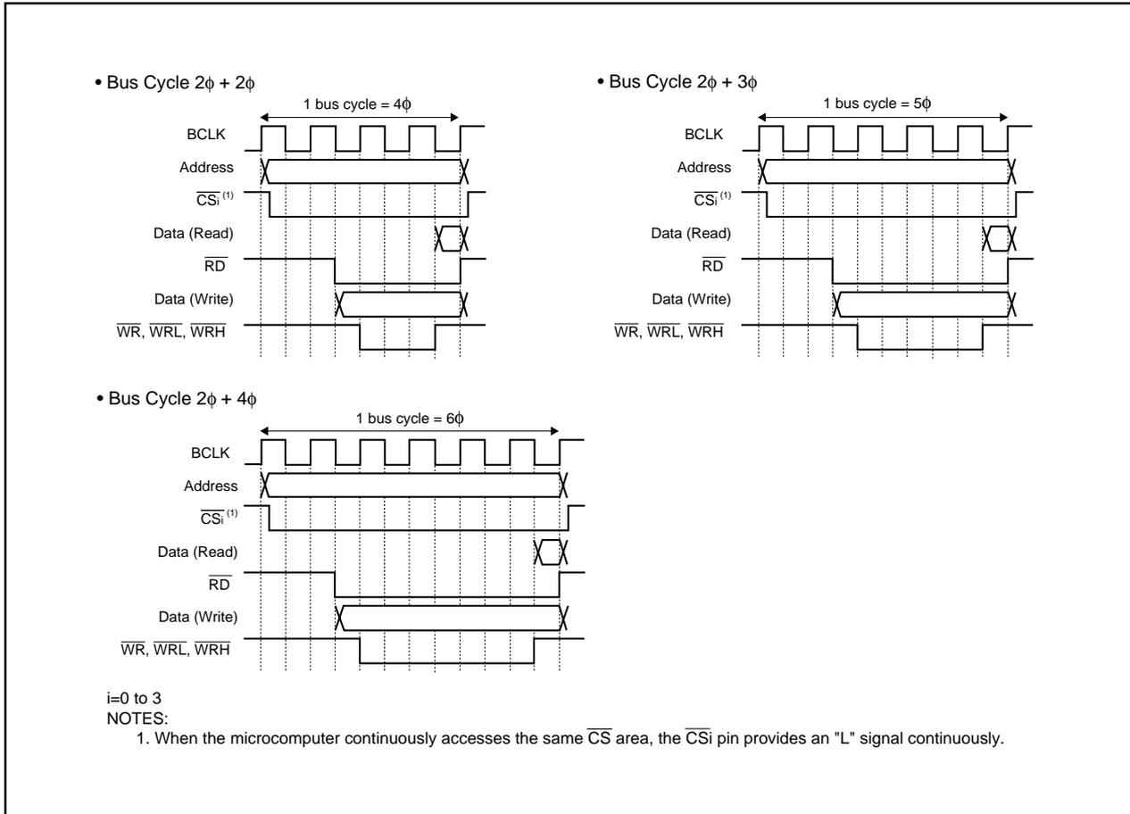
Figure 8.5 Bus Cycle with Separate Bus (2)
