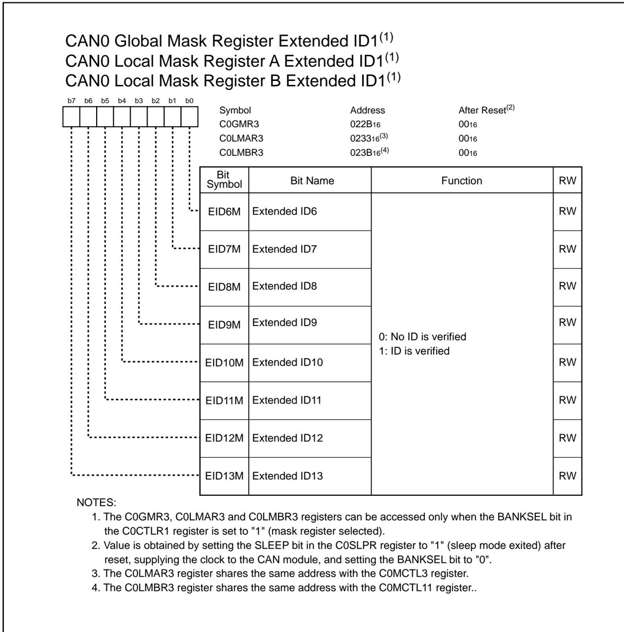
**Figure 23.25 C0GMR3, C0LMAR3 and C0LMBR3 Registers**
