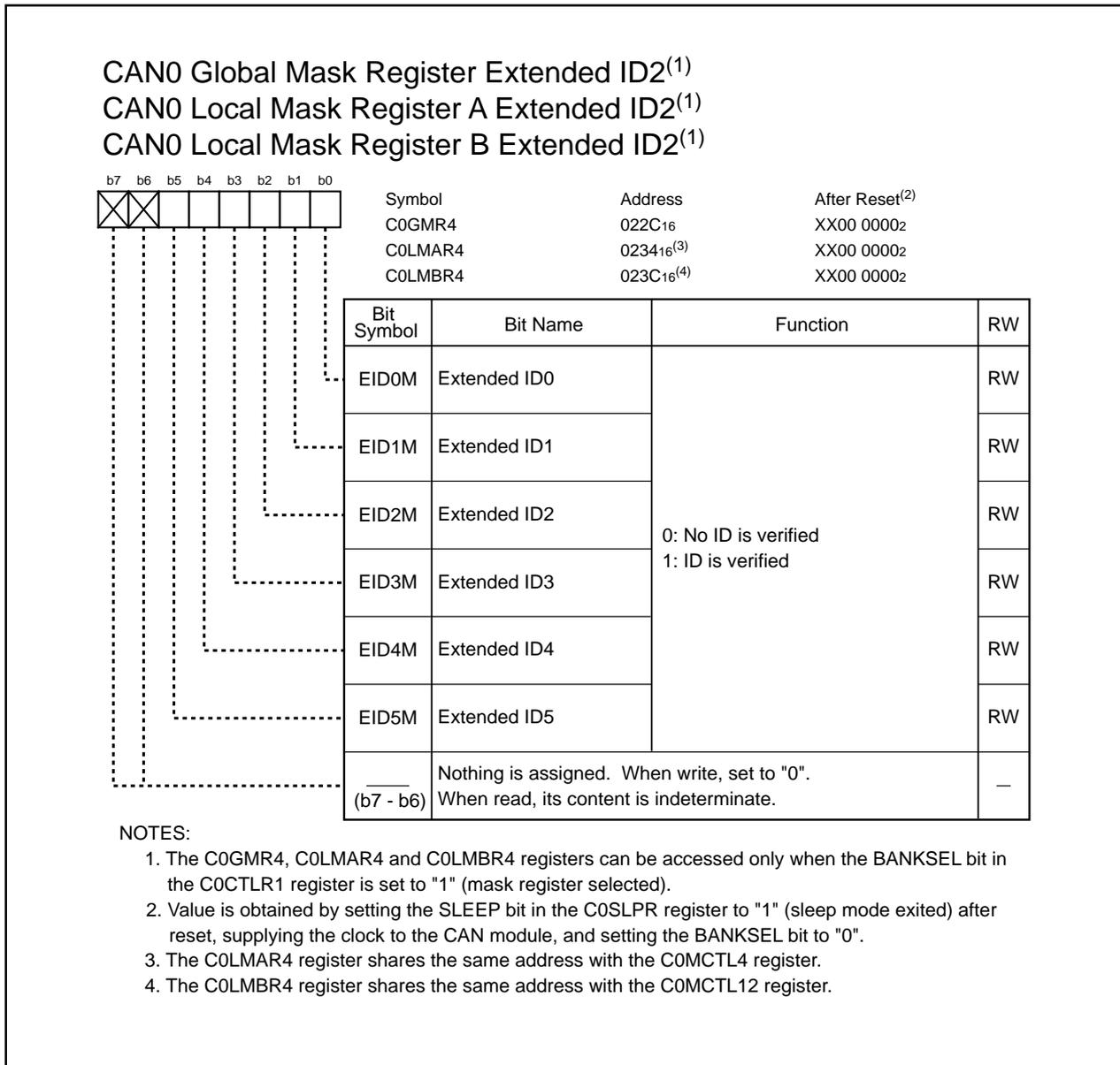
**Figure 23.26 C0GMR4, C0LMAR4 and C0LMBR4 Registers**
