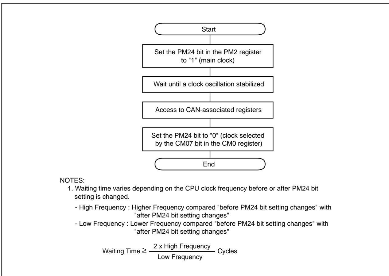
**Figure 23.36 Accessing Procedure for CAN-Associated Registers**
