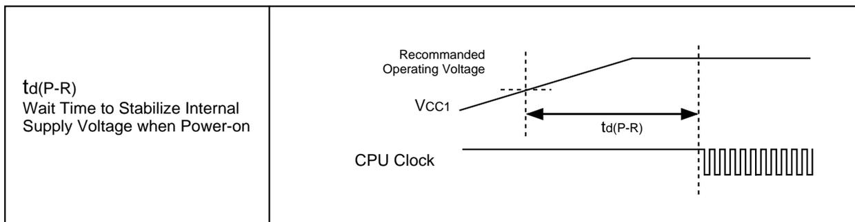
**Figure 26.11 Power Supply Timing Diagram**
