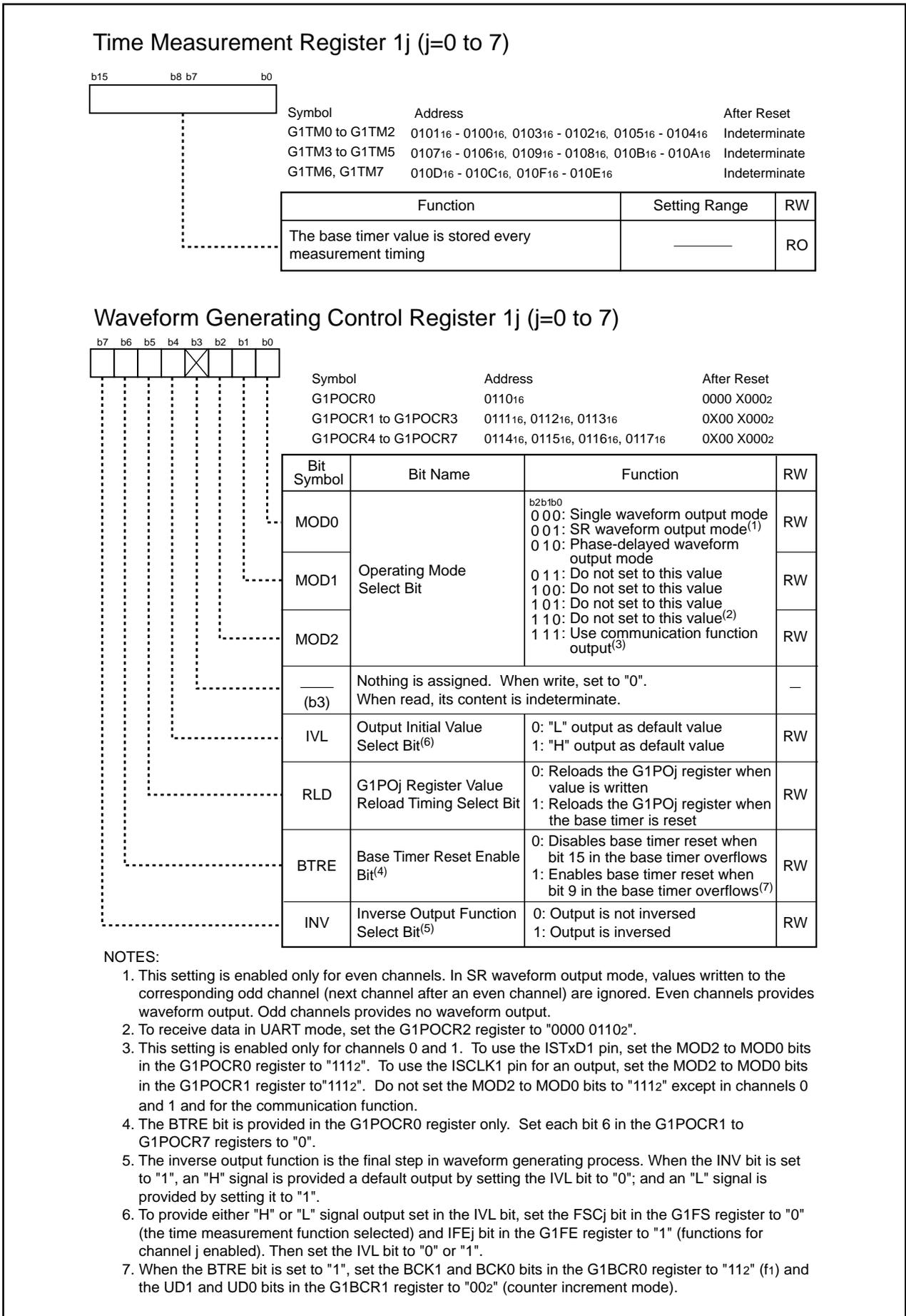
**Figure 22.6 G1TM0 to G1TM7 Registers and G1POCR0 to G1POCR7 Registers**
