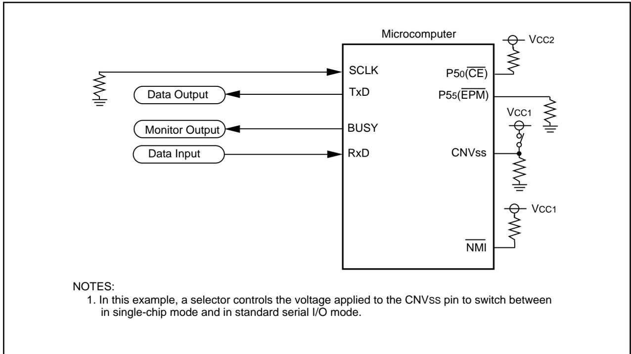
Figure 25.18 Circuit Application in Standard Serial I/O Mode 2
