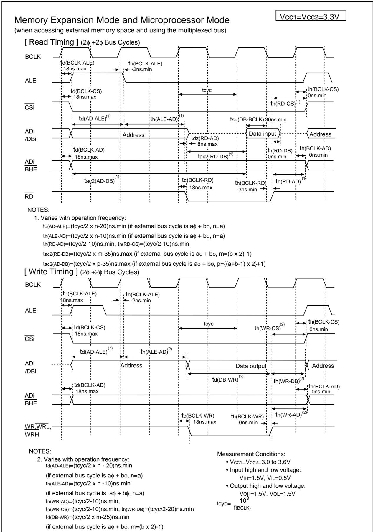
**Figure 26.8 V<sub>CC1</sub>=V<sub>CC2</sub>=3.3V Timing Diagram (2)**
