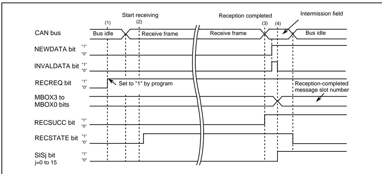
Figure 23.39 Example of CAN Data Frame Receive Operation
