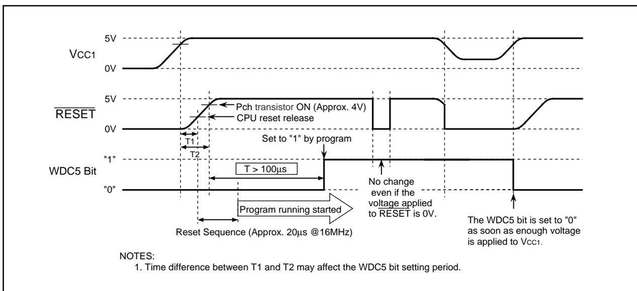
Figure 6.8 Cold Start-up/Warm Start-up Determine Function Operation
