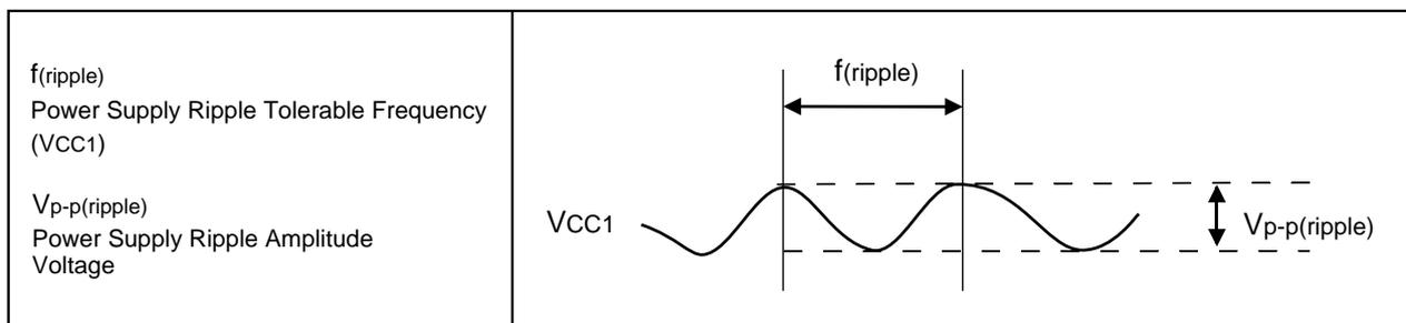
**Figure 27.2 Power Supply Fluctuation Timing**
