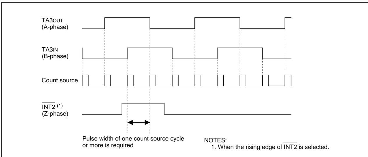
Figure 15.10 Two-Phase Pulse (A-phase and B-phase) and Z-phase
