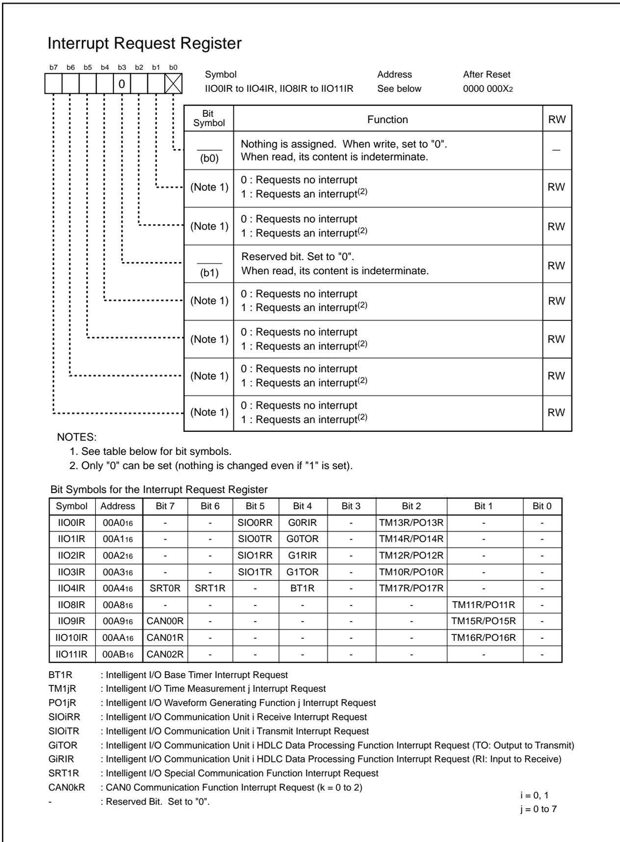
Figure 11.14 IIO0IR to IIO4IR, IIO8IR to IIO11IR Registers
