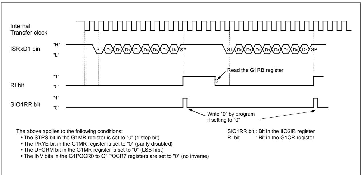
**Figure 22.32 Receive Operation**
