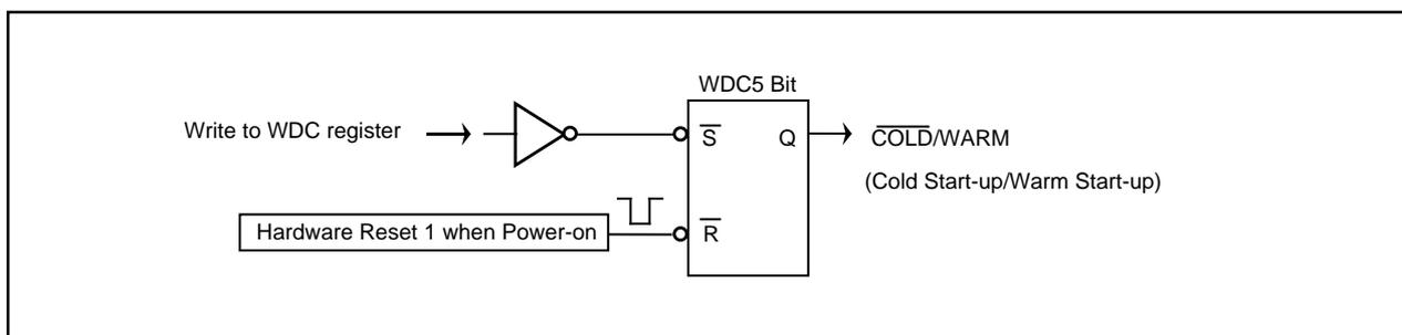
Figure 6.7 Cold Start-up/Warm Start-up Determine Function Block Diagram
