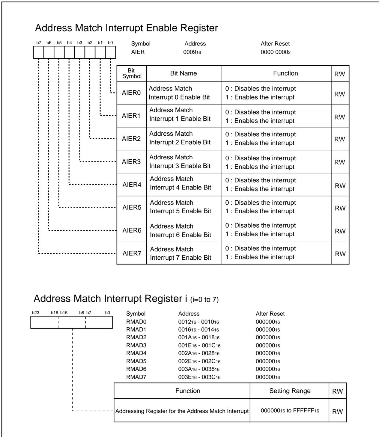
Figure 11.12 AIER Register and RMAD0 to RMAD7 Registers
