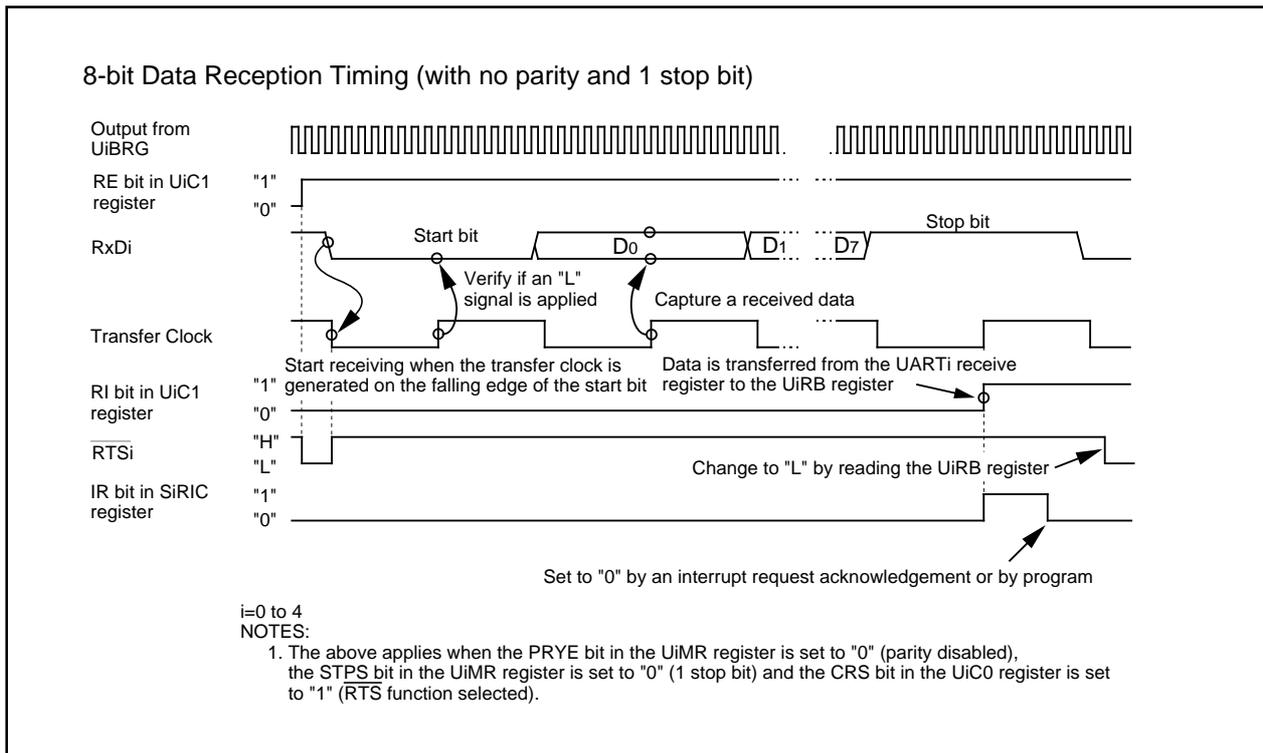
Figure 17.15 Receive Operation
