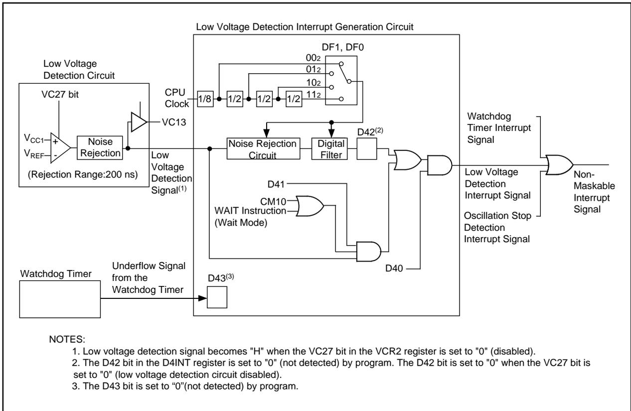
Figure 6.5 Low Voltage Detection Interrupt Generation Circuit
