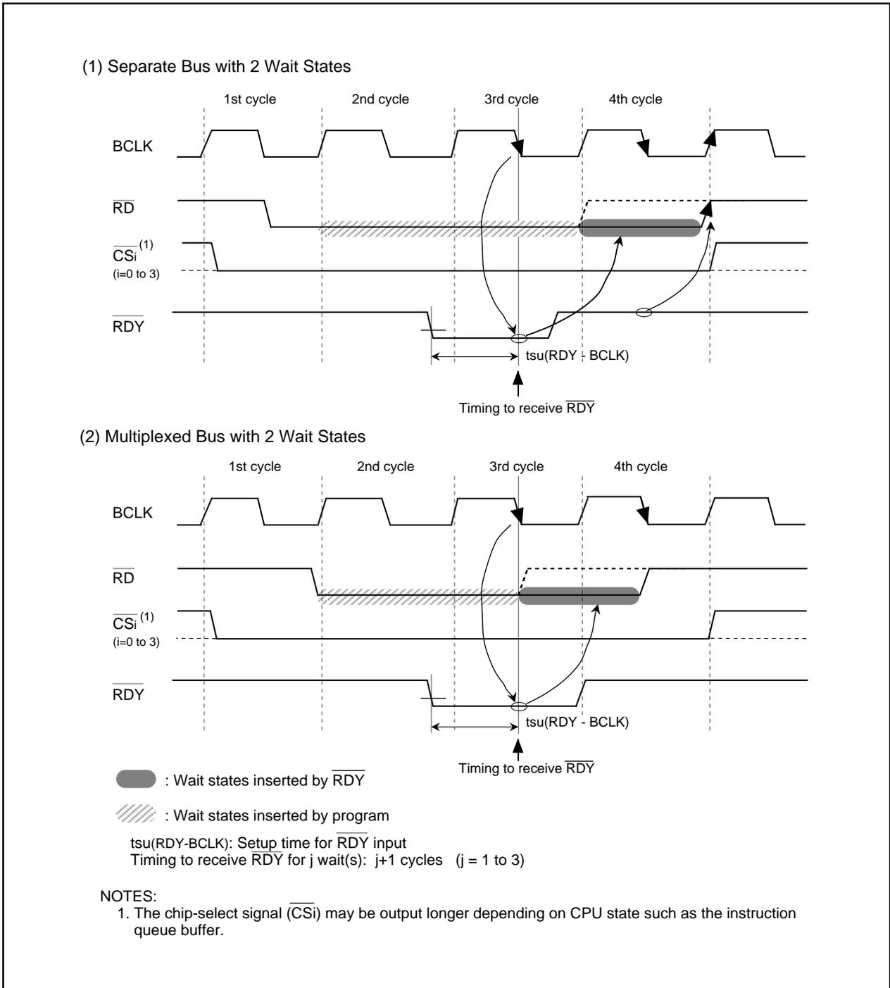
Figure 8.11  $\overline{RD}$  Signal Output Extended by  $\overline{RDY}$  Signal
