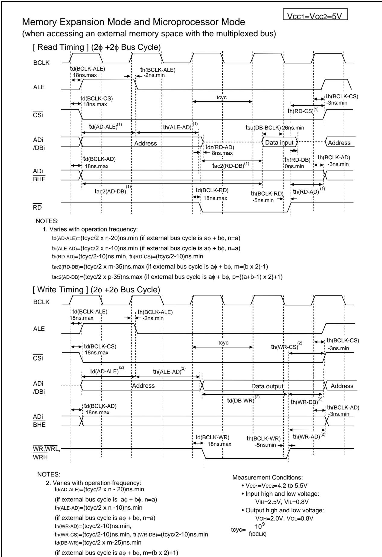
**Figure 26.4 V<sub>CC1</sub>=V<sub>CC2</sub>=5V Timing Diagram (2)**
