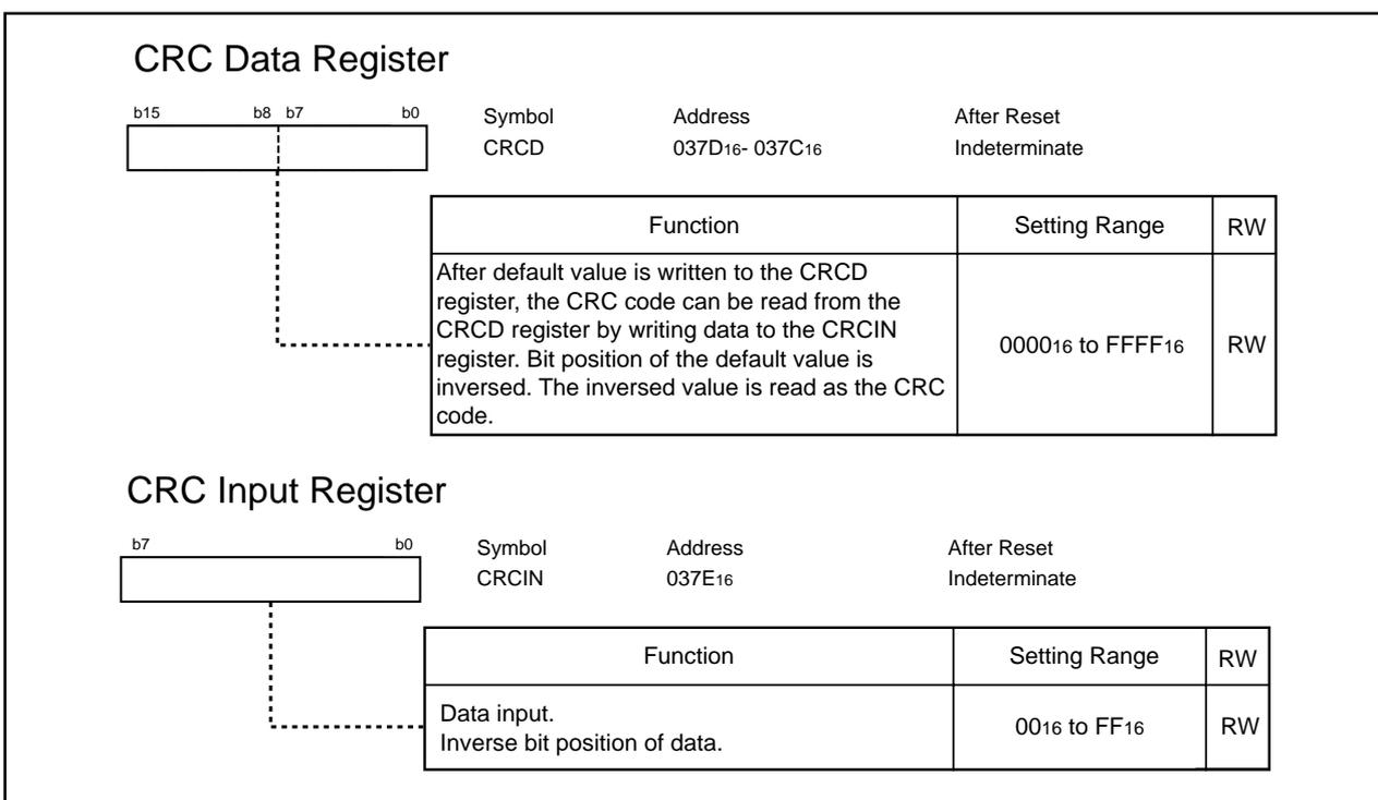
Figure 20.2 CRCD Register and CRCIN Register
