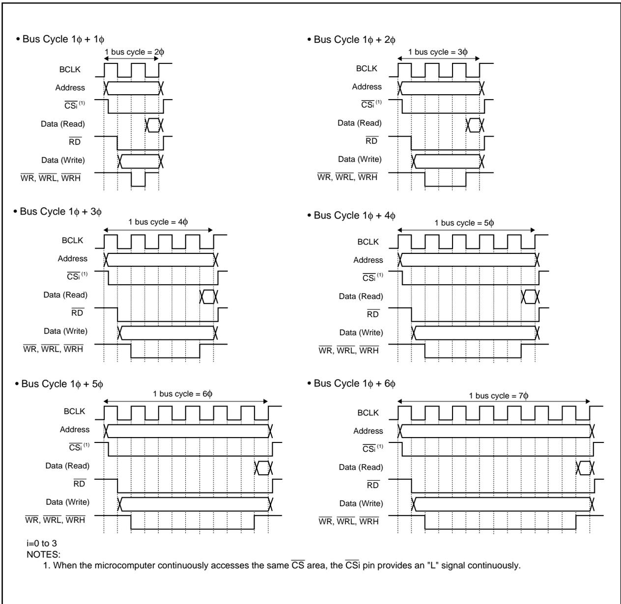
Figure 8.4 Bus Cycle with Separate Bus (1)
