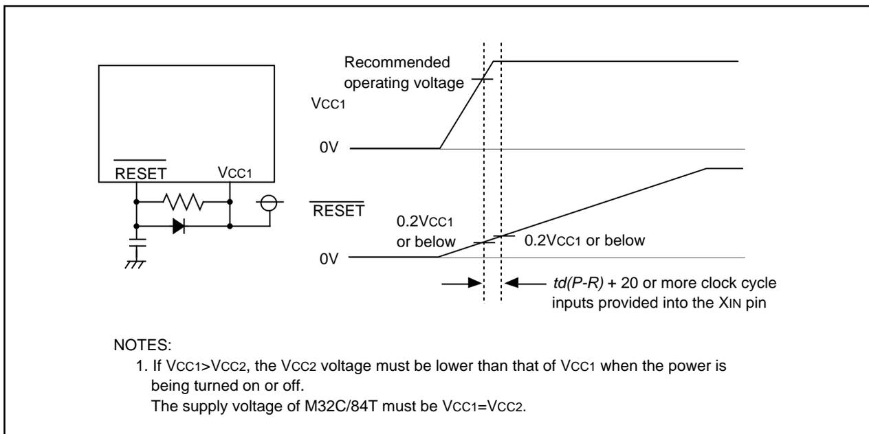
**Figure 5.1** Reset Circuit
