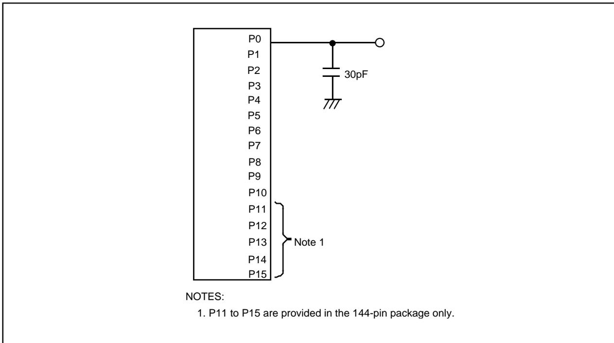
**Figure 26.2 P0 to P15 Measurement Circuit**
