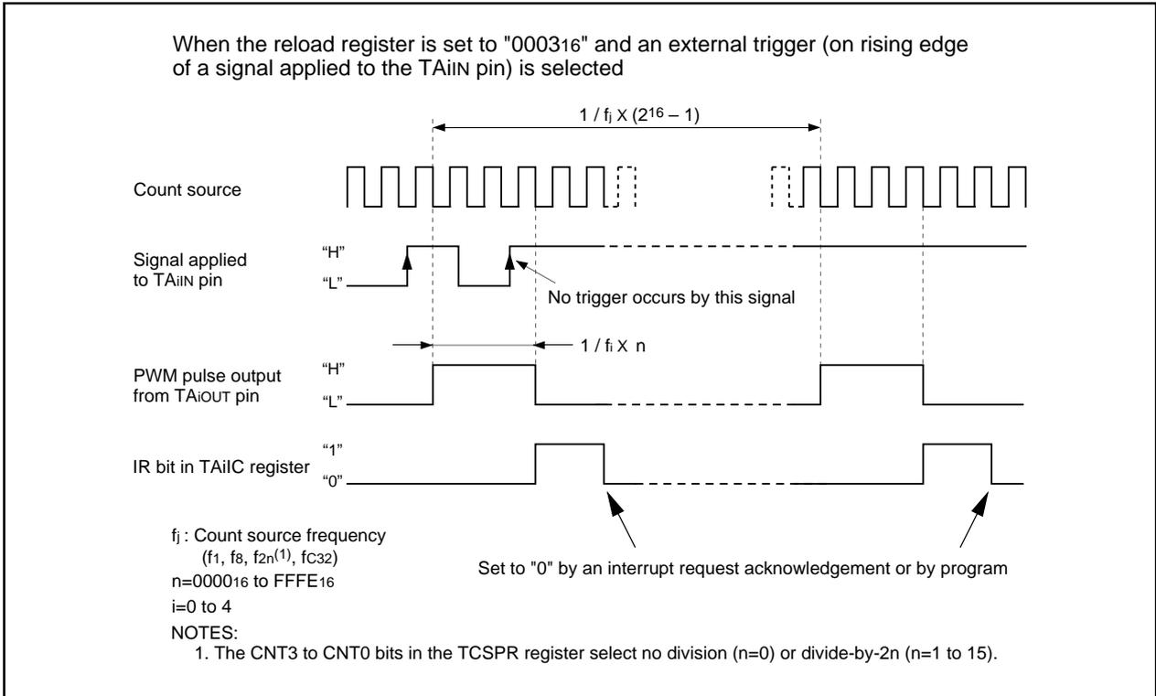
Figure 15.14 16-bit Pulse Width Modulator Operation
