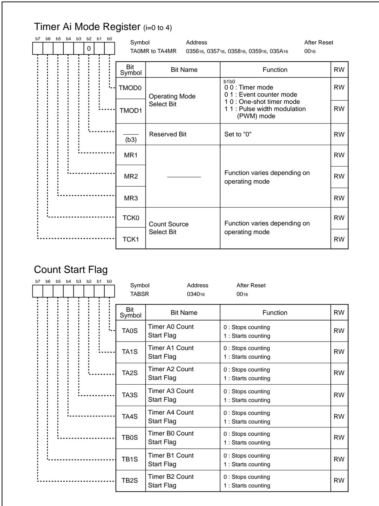
Figure 15.5 TA0MR to TA4MR Registers and TABSR Register
