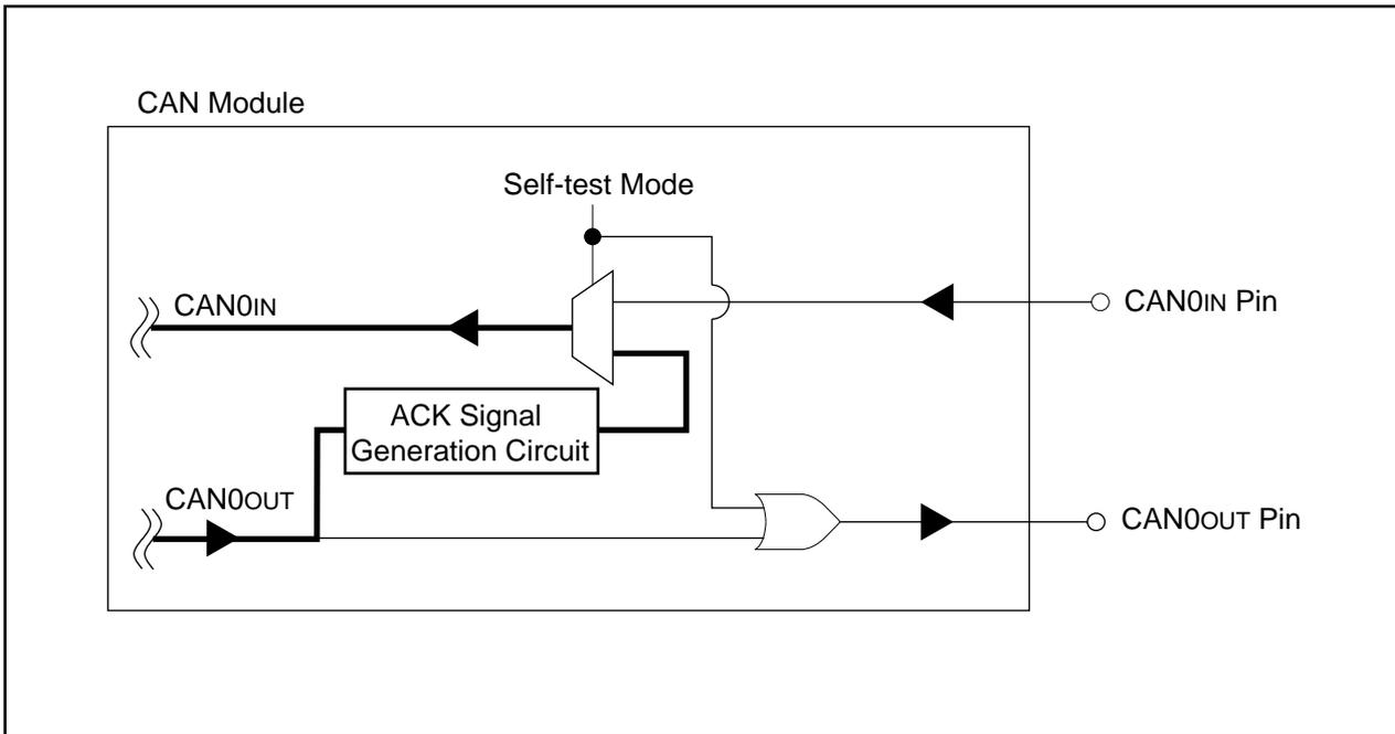
**Figure 23.19 Self-Test Mode**
