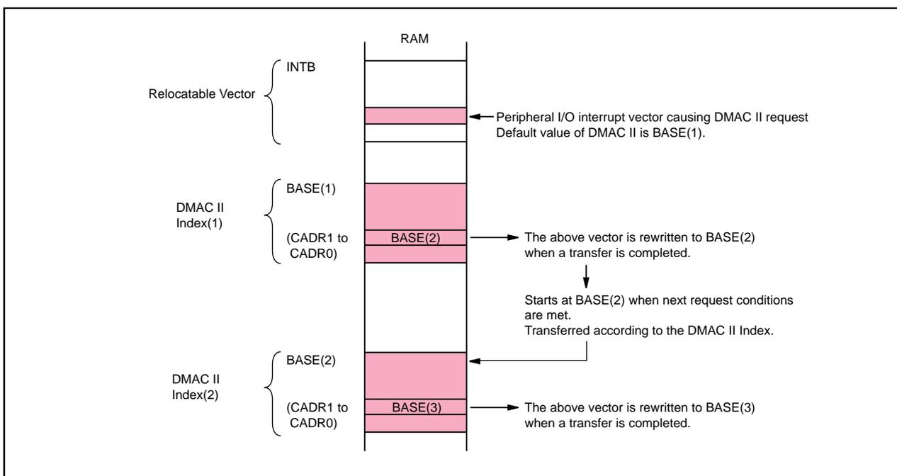
Figure 14.4 Relocatable Vector and DMAC II Index
