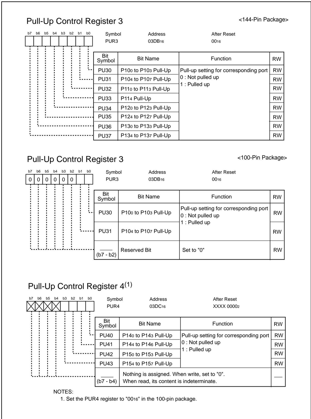
**Figure 24.16 PUR3 Register and PUR4 Register**
