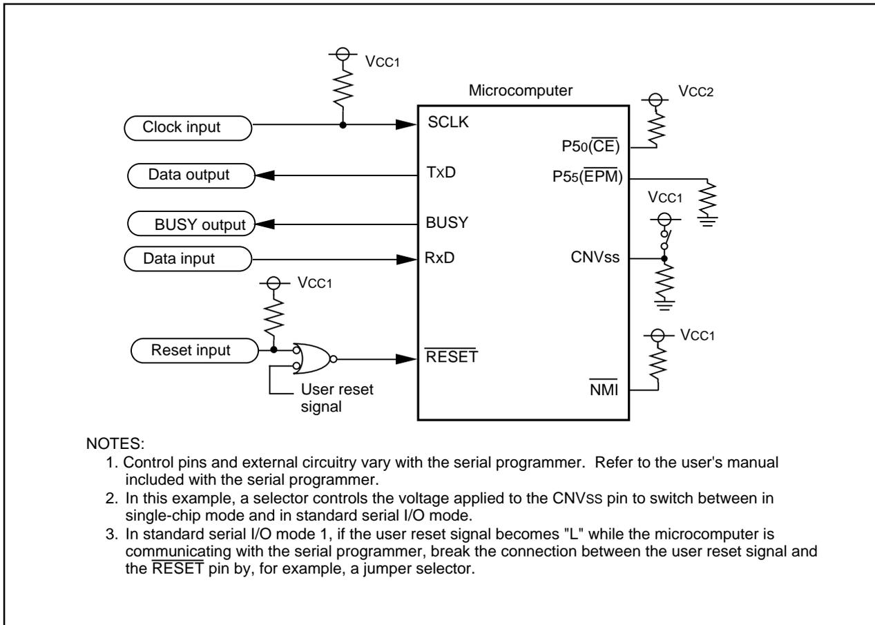
**Figure 25.17 Circuit Application in Standard Serial I/O Mode 1**
