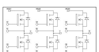
$$\begin{split} V_{DSS} &= 500 V \\ R_{DSon} &= 65 m \Omega \text{ typ @ Tj} = 25^{\circ} C \\ I_D &= 51 A \text{ @ Tc} = 25^{\circ} C \end{split}$$
