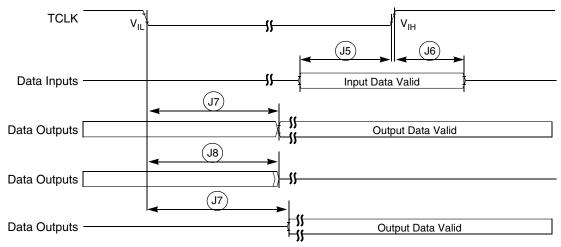
Figure 11. Boundary Scan (JTAG) Timing
