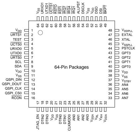
Figure 4. 64 LQFP and 64 QFN Pin Assignments
