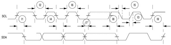
Figure 7. I<sup>2</sup>C Input/Output Timings
