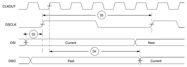
Figure 15. BDM Serial Port AC Timing
