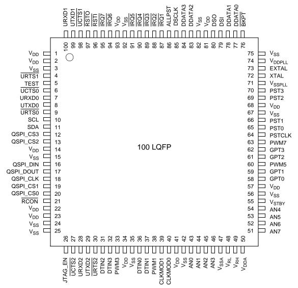
Figure 2. 100 LQFP Pin Assignments
