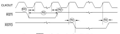
Figure 6. RSTI and Configuration Override Timing
