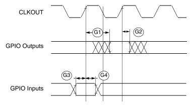
Figure 5. GPIO Timing
