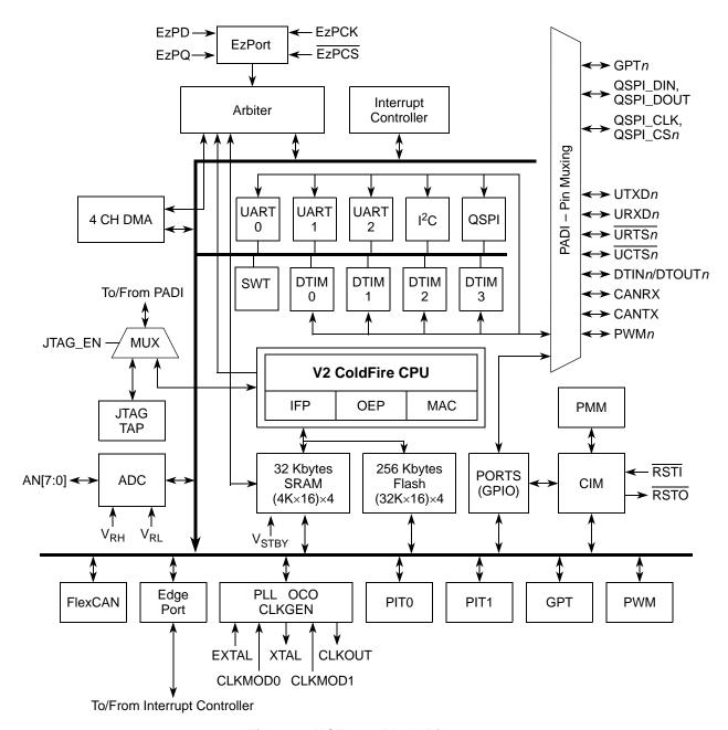
Figure 1. MCF5213 Block Diagram
