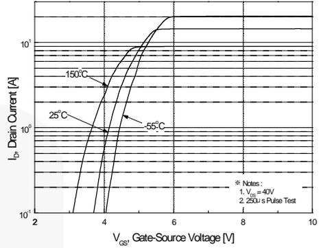
Figure 2. Transfer Characteristics
