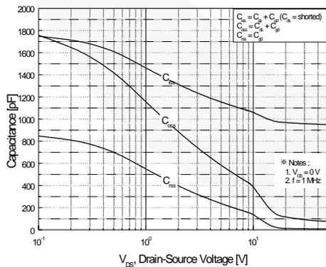
Figure 5. Capacitance Characteristics
