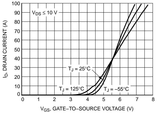
Figure 2. Transfer Characteristics
