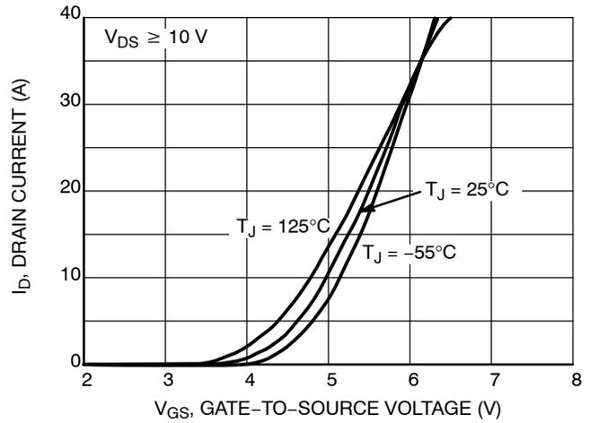
**Figure 2. Transfer Characteristics**
