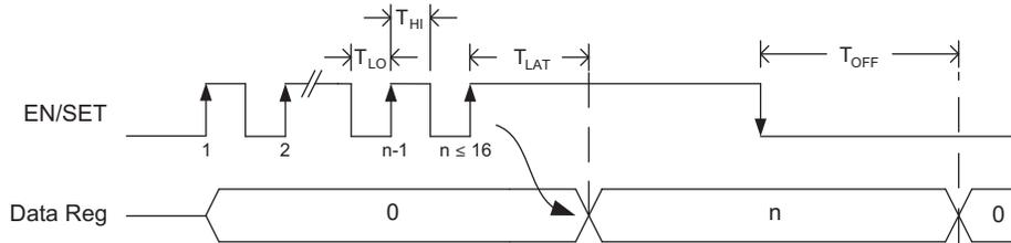
Figure 1: S<sup>2</sup>Cwire Serial Interface Timing.
