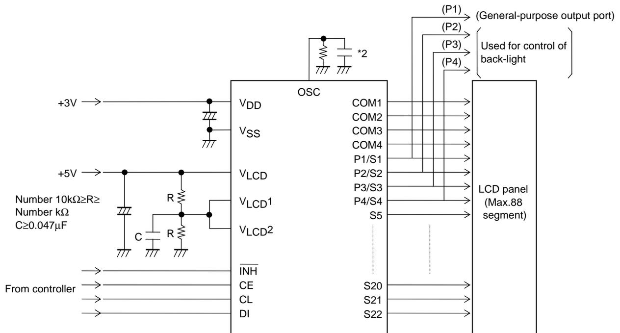
\*2 If a capacitor other than the external capacitor  $C_{osc}=680$  [pF] recommended is to be used, it is recommended to use a capacitor of 220 to 2200 [pF].
