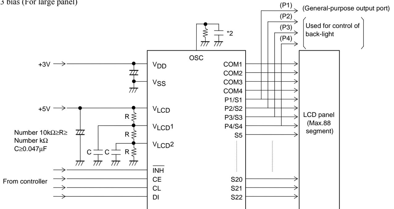
\*2 If a capacitor other than the external capacitor  $C_{osc}=680$  [pF] recommended is to be used, it is recommended to use a capacitor of 220 to 2200 [pF].
