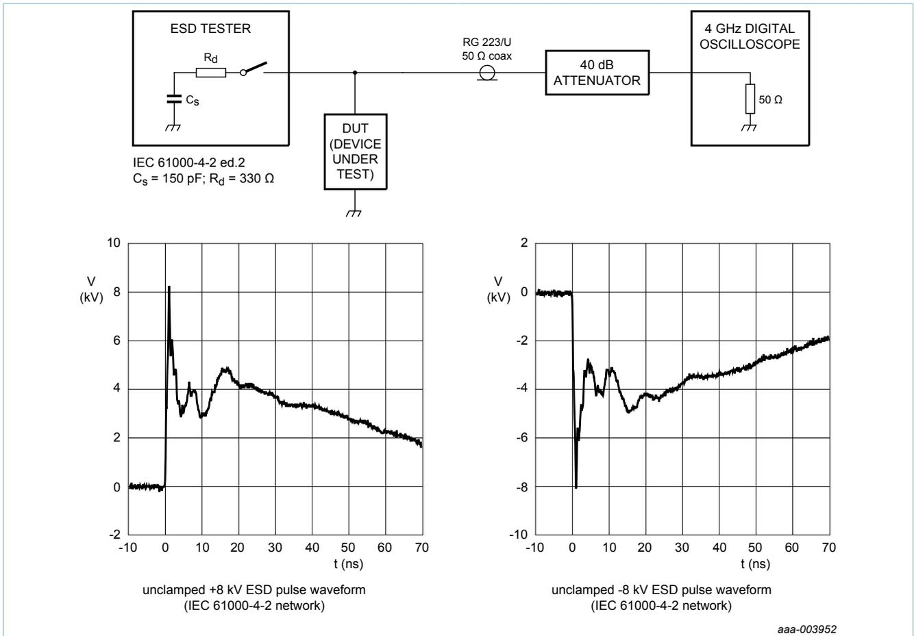
Fig. 3. ESD clamping test setup and waveforms
