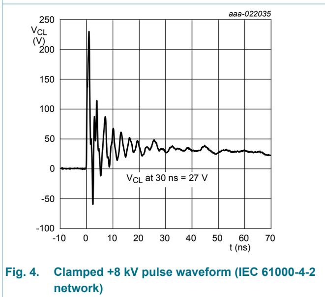
Fig. 4. Clamped +8 kV pulse waveform (IEC 61000-4-2 network)
