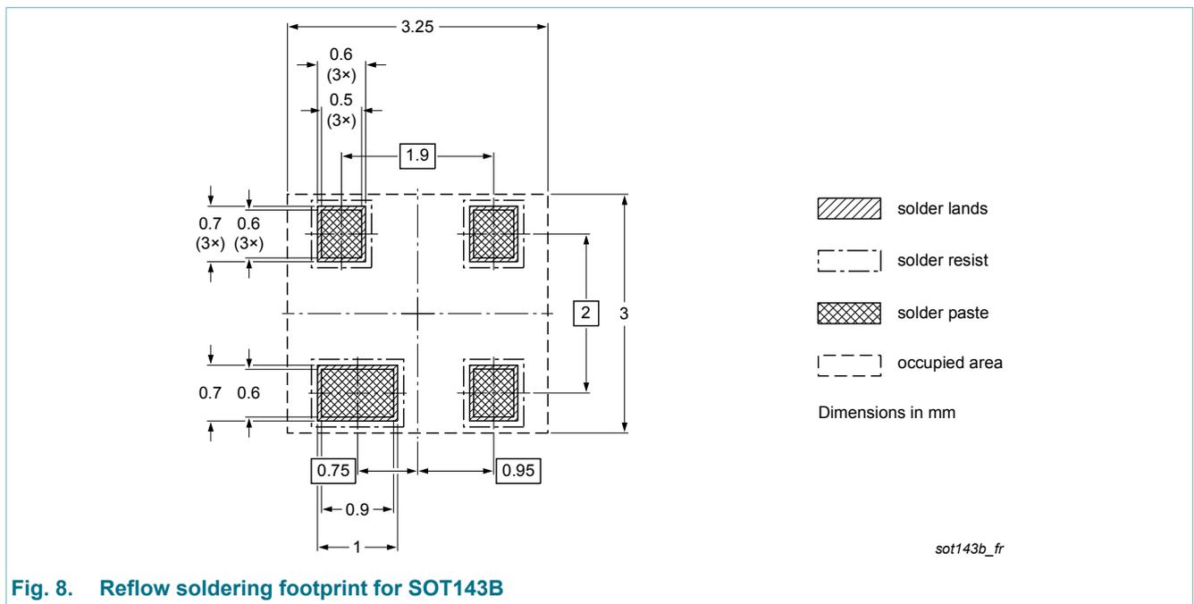
Fig. 8. Reflow soldering footprint for SOT143B
