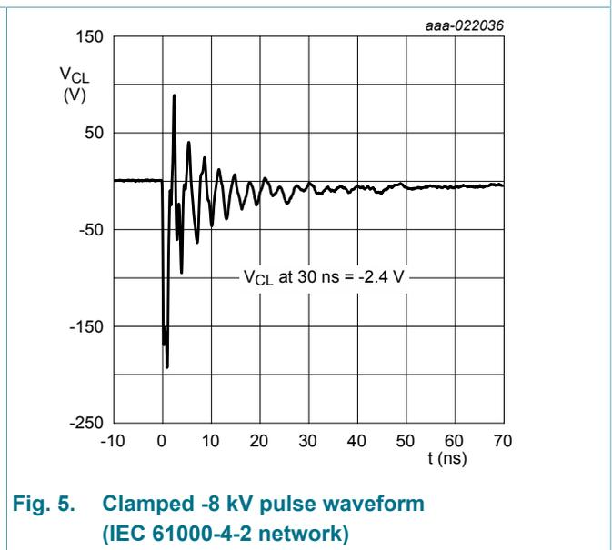
Fig. 5. Clamped -8 kV pulse waveform (IEC 61000-4-2 network)
