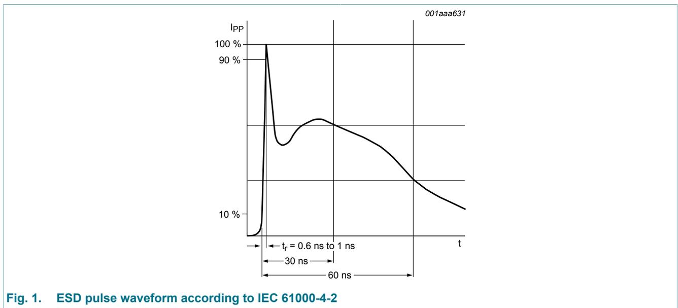
**Fig. 1. ESD pulse waveform according to IEC 61000-4-2**
